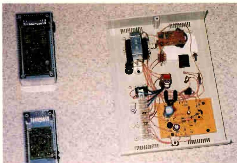
**Internal views of the assembled IR transmitter, IR receiver and control boxes.**
