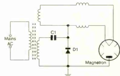
Fig. 1: The basic magnetron circuit.
