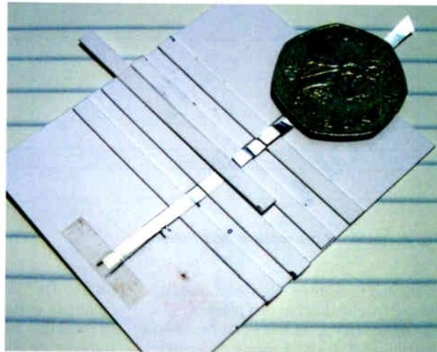
**Photo 6: Making the indentations in the replacement foil ribbon.**
