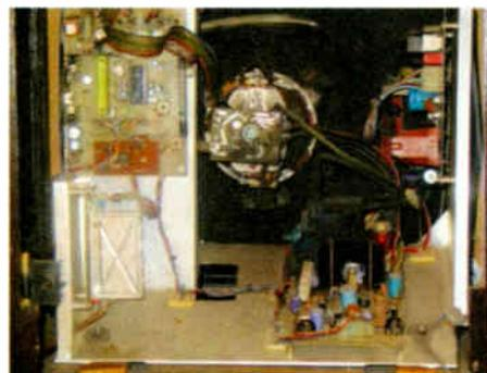
were originally next to the line output stage, are mounted vertically. This was done to avoid interference from the line output stage, the symptom being vertical striations. I also found it easier to carry out RGB grey-scale adjustments with the panel mounted vertically.
