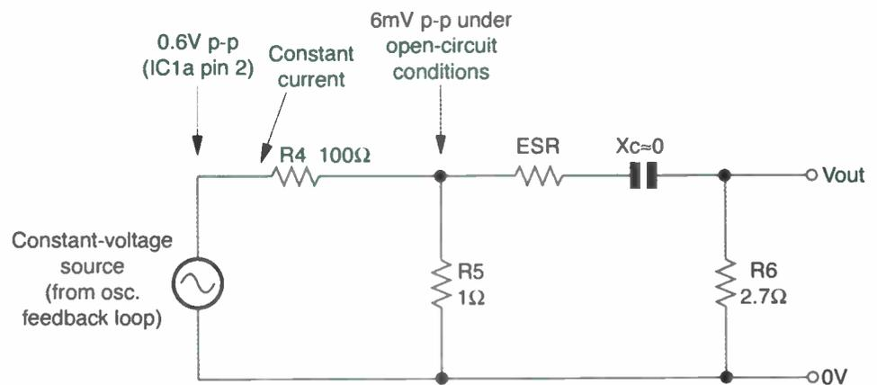
**Fig. 5: The method of test capacitor interface used in this meter. The source voltage is not a true constant voltage because of the need for R6, whose value must be comparable to the ESR of the capacitors in which we are interested.**
