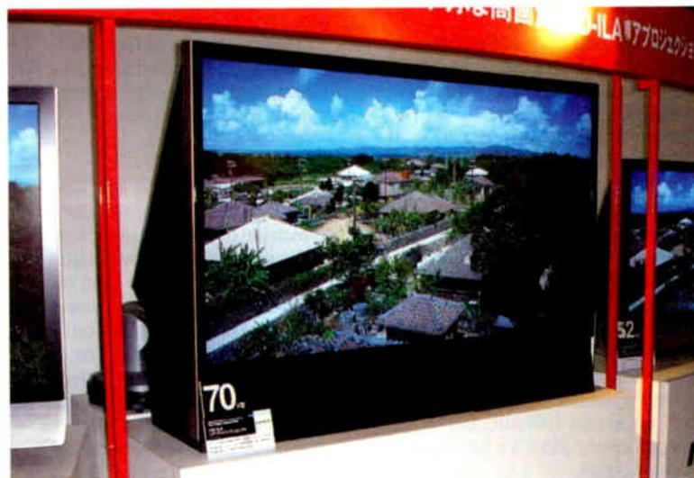
**JVC's giant 70in. rear-projection TV set which uses HD D-ILA (High Definition Digital Image Light Amplification) technology.**
