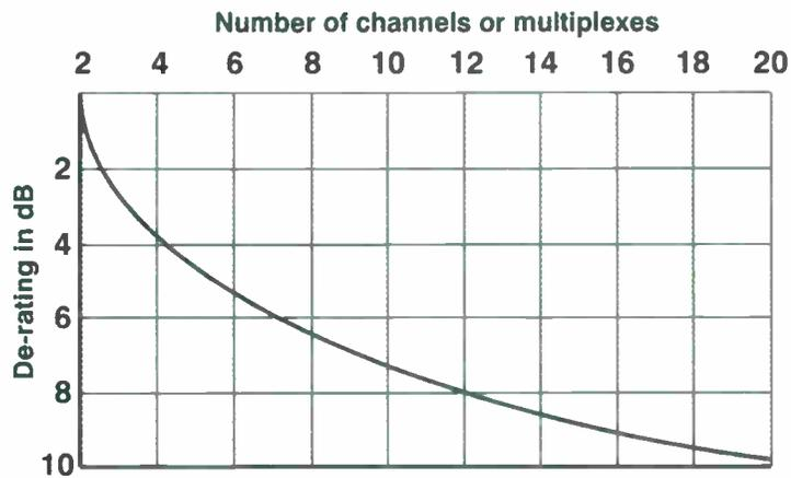
Fig. 19: Assuming that all channels are of the same strength, there is a simple relationship between the number of channels and an amplifier's maximum output.
