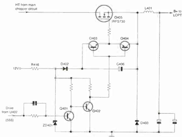
Fig. 1: The B+ chopper and driver circuitry used in the Compaq 151FS. Regulation relies on feedback from the line output transformer to pin 5 of the 555 timer chip.
