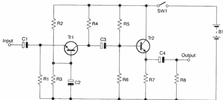
**Fig. 2: The preamplifier circuit.**
