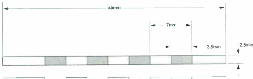
**Fig. 1: Details of the replacement ribbon.**
