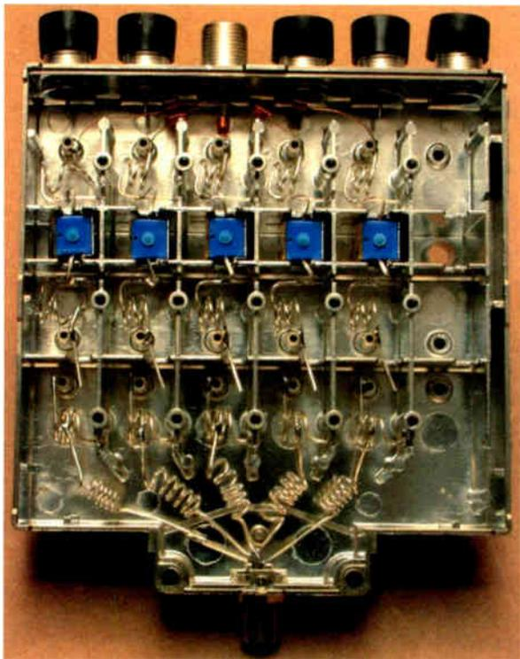
**Fig. 21: A five-channel filter unit with the rear cover removed. In this example all five channel paths share one input. From top to bottom, each path has a tuned stage, a variable attenuator (blue) then two more tuned stages.**
