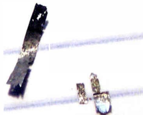
**Photo 4: The remains of the original ribbon element.**
