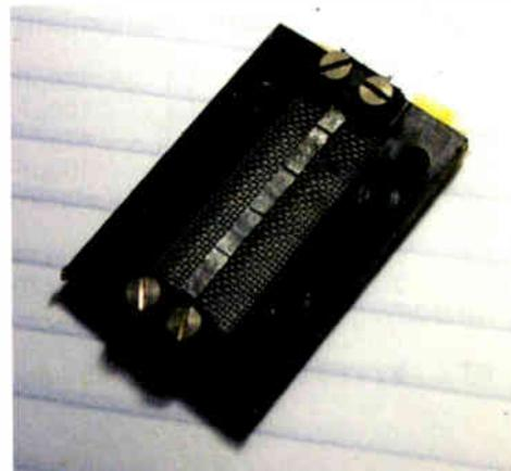
**Photo 3: The ribbon had been affected by corrosion, which had created two holes.**
