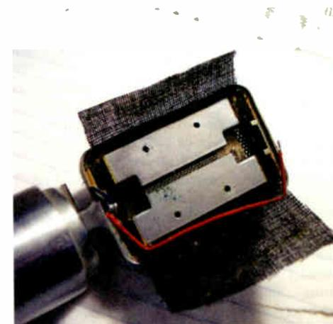
**Photo 5: The pole-pieces, with some corrosion still present.**
