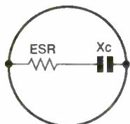
**Fig. 1: Simplified equivalent circuit of an electrolytic capacitor.  $X_c$  represents an ideal capacitor. Its reactance moves towards zero ohms as the frequency increases.  $X_c = 1/(2\pi fc)$ . The value of the equivalent series resistance ESR is determined mainly by the condition of the electrolyte.**
