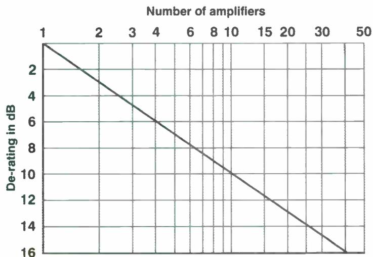
Fig. 20: If you connect four amplifiers in cascade, they must all be derated by 6dB. This is why the end-to-end amplification in a system should always be kept to a minimum.
