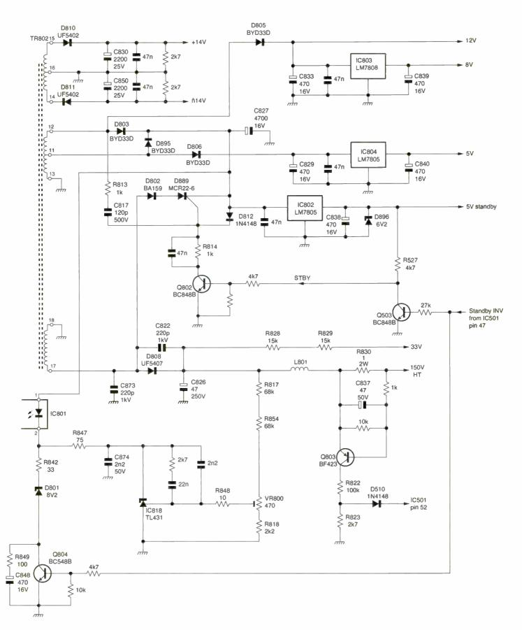
Fig. 2: Circuitry on the secondary side of the chopper power supply in the Vestel 11AK37 chassis.
