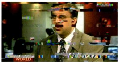
Typical example of digital picture breakup (pixellation) under poor-signal conditions, when the digital decoder can't cope.
