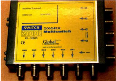
Fig. 34: The Global 5X6RX passive multiswitch.
