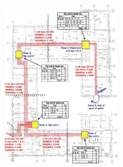
Fig. 26: Schematic of part of a system based on tap-off lines.
