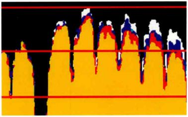
Fig. 32: An analyser display of one of the high-band polarisations. The whole satellite IF band is shown, with the low frequencies on the left. The horizontal red lines are 5dB divisions. The white, blue, red and yellow areas represent the response after 20, 40, 60 and 80m of CT100 cable respectively. The blue, red and yellow areas have been moved upwards, so that the response of the lowest multiplex is equalised. This highlights the extra signal loss at the higher frequencies.
