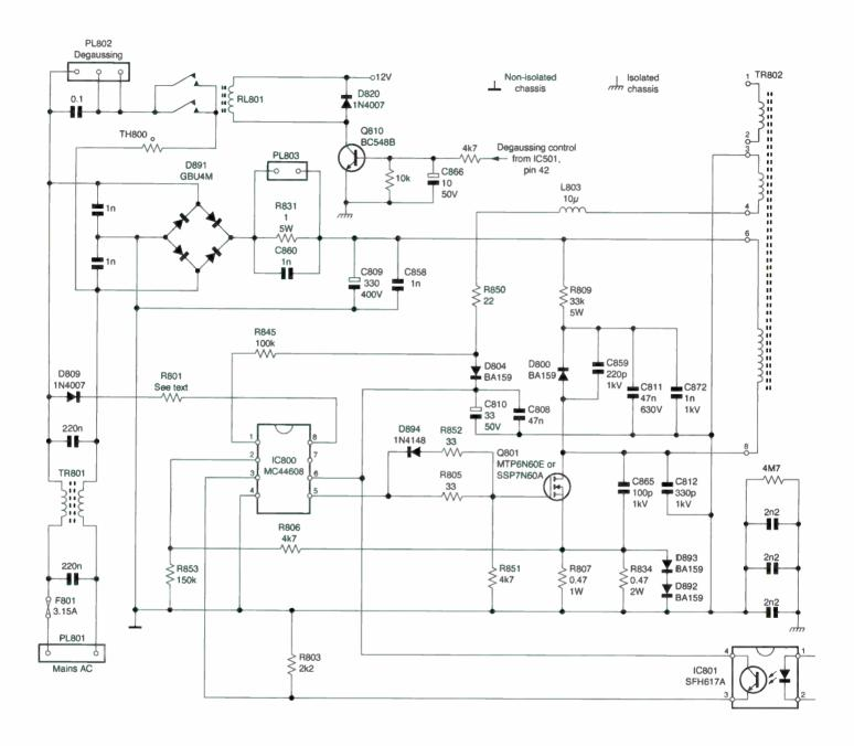
Fig. 1: Circuitry on the primary side of the chopper power supply in the Vestel 11AK37 chassis.
