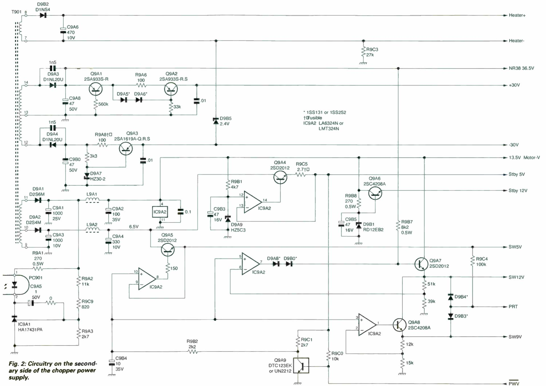
Fig. 2: Circuitry on the secondary side of the chopper power supply.
