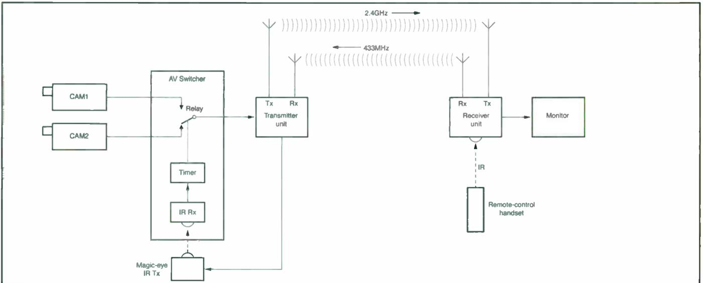
**Fig. 1: Block diagram of the AV-sender CCTV system with camera switching.**
