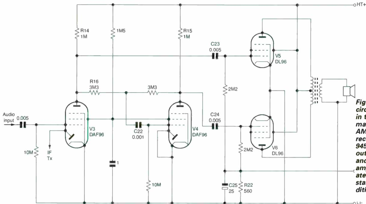
**Fig. 6: Audio circuitry used in the Ferranti mains/battery AM radio receiver Model 945, with a QPP output stage and the audio amplifiers operated under starvation conditions.**
