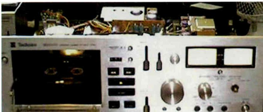
Technics. At the time Nakamichi was making the similarly over-engineered 700 Tritracer series. The unit weighs about 11kg and has clunky solenoids to operate the record/play slider switches; these solenoids are 3in. long and 1·5in. square. Smaller solenoids provide pause operation and pull the head block to the inserted cassette. There is even one to change from normal tape to chrome tape equalisation.
