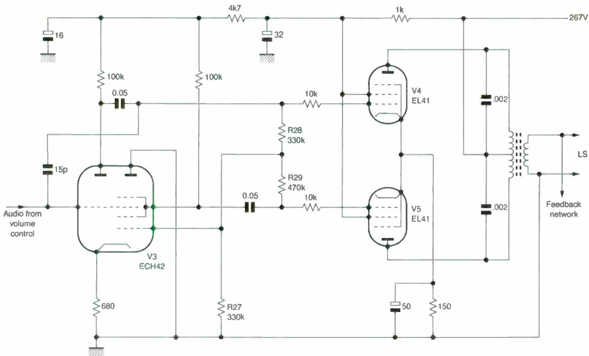
**Fig. 2:** The Pye Model P76RG used a triode-hexode frequency-changer valve as audio amplifier and phase inverter.
