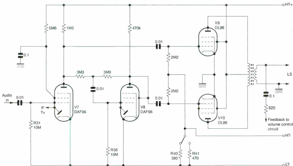
**Fig. 3:** The push-pull audio output circuitry used in the Ever Ready Sky Monarch.
