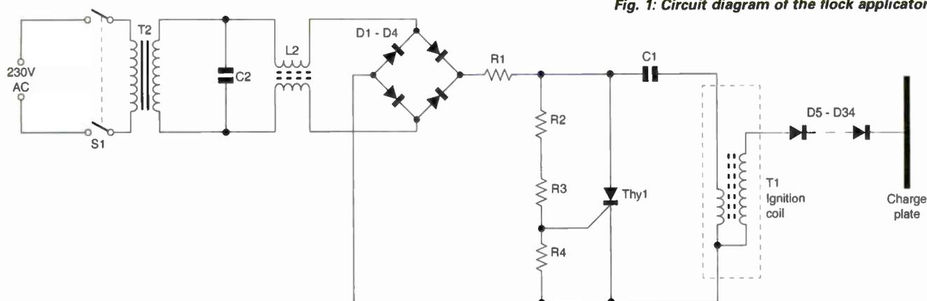
Fig. 1: Circuit diagram of the flock applicator.
