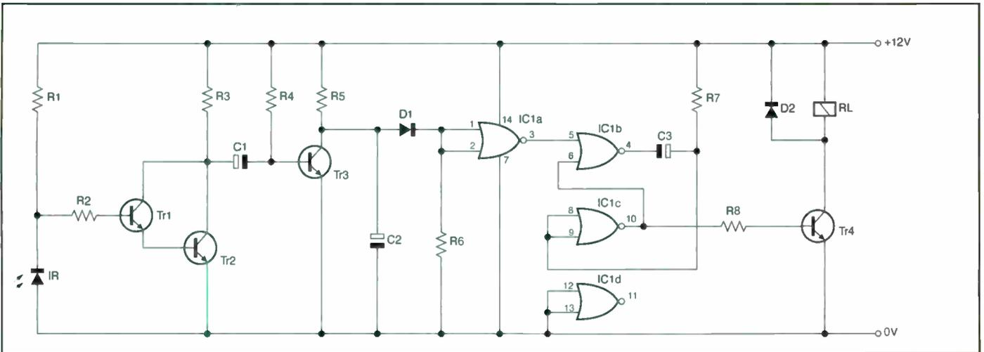
**Fig. 2: (above) Circuit diagram of the infra-red signal operated CCTV camera switcher unit.**
