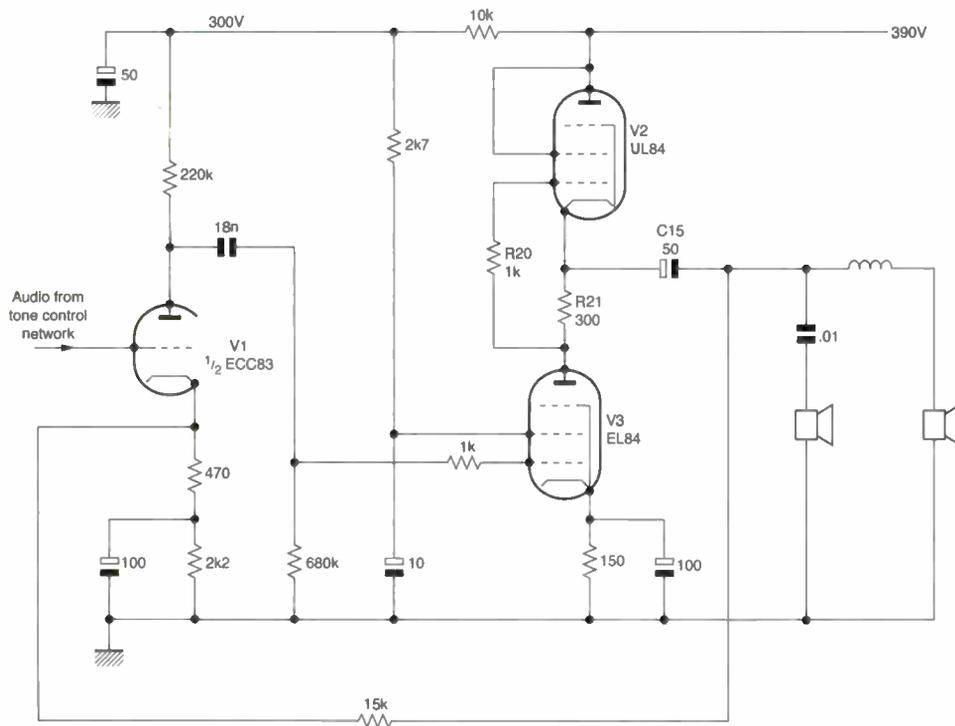
**Fig. 5: The transformerless push-pull circuit used in the Philips record player Model AG2126.**
