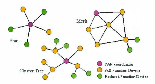
Fig. 3: How function varies depending on where a device is within the network and the network arrangement.
