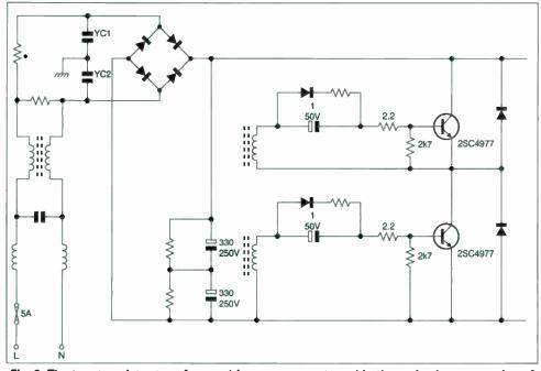
Fig. 2: The two-transistor transformer-drive arrangement used in the main chopper section of some ATX power supplies.
