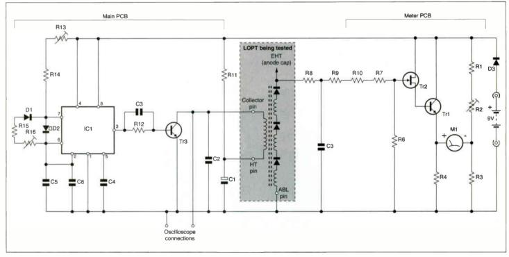
Fig. 1: Circuit diagram of the LOPT tester, which is built on two boards (main and meter).
