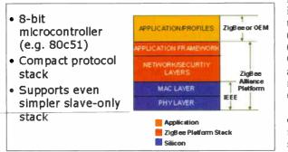
Fig. 2: The Zigbee protocol stack.
