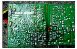
Left – Photo 2: Underside view of a typical ATX power-supply PCB, showing the clear demarcation between the primary and secondary sides of the circuitry.
