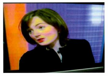
Fig. 9: Effect with one colour bit (R0) missing.
