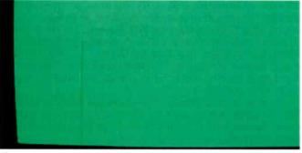
Fig. 3: A vertical line in the lower portion of a display. This indicates a data-drive fault with a dual-scan display.
