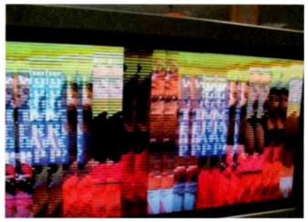
Fig. 11: An image-scalar memory fault – address line short-circuit to 0V.
