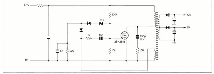
Fig. 1: Simplified circuit of a typical 5V standby section of an ATX power supply.
