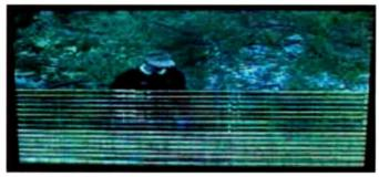
Fig. 13: Effect produced by a dry-joint at the sub-field processor.
