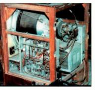
Photo 6: An experimental Murphy PAL/NTSC colour receiver that was produced in 1959.
