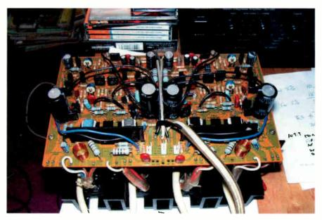
Photo 1: The Sansui AU919 power amplifier and heatsink removed from the case.
