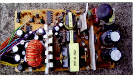
Photo 1: Top view of a typical ATX power-supply.
