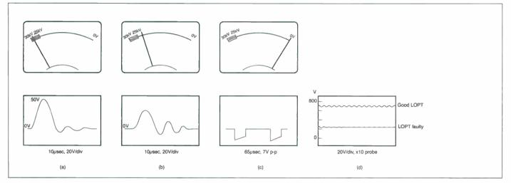
Fig. 3: (a) Meter reading and oscilloscope waveform with a good LOPT. (b) Meter reading and oscilloscope waveform with a faulty LOPT. (c) Meter reading and oscilloscope waveform with incorrect connection or an open-circuit winding. (d) Conditions at the anode connector with a good and a faulty LOPT, oscilloscope check.
