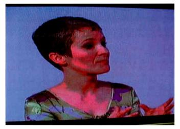
Fig. 10: Effect when one LVDS encoder data line is short-circuit to 0V.
