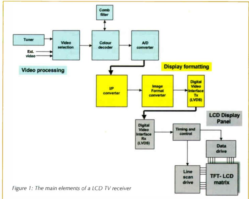
Figure 1: The main elements of a LCD TV receiver
