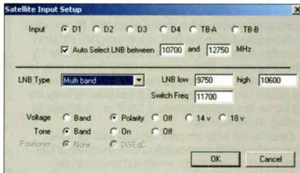
The photo above, shows a screen image of the LNB selection, as the program is intended for worldwide use it doesn't automatically default to the standard European Ku band universal LNB standard on installation. As indicated in the picture to use a universal LNB Select LNB type Multiband, lowband local oscillator 9,750 GHz, highband local oscillator 10,600 GHz and LNB switch frequency 11700.
