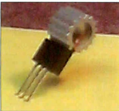
Failure of the CD to operate in this budget Hi Fi, with the laser not even homing, was caused by a defective 8v regulator transistor, Q701. Its type was completely unrecognisable, even to [www.datasheetarchive.com](http://www.datasheetarchive.com) and it's very rare to beat this excellent free-to-use web resource.
