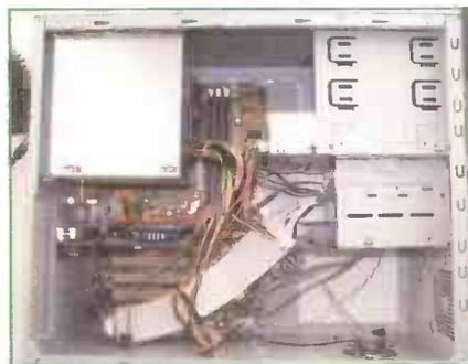
The next photo shows the completed assembly with side panels in place. Now you do not need to replace the side panels on the case yet because you never if you need to open it up again, but you are ready to connect the external devices and cables, including the monitor screen, keyboard and mouse, and finally the IEC power cable into the power supply socket.
