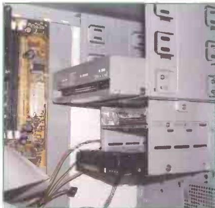
Note the position of the sockets on the various drives. The IDE drives (hard disk and CD) have sockets for power supply cables to their right as shown above, and for the IDE ribbon cables to their left.
