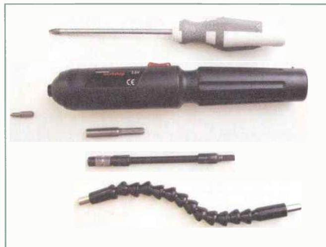
Below the power driver are some useful extensions for getting the driver bit into tricky and otherwise inaccessible spaces, particularly when using a mini tower case as we will be doing here.
