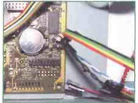
The most important convention to observe on most connections is that of the black or white cables going into the earth or ground or negative (-) pins, while just about any other colour will signify a power, signal or positive (+) pins.
