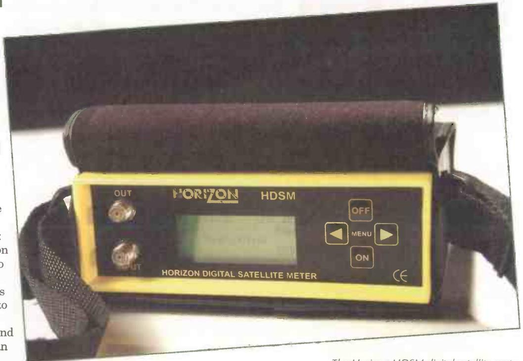
The Horizon HDSM digital satellite meter
