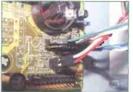
The A7S333 provides additional connectors for infrared port, front panel audio, and front panel USB, among others. The final connections should look something like the photo above.
