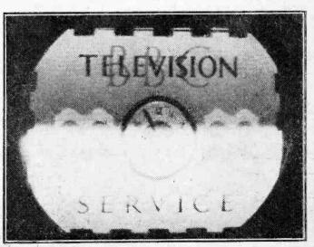
Fig. 3.—50 cycle ripple modulating the C.R. tube. (Compare with Fig. 1.) Ripple has spoiled interlace and frame linearity—lines are spread out towards top of picture.
