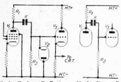
Fig. 1.—Condenser K affects the response of V3 compared with V1.
