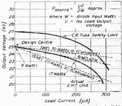
Fig. 15.—Various regulation characteristics for the E.H.T. supply unit. For clarity, the vertical scale covers only the range above 20 kV. This makes the curves appear rather worse than they really are.
