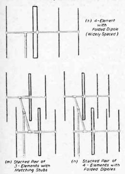
Fig. 3.—Multiple element arrays for use under difficult conditions.
