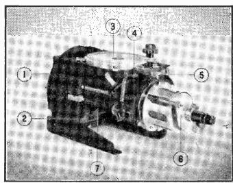
Fig. 8.—Optical unit of the system. 1. Spherical Mirror; 2. Plane Mirror; 3. Corrector Lens; 4. Yoke carrying the tube mounting, focus and deflection coils; 5. Yoke locking plate; 6. Focus coil locking screw; 7. Dustproof grommet.
