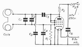
Fig. 3.—Circuit of the arrangement: R1 56 k $\Omega$  I watt; R2 10 k $\Omega$  | watt; R3 50 k $\Omega$  variable resistor; C1 100 pF; C2 50 pF variable trimmer; C3 50 pF; C4 50 pF; C5 500 pF; C6 500 pF; V—6F12, 8D3, 277, etc.
