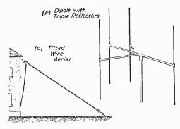
Fig. 4 (above).—The tilted wire, and a dipole with triple reflectors, and Fig. 5 (right).—A simple 'improvised' aerial made by extending the conductors of the downlead.
