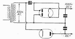
Fig. 4.—A half-wave rectifier used as a stabiliser.
