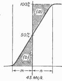
Fig. 6.—The critical part of the curve shown 'n Fig. 5 is indicated here. The sections m and n should be equal, as also should be areas (a) and (b).
