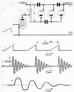
Fig. 14.—The voltage tripling circuit, waveforms of input voltage, and anode voltage.
