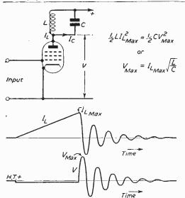
Fig. 12.-The "Ringing Choke" circuit.
