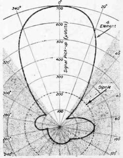
Fig. 6.—Polar diagram of vision reception only showing corresponding dipole reading.
