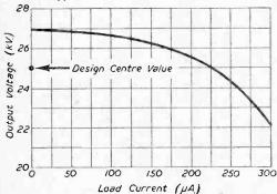
Fig. 11.-Limiting regulation curve of E.H.T. supply.
