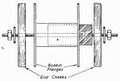
Fig. 4.—Assembly of the winding jig.
