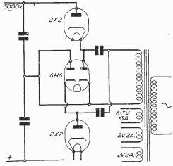
Fig. 6.-A circuit for providing E.H.T. voltages.
