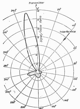
Fig. 7.—Polar diagram for signal/noise ratio for Fig. 6, with equal interference source at 40 degrees.
