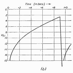
Fig. 13.—(a) Typical Anode-Current Anode Voltage diagram for a 'Ringing Choke' circuit. (b) The required grid-input waveform if the working point is to follow the line B.C.
