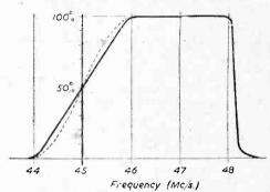
Fig. 5.—For maximum detail the vision response curve for single side-band reception should be as shown here.
