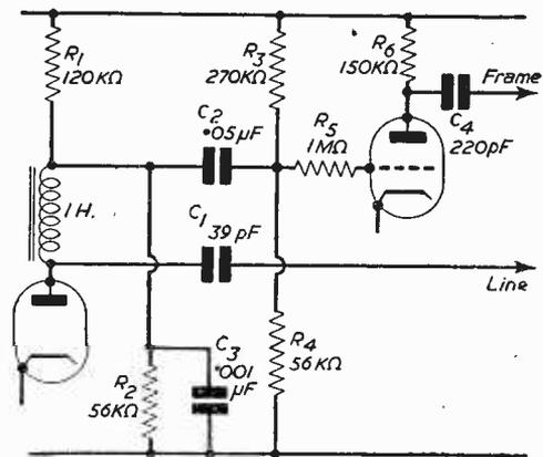
Fig. 6.—This arrangement, recommended by Mullard, uses a triode, and an iron-cored choke in place of the resistor for the anode load on line.
