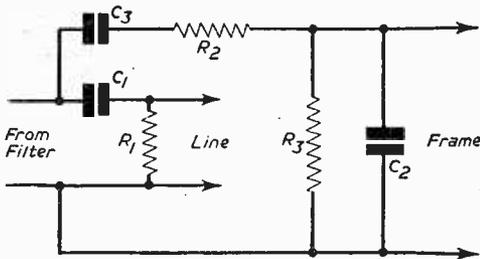
Fig. 1.—This is the basic integrator and differentiator circuit arrangements for use in frame and pulse separation. Although such an arrangement could be used following a limiter its efficiency would be low due to a variety of reasons. Compare this with the elaborate arrangement used in Figs. 4 or 6.
