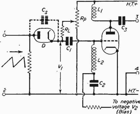
Fig. 1.—Multir circuit for the production of marker pips.
