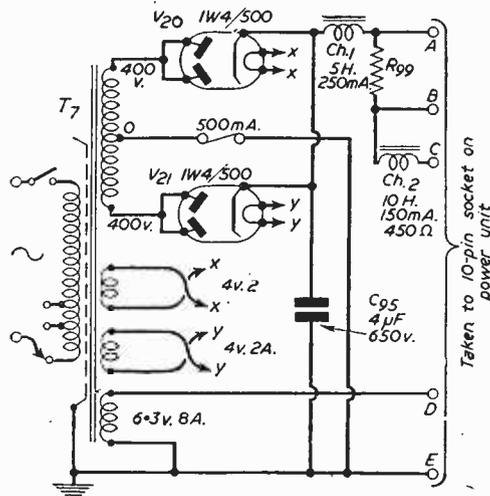
Fig. 3.—Theoretical circuit of the mains unit.
