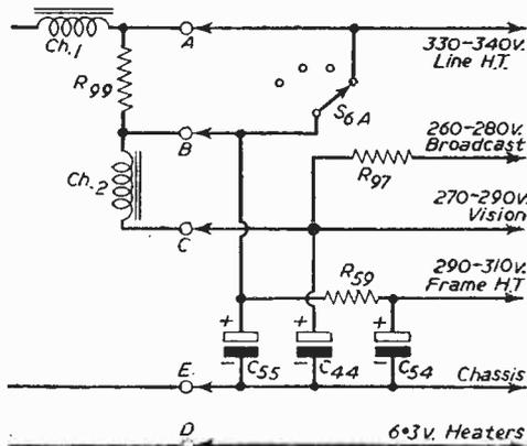
Fig. 4.—The voltage divider circuits
