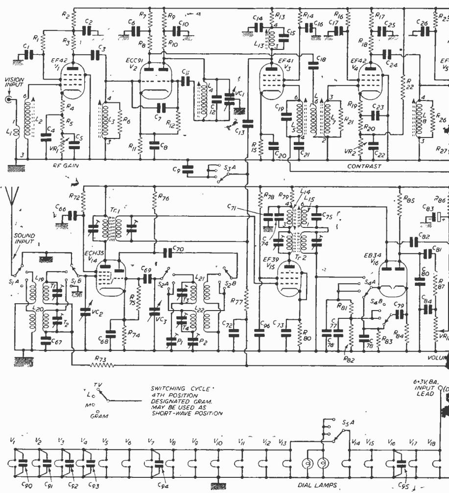
Fig. 1.—Theoretical circuit of the combined receiver, etc
