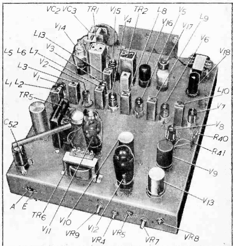
Fig. 2.—Chassis layout with essential component references.
