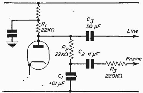
Fig. 2.—A practical interpretation of the Fig. 1 arrangement. This is the arrangement used in certain Ferguson receivers.
