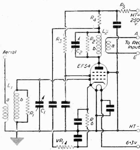
Fig. 1.—Single-valve pre-amplifier circuit.
