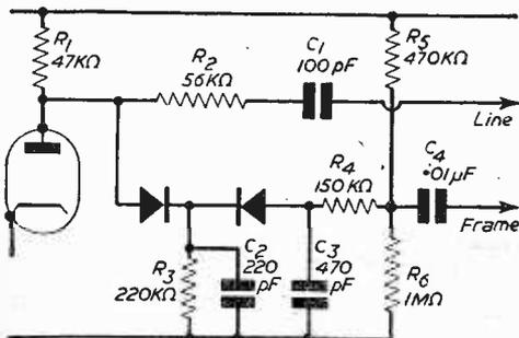
Fig. 5.—New Pye arrangement in which two rectifiers are used in place of the double diode seen in former circuits.
