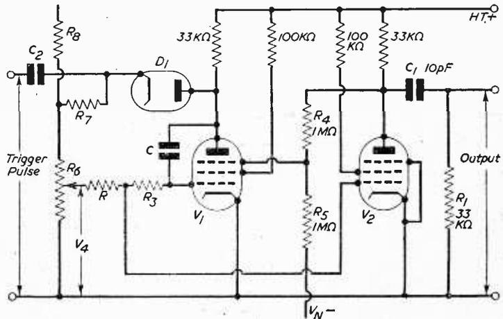
Fig. 2.—The Miller-Sanatron circuit.
