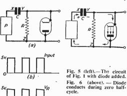
approaches that of the input waveform. It has, however, submerged until the projections on either side of the zero line are equal, and the positive and negative peaks fluctuate by .13 volts about the mean 2.5 volt value.
