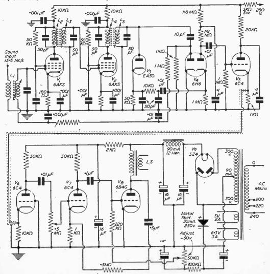
Fig. 2.—Circuit of the sound I.F. amplifier and sound amplifier power pack.
