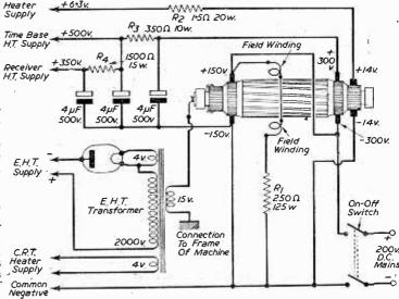
Fig. 5.—Complete circuit of power pack.
