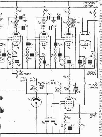
58.25 Mc/s into the aerial terminal of the receiver, rotate the oscillator tuning control and when the signal is heard at the sound receiver and a sharp dip is observed in the reading of the milliameter you know that the oscillator is on the right frequency.
