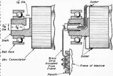
Fig. 2.—Details of holes for A.C. lead.
