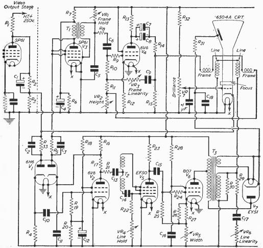
Fig. 2.-Complete circuit of the final arrangement.
