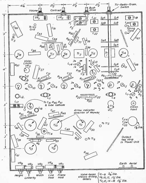
Fig. 2.—Details of chassis measurements, component positions, etc.
