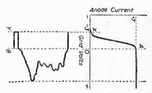
Fig. 12,-Valve characteristics required for sync separation.
