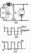
Fig. 7.—Action of circuit during D.C. restoration.
