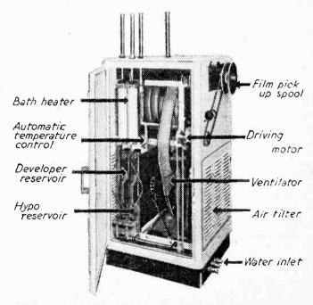
Details of the high-speed processing tank referred to above.
