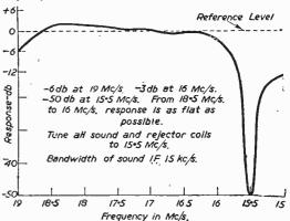
Fig. 4.—I.F. response after rejectors are tuned.
