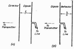
Fig. 2.—This diagram shows the essential differences between a director and reflector.
