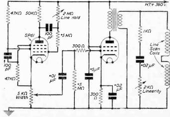
Fig. 1.—Experimental line time-base circuit.
