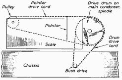
Fig. 3.—Suggested dial and condenser drive arrangement.
