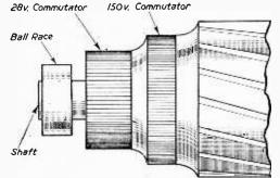
Fig. 1.—Original appearance of "A.C. end" of armature.
