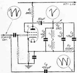
Fig. 6.-A typical R.C. coupled frame output stage, with linearity correction by N.F.B.
