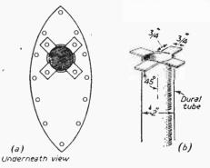
Fig. 6.—Details of the mounting required for the scheme shown in Fig. 5.
