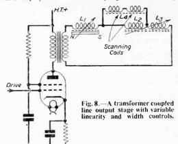
low - impedance scanning coils are usually employed, the impedance step-up being performed by the transformer. With R.C. coupling, however, the scanning coils should have an impedance similar to the optimum load value of the output valve. this being the counterpart of the anode load of an A.F. amplifier.
