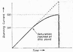
Fig. 9.—Counteracting for the exponential rise in current.
