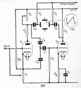
Fig. 2.—A self-linearising push-pull time-base.
