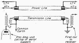
Fig. 2.—Details of the power and transmission lines.
