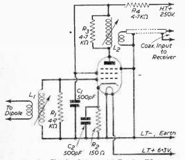
Fig. 1.-Circuit of the Aerial Pre-Amplifier.
