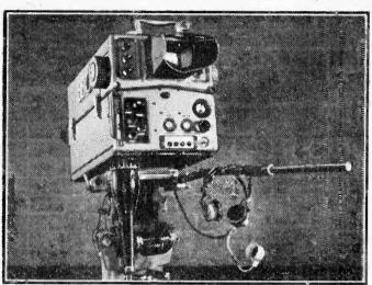
The Pye Image Orthicon camera. The lens turret is motor-operated.
