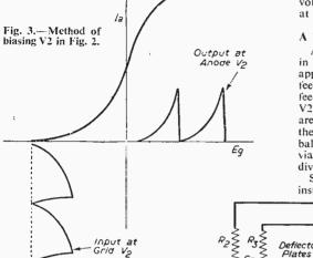
A sawtooth waveform may be analysed into a wide spectrum of frequencies and in order to preserve their wave shape the frequency response of the system should be fairly linear up to at least 10 times the fundamental frequency. In the case of the frame amplifier this is readily achieved, but at line frequency it is a different matter, for then the Miller effect and stray shunt capacitances become very important.
