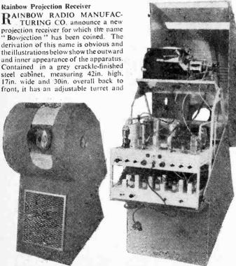
The new "Bowjection" receiver showing the internal arrangement of the various sections.
