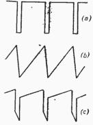
Fig. 5.—Voltage waveforms to produce a sawtooth current in (a) pure inductance, (b) resistance and (c) inductance and resistance combined.
