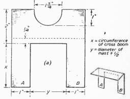
Fig. 4.—Details of the fixing clamp which can be seen in Fig. 3.
