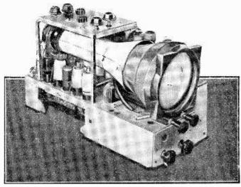
A typical converted ex-service unit complete with tube. £9 televisor using a Type 62 unit.
