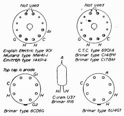
Fig. 3.-Valve base connections.
