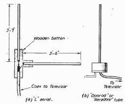
Fig. 2.—Two very simple forms of indoor aerial for areas close to the transmitter.
