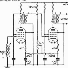
Fig. 3.—A circuit by G.E.C. showing how two stages can be controlled by a single potentiometer. The valves used are Z77's,
