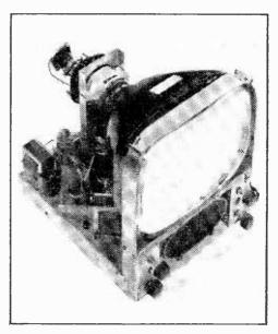
The use of eliptical speaker and rectangular tube enables the overall size of the receiver to be kept down.
