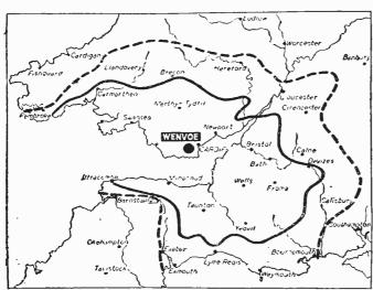
Fig. 1.—The Service area as plotted by the BBC. It may, of course, subsequently be found that results will differ slightly in certain districts, but the map may be taken as a reliable guide in planning the type of aerial which may be required.
