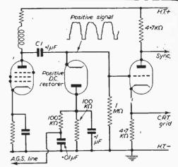
Fig. 5.-Another method of using the restorer diode,
