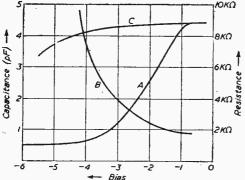
Fig. 1.—Curve A shows the change of control-grid capacitance and curve B the change of input resistance with bias. Curve C shows how the change in capacitance is reduced when both control and suppressor grids are biased.
