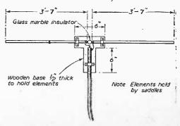
Fig. 6.—Constructional details of a dipole.
