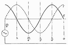
Fig. 13.—Reflected voltage and current from shortcircuited line.
