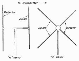
Fig. 7.—The simple "H" and the "X" type aerial. the latter having very good anti-interference properties.
