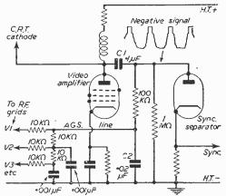
Fig. 1.—Conventional diode sync separator.
