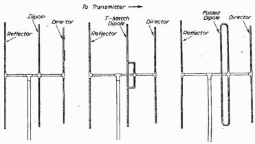
Fig. 8.—Three different forms of multi-array aerial for remoter districts.
