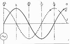
Reflected voltage and current from open circuited line Note: Current and voltage waves shown in one line only for clarity
