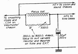
Fig. 5.—Details of the electromagnetic focus circuit.
