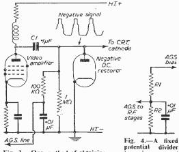
3.—One method of ohtaining A.V.C. from a restorer diode,
