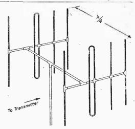
Fig. 10.—For areas of very weak signal strength an elaborate array of this type is not only desirable, but in many cases essential.
