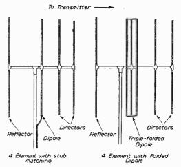
Fig. 9.—For fringe area reception aerials of this type are necessary.
