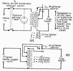
Fig. 1.—A two-winding brightener at (a), and an autotransformer brightener at (b),
