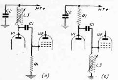
Fig. 4.—Showing at (a) a tuned anode circuit, at (b) a tuned grid circuit, and provided C1 has negligible impedance at the operating frequency, both circuits are equivalent as shown in simplified form at (c).
