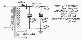
Fig. 2.—Power supply for an additional stage.
