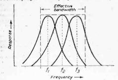
Fig. 6.—Illustrating how any desired pass-band may be obtained by the use of stagger-tuning.
