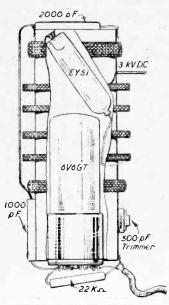
E.H.T. Coil with 6V6 G7 and EY51 inside coil (other components mounted outside)
