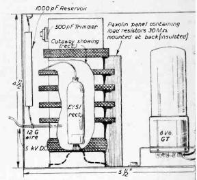
Fig. 4.—Details of the main components and layout. On the right (Fig. 5) is an alternative layout suggestion.
