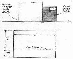
Fig. 7.-The detector screen.
