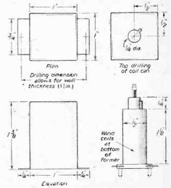
Figs. 5 and 6.—Details of coil shield cans and coil former type.
