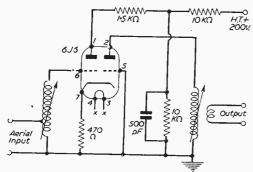
Fig. 1.-A simple grounded-grid amplifier circuit.
