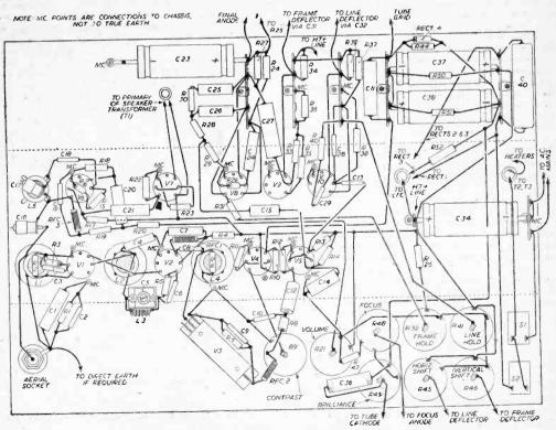
Fig. 8.—Under-chassis wiring.
