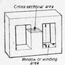
Fig. 2.—Transformer core showing the cross-sectional area and window.
