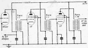
Fig. 2.—Basic Bifilar amplifier circuit.
