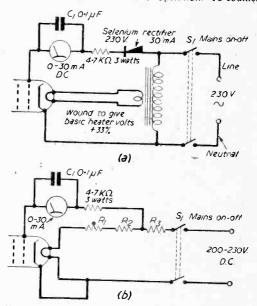
Fig. 4 (a).—Rejuvenator for A.C. supplies. (b) for D.C. supplies. Here, for 0.3A tubes R1 = CZ6 Brimistor, and R2, 3 are 260 Ω 50 W each, For 0.6 A tubes R1 = CZ4 Brimistor and R2, 3 are 130Ω90 W each.
