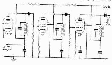
Fig. 1.-Basic single tuned stagger type amplifier.
