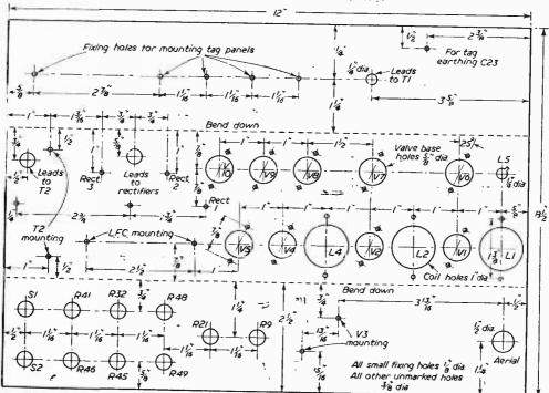
Fig. 4.—Chassis drilling diagram.
