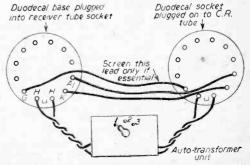
Fig. 3.—Typical arrangement of brightener unit.
