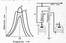
Fig. 8.—Curve (A) showing the response when two tuned circuits are undercoupled, (B) critically coupled, and (C) overcoupled.
