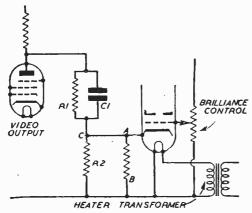
Fig. 1.—Circuit diagram illustrating the effect of the heater-cathode short-circuit on the video stage.
