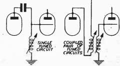
Fig. 6.—A single circuit and a coupled tuner.
