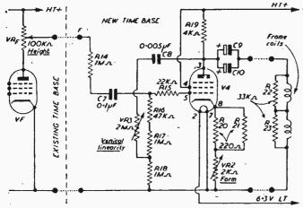
Fig. 2.—A frame timebase amplifier.
