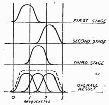
Fig. 7.—Diagram illustrating the effects of stagger tuning.
