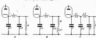
Fig. 2.— Networks as found in general types of television detector stages
