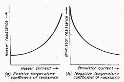
Fig. 3 (a).—A positive temperature coefficient of resistance. (b) A negative temperature coefficient of resistance.
