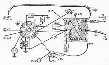
Fig. 17.—Details of the mixer stage.
