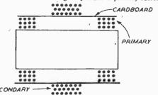
Fig. 4.—Details of the position of the secondary winding.
