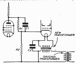
Fig. 2.-C2 short-circuits the video signal here.
