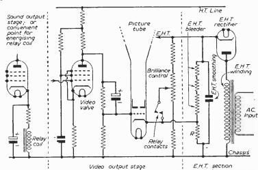
Fig. 1.—A picture-tube protection arrangement—for grid modulation.
