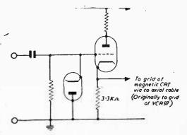
Fig. 4.—A' typical phase-splitter as used in the VCR97 timebase.
