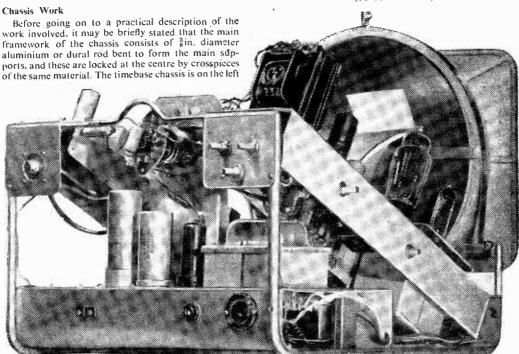
A rear view of the Lynx showing underside of timebase chassis.
