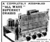
B.3.—A 5-valve 3wave band Superhet Receiver for operation on A.C. mains 100 - 120 volts and 200 - 250 volts, employing the very latest
