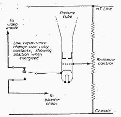
Fig. 2.—Showing how relay contacts should be modified for cathode modulated tubes.
