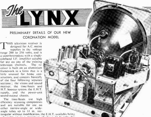
tangular without modification, the E.H.T. available being adjustable up to a maximum of about 13 K volts for use with the latter type of tube. As described, the chassis uses a 12 in. Mullard MW31-16 ion-trap tube working at 9 kV, but the mechanical changes necessary for other and larger tubes are not serious to the average constructor. Aluminised tubes may, of course, be used.
