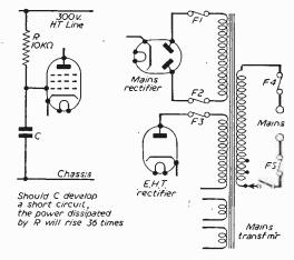
Fig. 6 (left).—Should C develop a short circuit, the power dissipated by R will rise 36 times.
