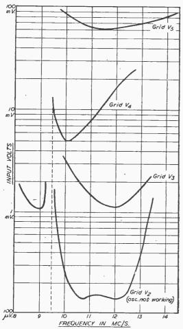
Fig. 2.—Response curves of vision I.F. stages.
