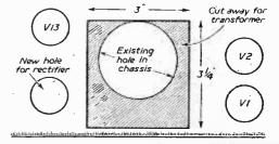
Fig. 15.—Cut-out to accommodate mains transformer.
