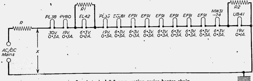
fig. 2.—A typical 0.3 amp. rating series heater chain.
