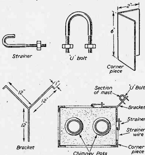
Fig. 6.—Details of chimney-lashing.
