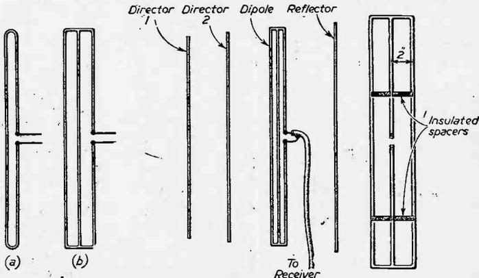
Fig. 7 (left).—Folded dipole aerials. Fig. 8 (centre).—Folded dipole with directors. Fig. 9 (right).—A triple-folded dipole.
