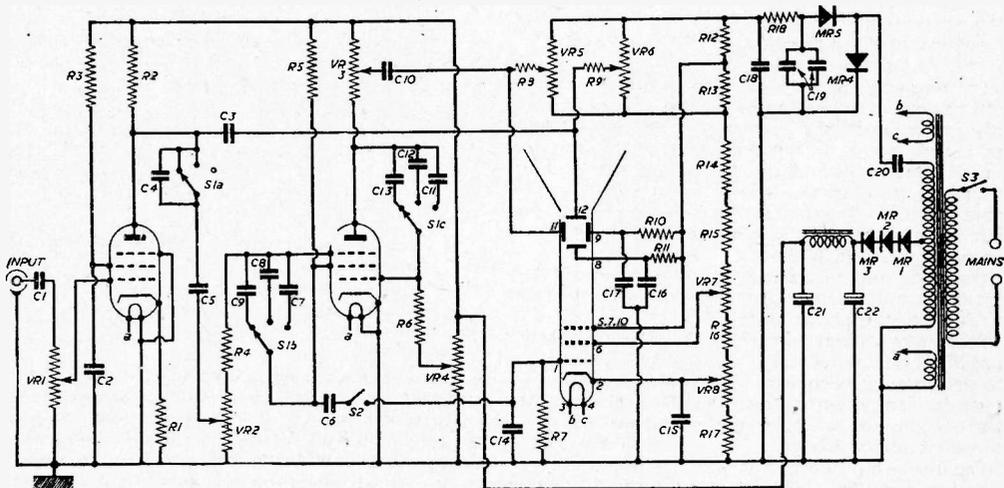
Fig. 1.—Complete theoretical circuit of the TV 'scope.
