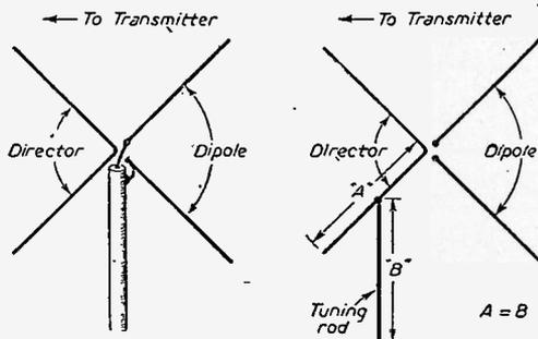
Fig. 3 (left).—Double-vee circuit. Fig. 4 (right).—A reactance tuner for double-vee aerial.
