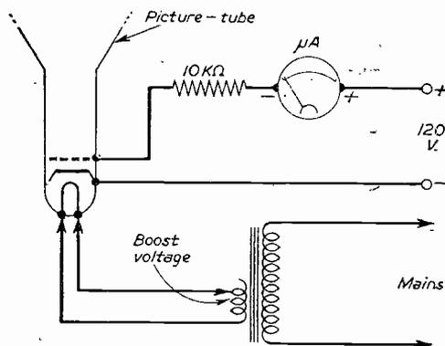
Fig. 60.—A picture-tube reactivating circuit.
