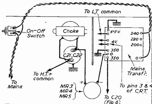
Fig. 7.—Wiring of the power supply.
