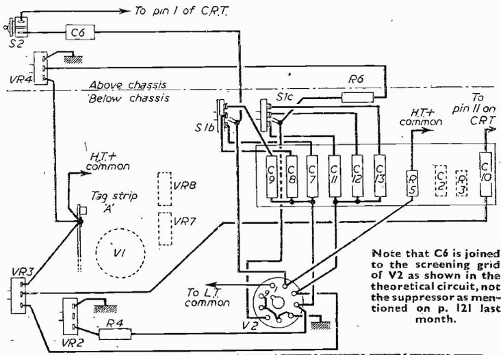
Fig. 5.—Wiring of the oscillator.
