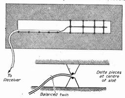
Fig. 9.—Details of the slot aerial.
