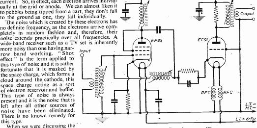
Fig. 1.—A Low-noise Cascode pre-amplifier.
