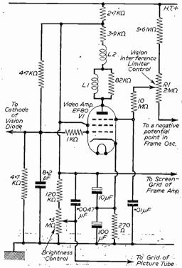
Fig. 69.—Circuit of the video amplifier stage of the Philips 1100U Series, showing vision interference limiter network.
