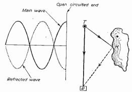
Fig. 2.—The reflected wave. Fig. 3.—Reception of one ghost,
