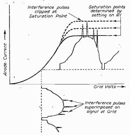
Fig. 68.—Grid volts—anode current characteristics of video amplifier in Fig. 69. Note how the valve is run into saturation current during interference pulses above peakwhite, while the peak-white signal is just below the saturation level.
