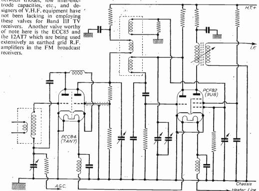
Fig. 2.—The cascode circuit as used in the latest KB receivers.
