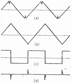
Fig. 2.—Waveforms associated with a plunger driven by a speaker cone adaption.
