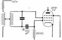
Fig. 3.—Frequency changer V2. This diagram shows how a leak in the 100 pF condenser can cause the symptoms described.
