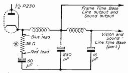
\*This resistor is mounted on the end of a paxolin panel on the left side of the upper chassis.
