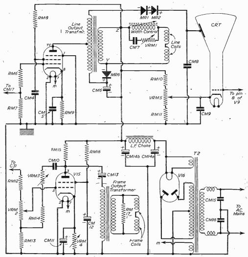
Fig. 1.—The timebase amplifier.
