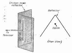
Fig. 8.—The corner reflector.
