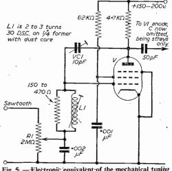
Fig. 5: — Electronic equivalent of the mechanical tuning systems.
