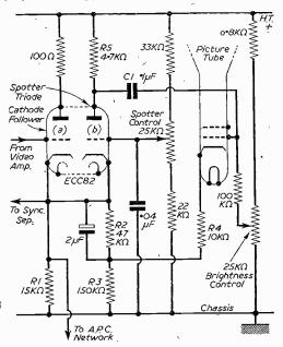
Fig. 70.—Circuit of white spot suppressor as used in the Pye V4 series.
