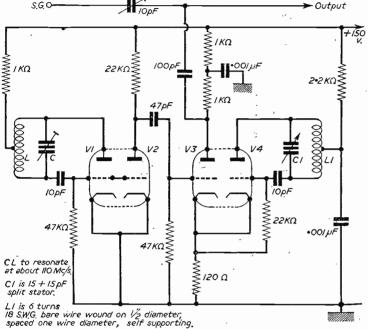
Fig. 3. — A simple sweep circuit.
