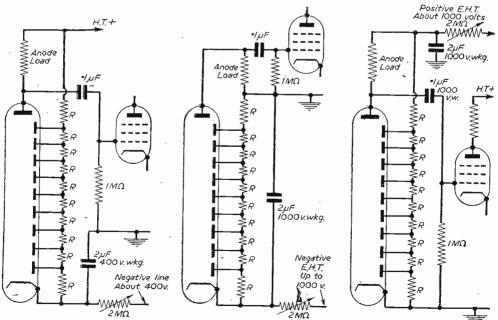
Figs. 1, 2 and 3.—Circuits for the 931A. In these diagrams the cell has been shown elongated for convenience in showing the voltage supplies to the dynodes:
