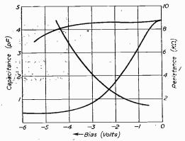
Fig. 71. — Curves (a) and (b) respectively show how the input capacitance and resistance change with grid bias potential. Curve (c) shows how the capacitance change is reduced when both control and suppressor grids are biased.
