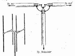
Figs. 6 and 7.—A double "H" aerial and the cable connections for a double "H."
