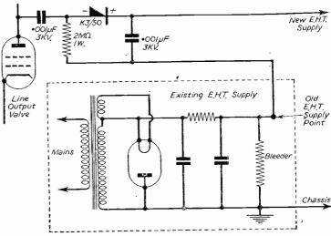
Fig. 5.- A typical flyback E.H.T. circuit.
