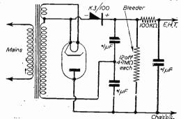
Fig 2.—The standard doubler circuit.
