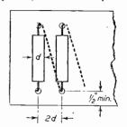
Fig. 5.—Method of mounting resistors to form the voltage-dropping chain.
