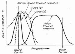
Fig. 90.—The sound and vision responses of a single sideband receiver, showing how the vision signal may gain admittance to the sound channel by curve (a) if the sound channel bandwidth is too wide, or by curve (b) if the sound channel is mis-tuned.
