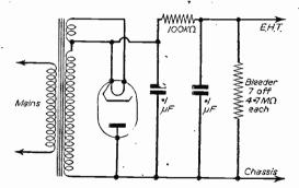
Fig. 1.—A standard mains E.H.T. circuit.
