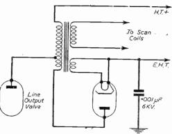
Fig. 6.—Typical flyback E.H.T. circuit.
