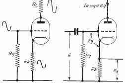
Fig. 1 (left).—Resistance-loaded amplifier with cathode bias. Fig. 2 (right).—Cathode follower,
