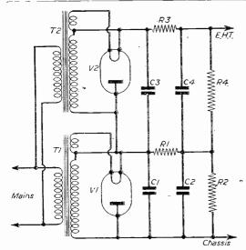
Fig. 3.-A doubler circuit using two transformers.
