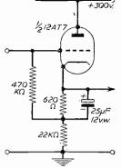
of course, vary, but the assumption of a mean value, such as that quoted in valve tables, gives reasonable results in practice. Another effect overlooked is that due to the variation of the "cut-off" grid voltage as the anode-cathode voltage of the valve alters. This can be ignored if a reasonable safety margin is allowed on the amplitude of the input signal catered for.
