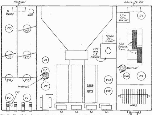
Fig. 5.—Simplified under-view of chassis. Note position of C17, 15 pF grid-coupling condenser which is difficult to replace.
