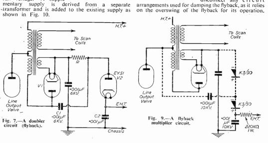
Note carefully the direction of positive and negative of both the rectifier and the electrolytic condenser.
