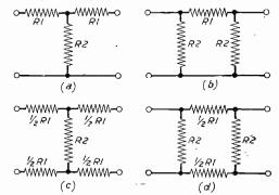
Fig. 88.—Attenuators: (a) "T" type for coaxial feeders; (b) "pi" type for coaxial feeders; feeders; (b) "pi" type for coaxial feeders; (c) "T" type for twin feeders; (d) "pi" type for twin feeders.
