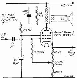
Fig. 89.—The sound output stage of K.B. FV30, FV40 and FV50 series receivers.
