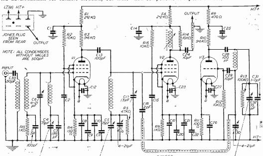
Circuit of the R.F. unit No. 26, referred to as Fig. 4 in the article on RF Units on page 408 of last month's issue.
