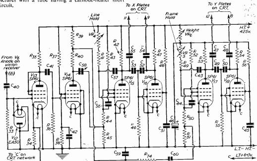
Fig. 1.—The original timebase circuit.
