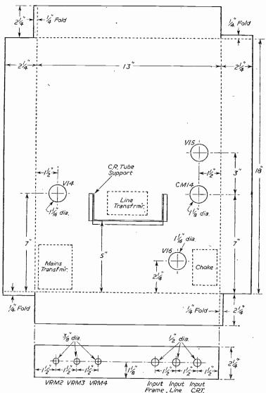
Fig. 2. — Details of the new chassis and position of various parts.
