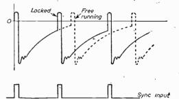
Fig. 4.—This diagram shows how the free-running condition is taken charge of by the Hold setting.
