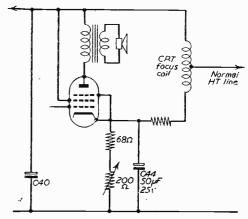
Fig. 3.—Showing the effect of the sound output stage on focusing.
