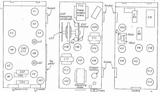
Fig. 1 (left).—Under-chassis view of R.F. unit. C22 and 23 are video amplifier electrolytics; C40 and 73 are main smoothing condensers; C44 is sound output bias condenser. (Centre).—Top view of timebase and power unit, and (right) underview of this unit in which C71 is reservoir condenser. C64 and 65 are frame-output electrolytics, and R103 is series framehold resistor.
