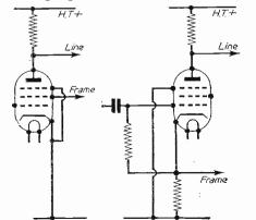
Fig. 2.—Two methods of taking out the sync. pulses to avoid interaction.
