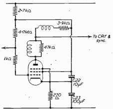
Fig. 2.—Video amplifier circuit showing the electrolytic condensers.
