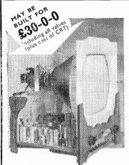
THE COMPLETE TELEVISOR IS SAFE TO HANDLE, BEING COMPLETELY ISOLATED FROM THE MAINS BY A DOUBLE WOUND MAINS TRANS-DOUBLE WOUND MAINS TRANS-FORMER. ALL PRESET CONTROLS CAN BE ADJUSTED FROM THE FRONT, MAKING SETTING UP VERY SIMPLE.
