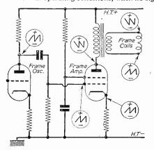
Fig. 2.—Showing sawtooth waveform at different points.
