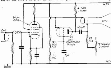
Fig. 5 .- "Black spotter" limiter, using extra triode valve.
