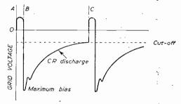
Fig. 2.-Waveform across the condenser C of Fig. 1.
