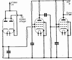
Fig. 3.—The ideal sync. separator arrangement, with isolation of picture pulses.
