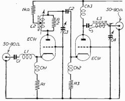
Fig. 2. - A two-stage amplifier suitable for Band III.
