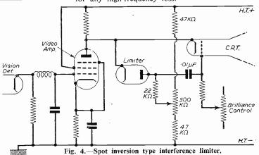
The extra amplification needed for the limiter circuit is obtained by using a tapped video load and it is an advantage to increase the H.T., if possible, to compensate for this additional
