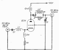
Fig. 1. - A single stage, grounded-grid amplifier.
