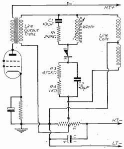
Fig. 2.—Method to be used when a damping diode is included.
