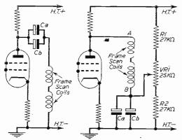
Fig. 3 (left). — Normal high impedance frame circuit. Fig. 4 (right). — Shift controls added to the Fig. 3 arrangement.
