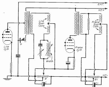
Fig. 5. — Circuit for two shift controls — frame and line.
