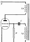
Fig. 1.—A typical circuit of a blocking oscillator.
