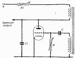
Fig. 3.—The variable resistor, R1, affects the amplitude and also the linearity of the waveform.
