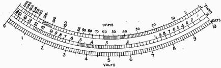
This scale may be cut out and stuck to the scale board. It is accurately drawn for this instrument.
