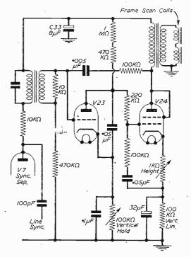
Fig. 1.—Frame timebase. Note  $32\mu F$  vertical linearity bypass. This circuit is for early table models only as far as the method of feeding frame pulses from sync separation are concerned.
