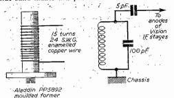
Fig. 3.—Suitable rejector for use with ex-Government I.F. strips.
