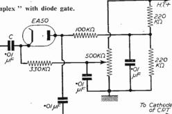
Fig. 15.-Diode with separate potential divider.
