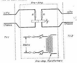
Fig. 5.—Using a mains-operated relay for switching on and off.
