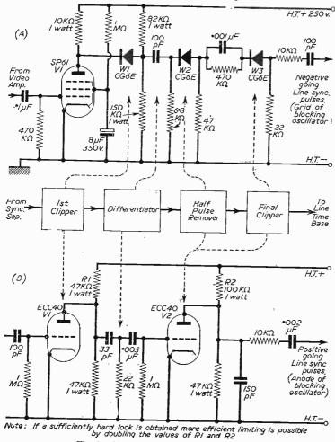
Fig. 2.—Two methods of line-pulse shaping.
