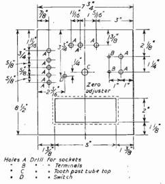
Fig. 1. — Details of the plywood top of instrument.
