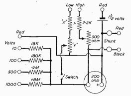
Fig. 11.—Circuit of the meter.
