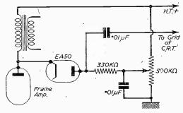
Fig. 16.-Directly-coupled gate.
