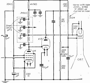
Fig. 3.—Video amplifier, noise limiter and CRT circuit. R124 is located beneath the chassis, adjacent to the radio aerial sockets.
