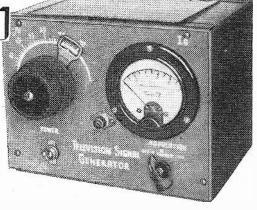
practice the oscillator frequency reaches a steady value within one minute of switching on and the long-term frequency stability has been found to be very good.
