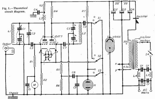
ing 200 volts at 30 mA and 6.3 volts at 1.5 amps., followed by a metal rectifier feeding a resistance capacity smoothing network. Where test gear is concerned it is well worth paying a few shillings extra for a completely isolated mains transformer as there is a very real danger when using unisolated test equipment with A.C./D.C. television receivers. To reduce radiation from the unit via the mains lead an R.F.
