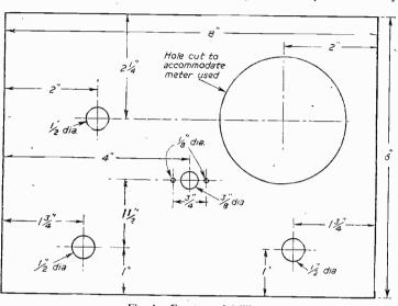
Fig. 4.—Front panel drilling.
