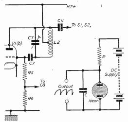
Fig. 2 (left).—Alternative 81 kc/s oscillator circuit if centre-tapped coil is available. CT=250 pF trimmer. R4, C5 and C6 are not required. Fig. 3 (right).—Basic circuit of a neon relaxation oscillator. The D.C. supply charges C through R until the potential of C is sufficient to cause the neon to strike. On striking, the neon discharges C and the cycle is repeated.
