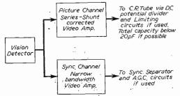
Fig. 1(a).—Block diagram of picture and sync channels.
