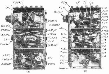
the TV sound, connect a Fig. 4.—Details of the lower chassis. (Left, before modification; Right, after.)
