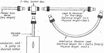
Fig. 7.—Coupling in the variable stub.
