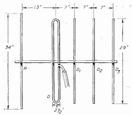
Fig. 2.—A Yagi array with folded dipole.
