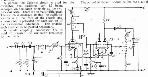
Fig. 1.-Complete circuit of the tuner.
