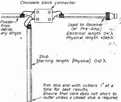
Fig. 5.—A simple matching stub arrangement.
