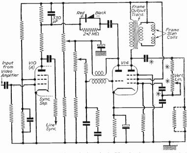
Fig. 3.—Sync senarator and frame timebase circuit. (Note that the components marked with a star are linearity feedback components which can cause flashing or arcing at the valve base of V14 if faulty.
