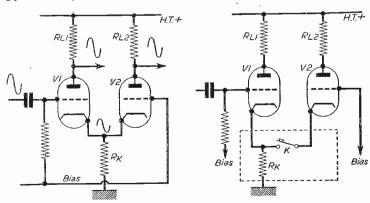
Fig. 1 (left).—Basic long-tailed pair circuit. Fig. 2 (right),—Development of the circuit.
