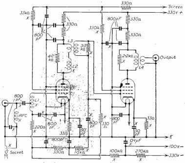
Fig. 1. - Circuit before modification.
