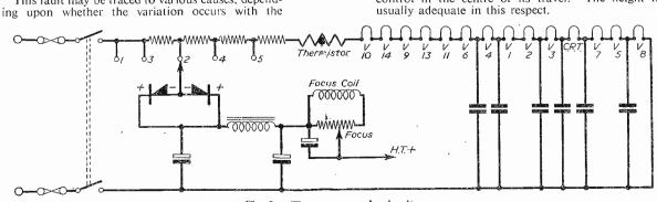
Fig. 2. —The power supply circuit.
