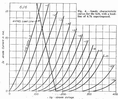
If a sine wave is applied to the grid of V1 in the circuit of Fig. 1, and the amplitude is large enough to cut the valve off, then the rapid change in cathode current can be made to produce a square wave at V2 anode. To do this, the anode current in V2 must be initially cut off. This is achieved by biasing the grids separately, that of V2 being more negative than V1 grid.
