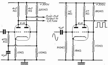
Fig. 5 (left).—Paraphase amplifier circuit for cathode ray tube. Fig. 6 (right).— Long-tailed pair clipper circuit.
