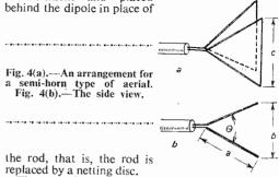
The use of such an arrangement is only justified in areas of very poor signal strength which suffer from interfering signals from behind the array.
