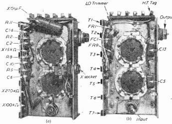
Fig. 3. - Details of the upper chassis. (Left, before modification; Right, after.)
