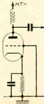
Fig. 2. — Grounding the grid.
