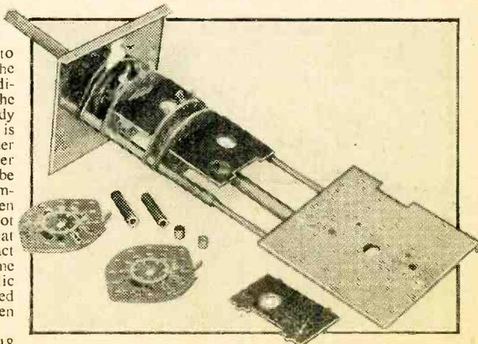
Component parts of the switch assembly.
