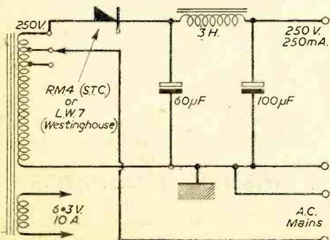
Fig. 5.—Half-wave system directly connected to mains. Boosted if below this voltage. Note the high values of the capacitors.
