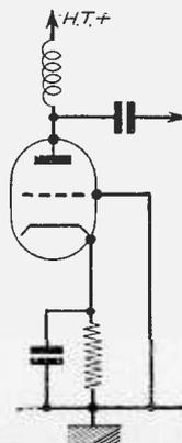
Fig. 2. — Grounding the grid.
