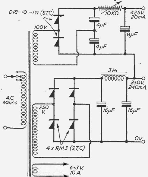
Fig. 4.—A more economical supply for a VCR97 Receiver, which can later be used for a magnetic picture tube if required.
