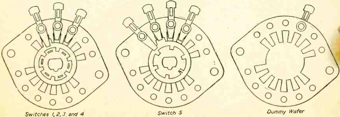
Fig. 3.—Details of the six switch wafers.
