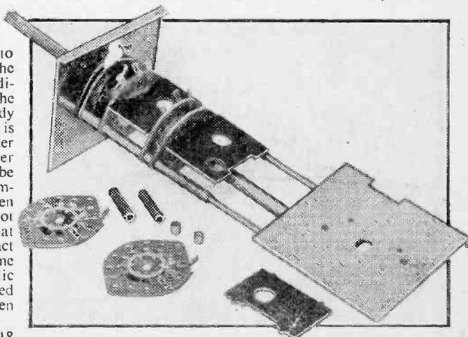
Component parts of the switch assembly.
