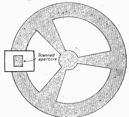
Fig. 1.—Showing the principle of Baird's original colour disc scanner which used three spiral sets of holes, one set for each colour.
