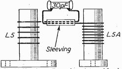
Fig. 5.—How the coupling condenser between L5 and L5A is arranged.
