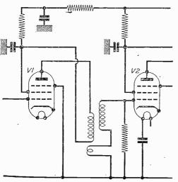
Fig. 1.—Circuit of the I.F. coil as originally published.
