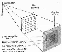
Fig. 1 .-- An illustration of the shadow effect.
