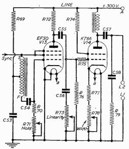
Fig. 12.—Typical simple form of line timebase.
