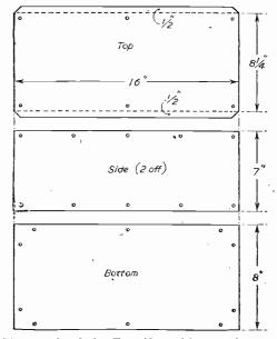
Figs. 17, 18 and 19.-Top, sides and bottom of chassis.
