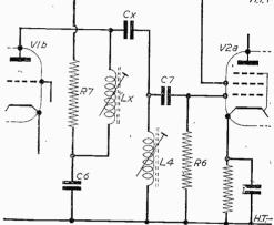
Fig. 4.—Circuit of the modifications to the Teletron Converter. Cx is 2 pF, and Lx consists of three turns widely spaced.
