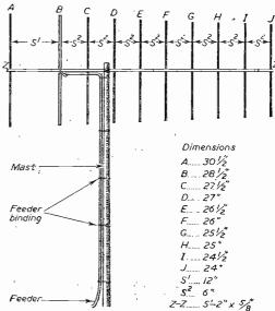
Fig. 1.—Details of the 10-element beam aerial described here.
