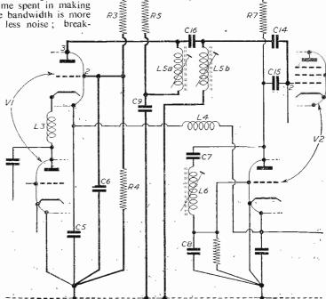
Fig. 2.-Modifications to the P.T. Converter shown in heavy lines.
