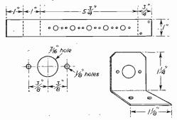
Figs. 14 and 15.-Details of the potentiometer bracket.
