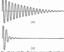
Fig. 23 (A and B).—Response curves with sound and faulty line transformers.
