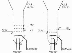
Fig. 1.—Showing pentode base and internal connections.
