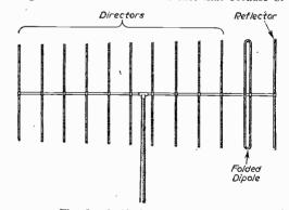
Fig. 3.—A 12-element array.
