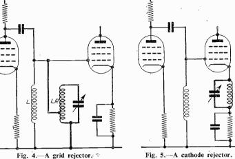
Fig. 5.-A cathode rejector.
