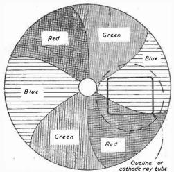
Fig. 2.—The actual shape of the colour filter disc used in the CBS frame sequential system depends on its position with respect to the cathode-ray tube. It must be over twice the diameter of the tube, and projection tubes were often employed on account of their small size,
