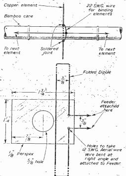
Figs. 2 and 3.—Method of connecting up the elements, and the folded dipole mounting block.
