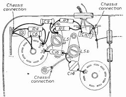
Fig. 1.—Location of the new coil L5a and new position of existing components in the P.T. Converter.
