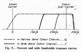
the figure. The chrominance carrier is normally generated at 2.65781 Mc/s, modulated with the chrominance signal, mixed with the normal luminance video signal and then passed to the transmitter in the normal way.
