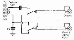
Fig. 3.—Output switching.
