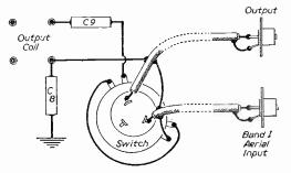
Fig. 8.—Practical arrangement of Fig. 3.
