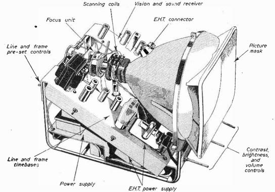
Fig. 16 .-. A home-built television receiver with the important parts identified.
