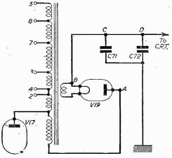
Fig: 3.-Testing points on electromagnetic EHT.
