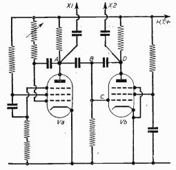
Fig. 6.—Typical paraphase circuit.
