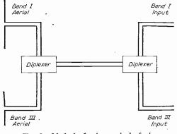
Fig. 6.-Method of using a single feeder.
