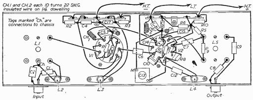
Fig. 1.-Layout and wiring of the converter.
