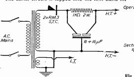
Fig. 4.—Suitable power supply unit.
