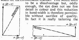
Fig. 3.—Showing how a variation of colour is produced by combining the signals of different amplitudes.
