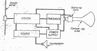
board is being televised. If the width—Fig. 15.—Block diagram of a modern television receiver showing the of the scanning line corresponds to the
