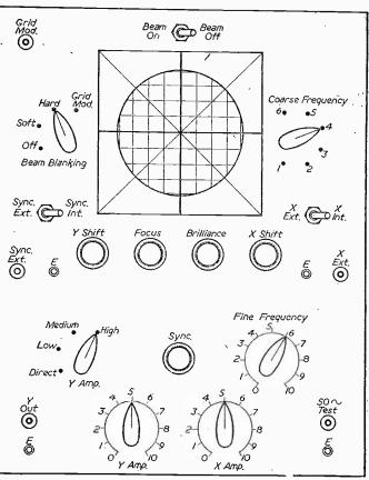
Diagram of the controls for the finished instrument,
