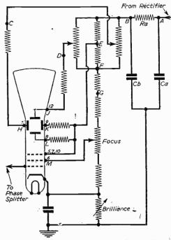
Fig. 2.—Testing points on electrostatic EHT.
