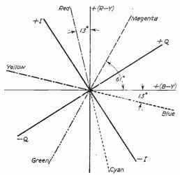
Fig. 2. — Phase diagram showing the relative phase of the (R-Y) and (B-Y) signals, and also of the 1 and Q signals.
