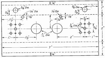
Fig. 7.-Details of the chassis.
