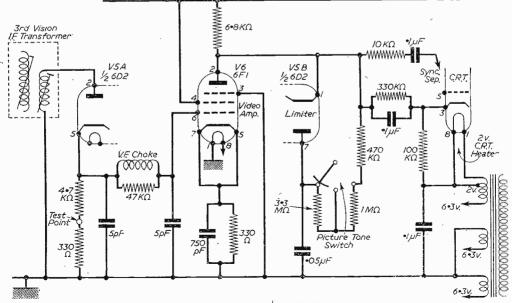
Fig. 2.—Circuit showing the C.R.T. wiring.
