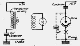
Figs. 9, 10 and 11. Testing for continuity; an oscillator tester, and (right) a condenser test.
