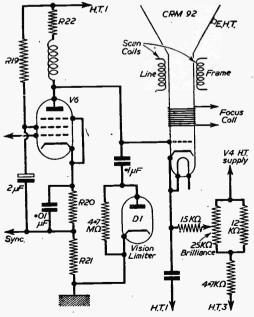
Fig. 2.-Video amplifier output, C.R.T. and brilliance circuit.
