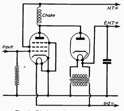
Fig. 1.-Ringing choke output circuit.
