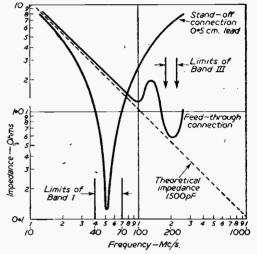
Fig. 1.-Set of curves for a Dubilier stand-off insulator, reproduced by courtesy of Messrs. Dubilier.
