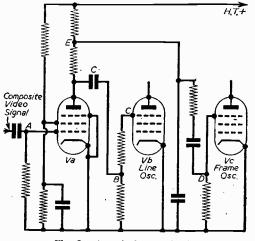
Fig. 8.—A typical sync circuit.
