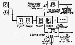
Fig. 20.—A block diagram similar to Fig. 19, but relating to a superhet receiver. See also Fig. 21.
