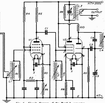
Fig. 6.-Circuit diagram of the Band I converter.
