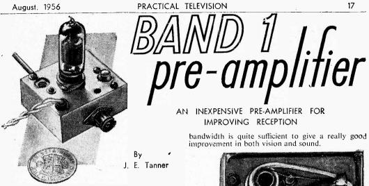
THE writer was asked to try to improve the reception on a friend's TV. After checking the valves in the R.F. stages, it was decided that a pre-amp, was necessary, and the one shown here was built and is proving very successful; there are no special circuits and everything is quite straightforward. The main feature of it is its small size-only 21in, x 2in, x 31in, with valve.
