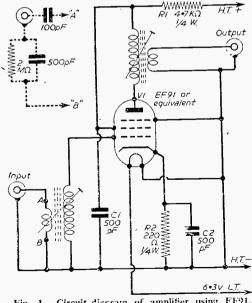
Fig. 1.-Circuit diagram of amplifier using EF91.
