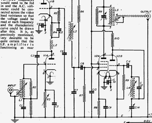
Fig. 4.-Circuit diagram of the Band III converter.
