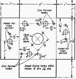
Fig. 2.-Showing drilling and fixing hole details.
