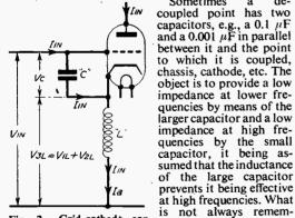
Fig. 2.-Grid-cathode capacity (C) and circuit constants.
