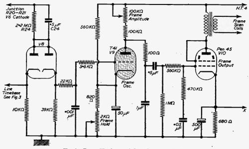
Fig. 4.-Frame Timebase and Sync Separator circuit.
