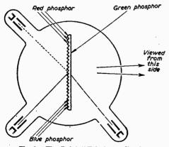
Fig. 1.-The Baird "Telechrome" tube.
