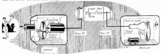
Fig. 36. - A disc colour system as used by the C.B.S. of America.
