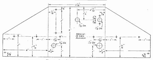
Fig. 6.—Case bending and drilling details.
