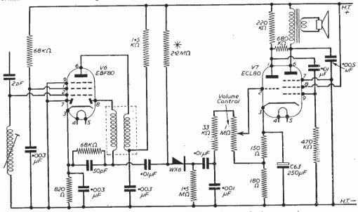
Fig. 7 .- Sound I.F., detector, limiter and output circuit.
