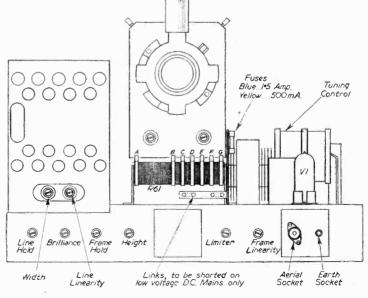
Fig. 2.-A rear chassis view.
