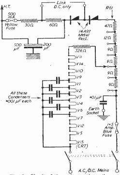
Fig. 6.—Circuit of the mains supply section.
