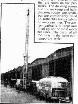
An O.B. control room (to the right of the picture), with an Eagle Tower which enables the mobile mast to be raised to 60ft.
