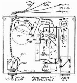
Fig. 4.—Under chassis wiring scheme.
