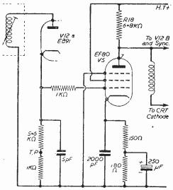
Fig. 3.-Detector and video amplifier circuit.
