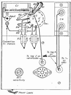
Fig. 5.-Above chassis and panel wiring details.
