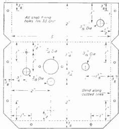
Fig. 2. Chassis bending and drilling details.
