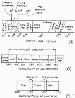
Fig. 32.—The complete electromagnetic spectrum (a); the visible spectrum (b) and (c) simplification for colour television.
