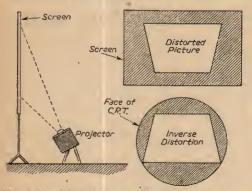
Figs. 1, 2 and 3.—A screen and projector at angle to each other and the resultant distorted picture.
