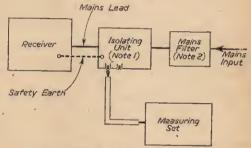
Note I. A measurement is made of the Interference voltage existing between each Mains lead and earth.
