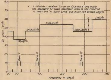
Fig. 1. - . Limits for R.F. oscillator radiation.
