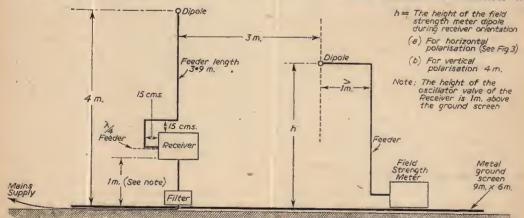
Fig. 2. - Measurement of R.F. oscillator radiation.
