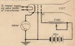
Fig. 3.—The meter may be used in the grid circuit to read grid current, but this was not successful, so the meter was placed in the cathode circuit.
