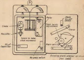
Fig. 3.—Details of the parts. The silencer is the large central circle.
