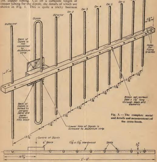
especially the bending, and a full-size paper drawing should preferably be made, as shown in Fig. 1, but without dimensions. As the bending proceeds this will act as an accurate guide or template. A piece of string measured around the outside of the drawing will give the exact length of tubing required. Do not
