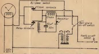
Fig. 1.—Theoretical circuit of the automatic clock switch.
