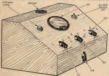
Fig. 2.—A suggested containing case for the tester. S4 should also have a scale.
