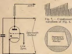
Fig. 5. —A basic timebase circuit.
