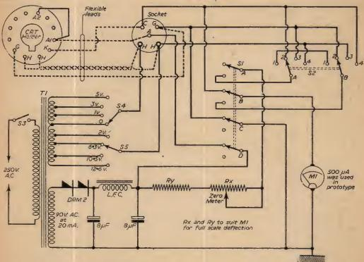
Fig. 1.—Theoretical circuit. S2 A and B are the shorts test switch. Position 1. Zero meter. Position 2. Cathode' grid. Position 3. Grid heater. Position 4. Heater cathode. Read on meter, if no reading, tube has no shorts. Shorts show up on meter as a deflection clockwise, S4 and S5 are set at 6.3 yotts.
