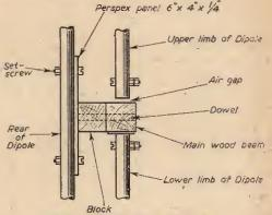
Fig. 4.-Details of the dipole gap.
