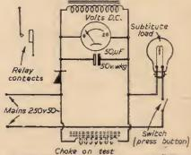
Fig. 4.—Experimental circuit for obtaining suitable value of inductance.
