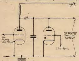
Fig. 6. -- A frame timebase circuit.
