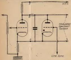
Fig. 10. - Gain control fitted to adjust slopes of sides.
