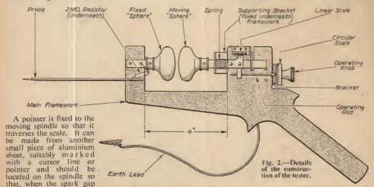
is closed, the pointer is at or near to the zero end of the scale. The exact position is unimportant, since the scale position is quite arbitrary.
