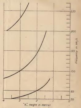
Fig. 3. - Field strength meter aerial height during receiver orientation.
