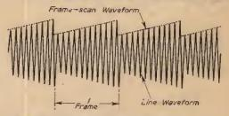
Number of lines greatly reduced to facilitate presentation Fig. 4.—Waveform of frame scan.
