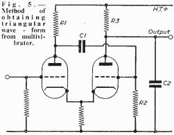
timebase, the multivibrator frequency is made much higher than the required sweep frequency, and the anode load of the output valve is made much higher than usual.
