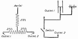
Fig. 1 (Left).—Theoretical circuit for two outlets. Fig. 3 (Right).—Arrangement of the switching system.
