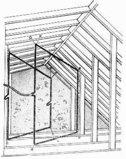
Fig. 2.—Optimum positioning of the author's aerial in the loft.
