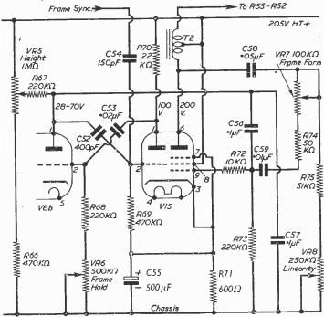
Frame oscillator and output stages.
