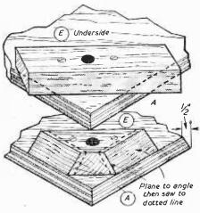
Fig. 3 (above).—Fixing the apron.
