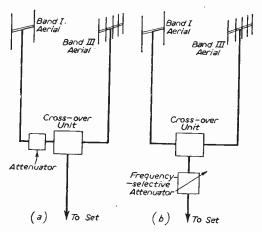
Fig. 2.—Showing at (a) the position for the introduction of an attenuator for eliminating cross-modulation on Band I, and at (h) the position for a frequencyselective attenuator which serves to adjust the level of the Band I signal with respect to the Band II signal, which is hardly affected by the unit. This method is essential where a combined aerial and single downlead are adopted.
