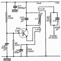
Fig. 4.—The transistorised local oscillator.
