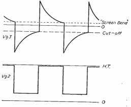
Fig. 2.—Waveforms in the transitron,
