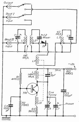
Fig. 2.—A Channel 9 to Channel 1 Converter.
