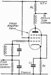
Fig. 1.—Sensitivity increase of the video amplifier can be accomplished either by increasing the value of Cc or RL.
