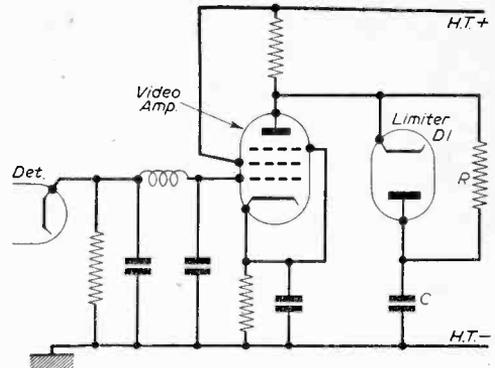
**Fig. 1.—Simple automatic type of vision limiter.**
