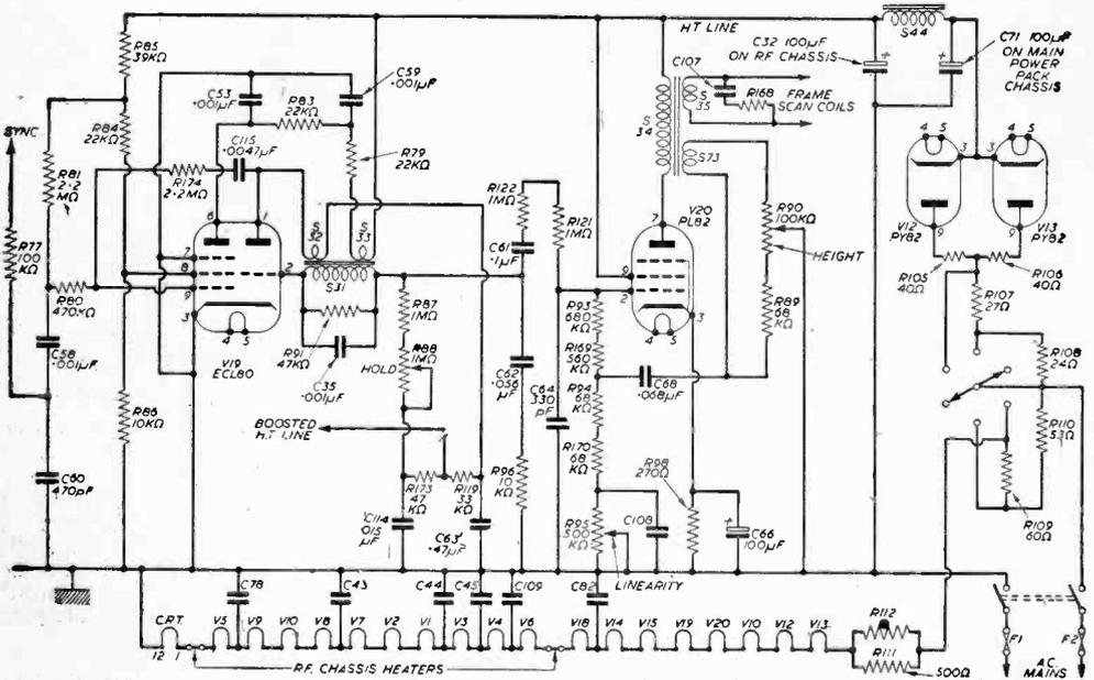
Fig. 2.—H.T. supply and frame timebase circuits.
