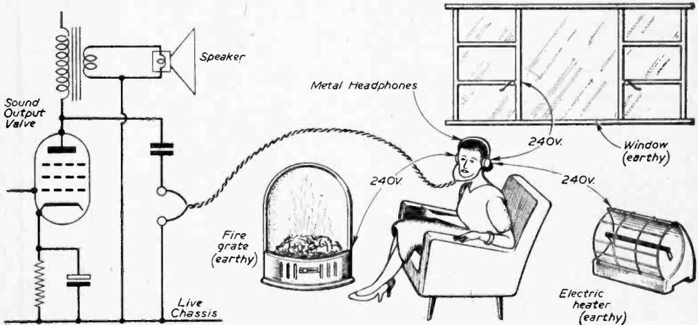
Fig. 1.—The dangers of connecting headphones direct to a live chassis.
