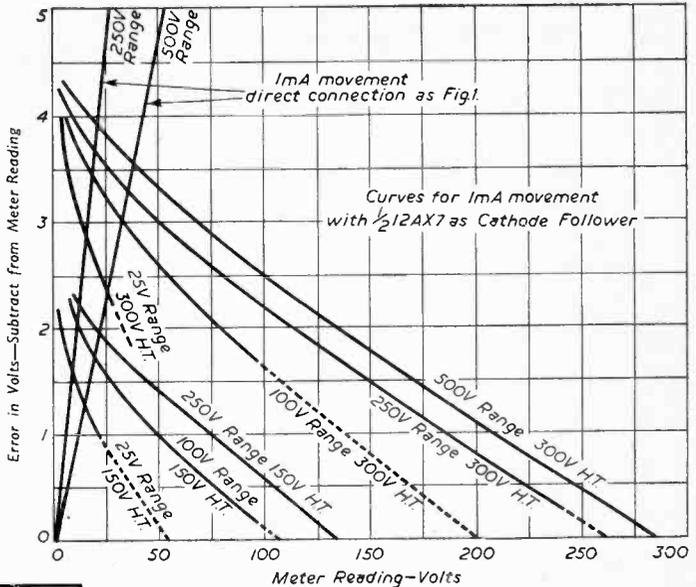
Fig. 3.—Error curves corresponding to the connections in Figs. 1 and 2.
