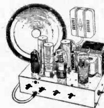
A.C. mains 200-250 v. Size 10in. x 6in. x 2in. Incorporating 6 valves, H.F. pen., 2 triodes, 2 output pens and rectifier. For use with all makes and type of pick-up and mike. Negative feedback. Two inputs, mike and gram., and controls for same. Separate controls for Bass and Treble lit. Response flat from 40 cycles to 15 Kcs..
