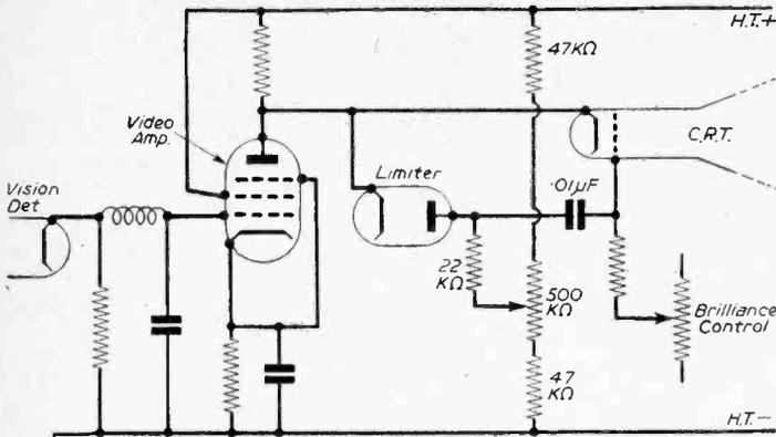
Fig. 4.—Spot inversion type interference limiter.
