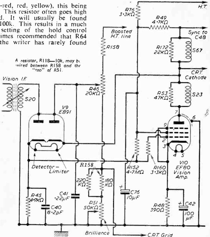
Fig. 3.—Video detector and amplifier stages.
