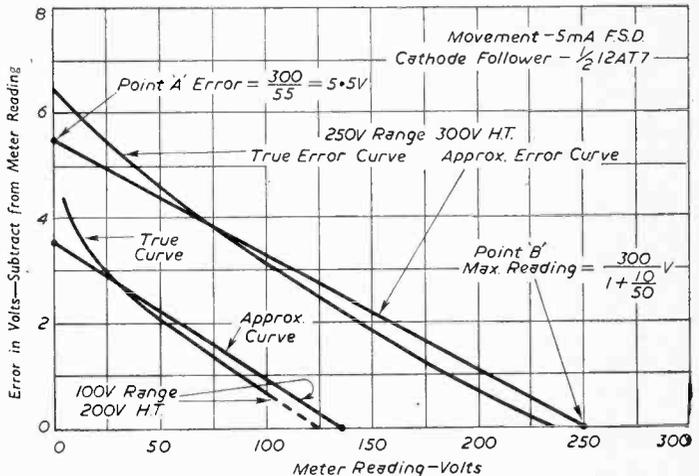
Fig. 5.—Comparison of approximate method and true error.
