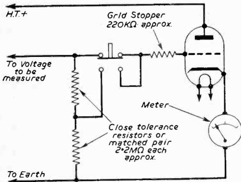
Fig. 4.—A suitable circuit for the cathode follower voltmeter.
