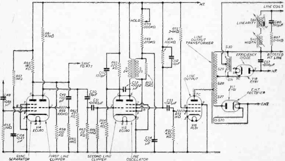
Fig. 1.—Sync separator and line timebase circuits.
