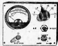
Comprising 2in. moving coil meter scale calibrated in AC/DC volts, ohms and milliamperes. Voltage range AC/DC 0-50, 0-100, 0-250, 0-500. Milliamps 0-10, 0-100. Ohms range 0-10,000. Front panel, range switch, wire-wound pot. (for ohms zero setting), toggle switch, resistor and rectifier. In grey hammer finish case.
