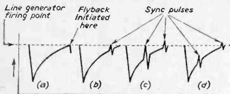
Fig. 3.—Firing points of line generator: (a) free-running, (b) normal synchronised line scan, (c) fired prematurely in the middle of a line scan during the framing period, (d) normal synchronised line scan during the framing period.
