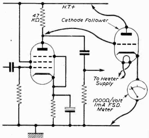
Fig. 2.—Using the cathode follower voltmeter for reading an anode voltage.
