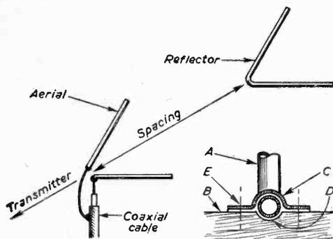
Figs. 2 and 3.—Adding a reflector, and the method of fixing the elements.
