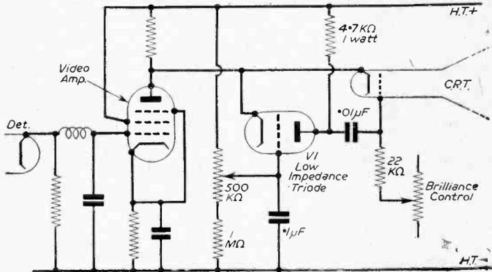
Fig. 5.—"Black spotter" limiter, using extra triode valve.
