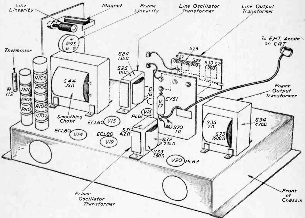
Fig. 6.—The chassis layout.
