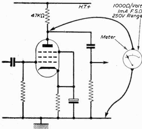
Fig. 1.—Using a conventional meter to read an anode voltage; errors may be introduced if the meter takes a large current.
