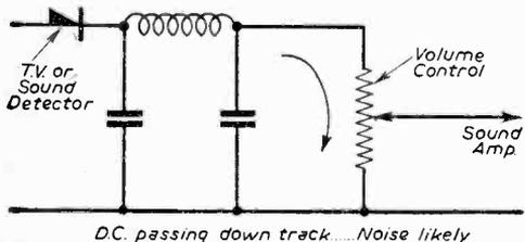
Fig. 3(a).—The usual method of wiring the volume control; D.C. passes through the control.
