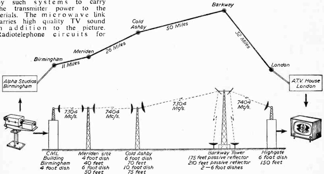
Fig. 1.—A diagram of the route taken by the new TV link.
