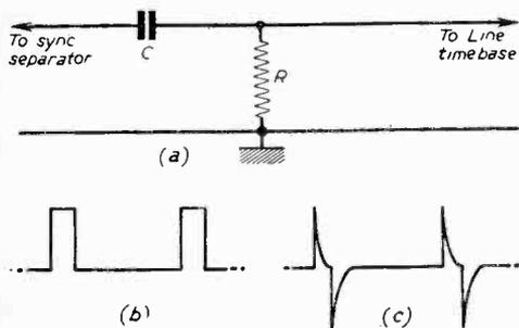
Fig. 1.—A basic differentiator circuit is shown at (a) and line sync pulses at (b), while (c) shows how the pulses are shaped due to the action of (a).
