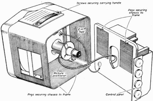
Fig. 3.—A view of model TP\$180 showing how the chassis detaches from the main frame.
