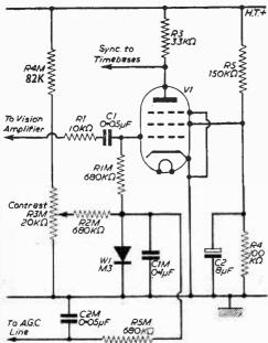
Fig. 4—Obtaining an AGC bias from the sync separator stage and including a manual contrast control.
