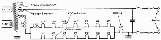
Fig. 2.—A conventional series/parallel arrangement with the small mains transformer which supplies the CRT heater voltage also used as a voltage selector ballast. "Cold" meter checks on one chain are easier if one valve from the opposite chain is removed (Ekco T161).
