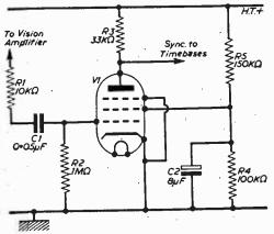
Fig. 3-Typical sync separator circuit.
