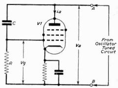
Fig. 2-A reactance valve sweep circuit.
