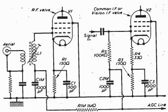
Fig. 2—Eliminating the contrast control from Fig. 1 and rearranging the circuit for an AGC line.
