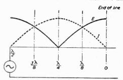
Fig. 14.—Voltage and current distribution at the end of an open-ended line.
