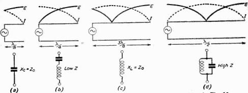
Fig. 16.—Compare these curves, of a short-circuited line, with those in Fig. 15.
