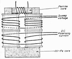
Fig. 3-A ferrite modulator.
