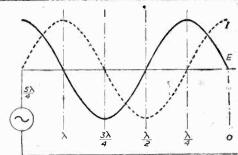
Fig. 13.—Reflected voltage and current from short-circuited line.
