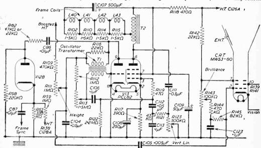
Fig. 3.—The frame timebase and C.R.T. circuit.
