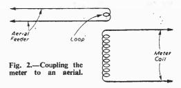
diameter should usually serve for about 45 to 90Mc/s, with a 2½-turn coil for 70 to 150Mc/s, and a 1-turn coil for up to about 250Mc/s. With the very small coils, extremely short wiring is essential, as mentioned, or the valve will cease to oscillate.
