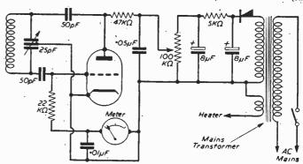
Fig. 1.—The circuit diagram of the grid dip meter.
