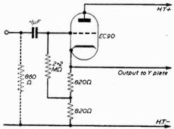
Fig 2.—Output circuit to oscilloscope.
