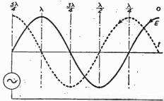
Reflected voltage and current from open circuited line Note: Current and voltage waves shown in one line only for clarity
