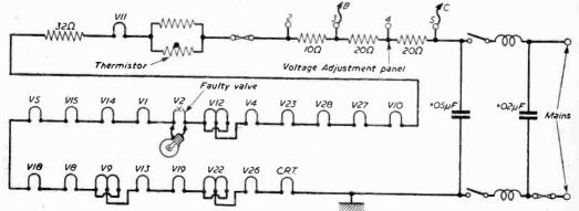
Fig. 1.—Typical example of a 0.3A heater chain (Pye V4).
