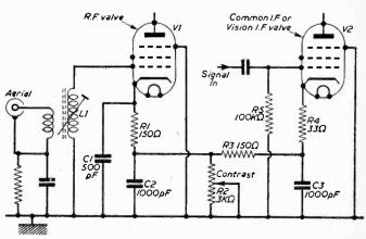
Fig. 1-Typical contrast control circuit.
