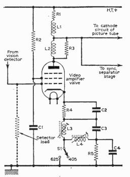
Fig. 27-Video amplifier stage used in some switchable receivers. On 405 lines the stage is biased for the positive signal drive by the voltage dropped across R4 and R5 in series, but on 625 lines the bias is reduced to cater for the negative signal drive by switch SI short-circuiting R5.
