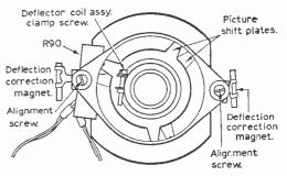
Fig. 8(c)—Picture adjustments provided on some Bush receivers.
