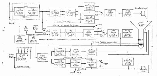
Fig. I—Block diagram of the new Pye switchable Model V700D. Note that the stage references here correspond to those on the circuit sections.
