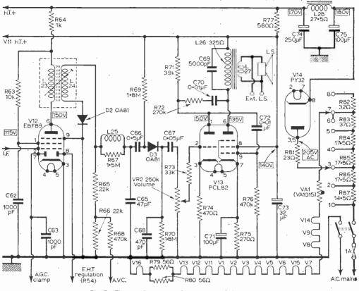
Fig. 5—The sound section and the power supply circuitry.
