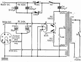
Fig. 2 (above)—An improved version of the basic arrangement, using full-wave rectification.
