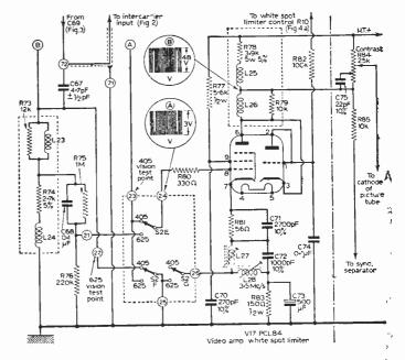
Fig. 5—Showing the vision detector "reversal" switching and the video amplifier stage. Note that the triode section of VI7 is used as the white spot limiter valve on 405 lines only. Points A and B correspond with those similarly identified in Fig. 4,
