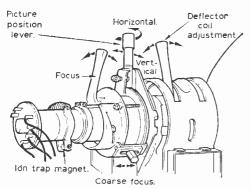
Fig. 8(a)—Sketch showing picture adjustments provided on some Ferguson models.
