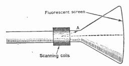
Fig. 5-Corner cutting often occurs due to the electron beam striking the neck of the tube when the scanning coils are removed from the flare of the tubealso see Fig. 6.
