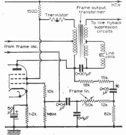
Fig. 55—The basic frame amplifier circuit of the K-B New Queen Special, Model OV30. In the event of limited picture height, the capacitor marked thus\* can be reduced from  $0.05\mu$  to  $0.025\mu$  (see text). down to about  $0.025\mu$ F, but in most cases it will be found that a value of  $0.04\mu$ F gives a good compromise of height and linearity in relation to the controls (see Fig. 55).
