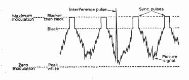
Fig. 36—Showing how an interference pulse appears on a negatively-modulated television signal. Note that the pulse rises in the direction of the sync pulses.
