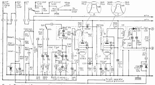
Fig. 4—The vision i.f. stages and vision detector circuit and the tuner switching arrangements. The i.f. stages are designed for the required 625-line passband and filters are switched into circuit to restrict the passband on 405 lines. The "distant", "intermediate" and "local" tappings alter the delay of diode VI3.
