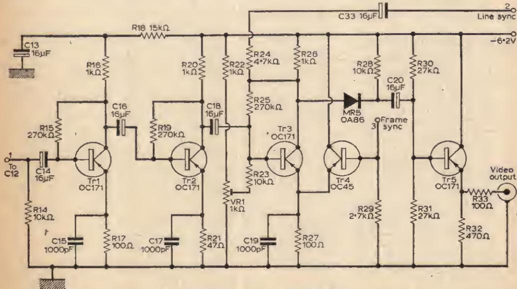
Fig. 2—The video amplifier circuit.
