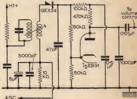
Fig. 15—Decca DM4, etc., detector and noise limiter, using both thermionic valve and semiconductor diode.
