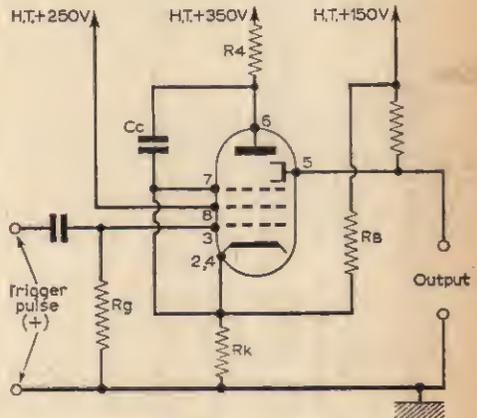
Fig. 4—A simplified representation of the EFP60 stage of the circuit.
