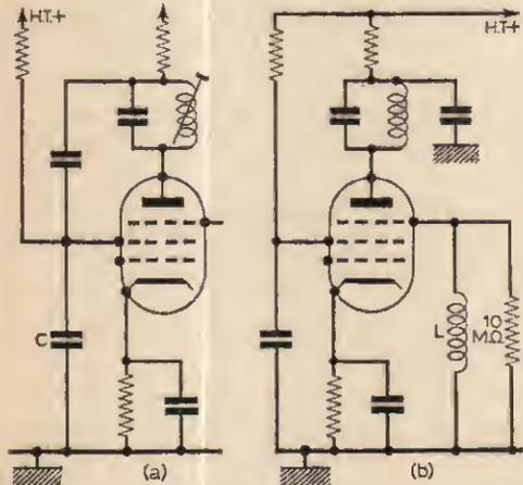
Principal fault with the older models was deterioration of the high value load resistor, or the resistor from h.t. which provided bias. An example is the HMV 1918, where the EB91 has a 3.9MΩ anode load, which can increase to 10MΩ and cause distortion and intermittent sound breakthrough. Loads on TV sound detectors tend to be lower than on radio receivers, with smaller reservoir capacitors, because of the higher frequency i.f.
