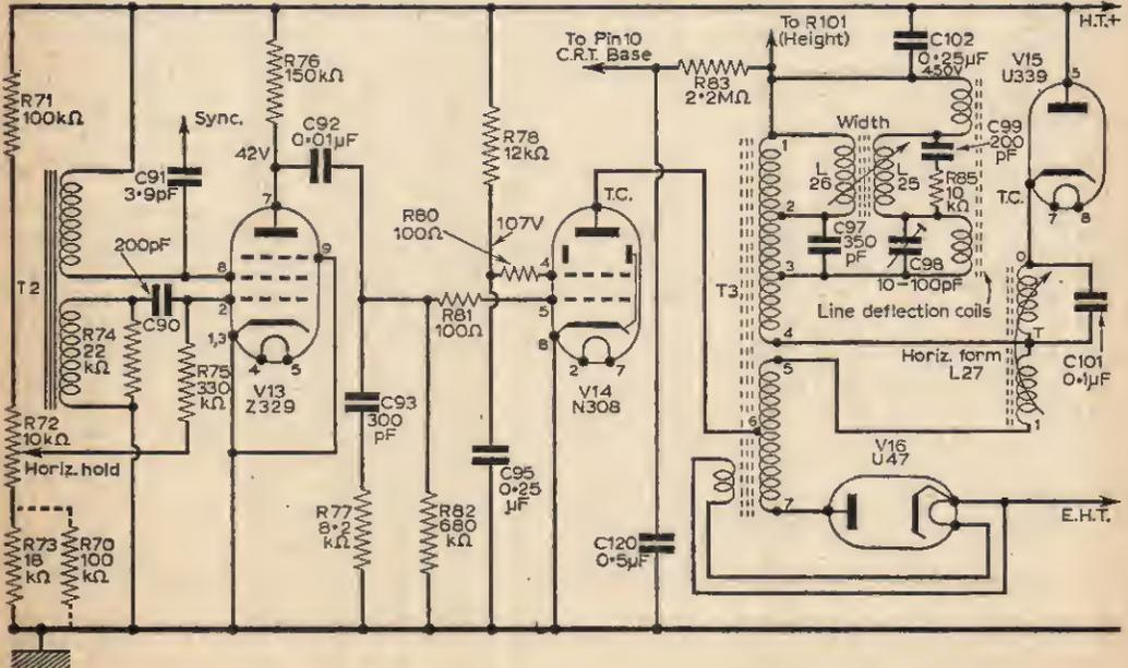
Fig. 4a—The line timebase section of the circuit.
