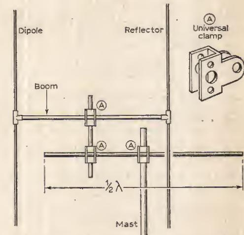
Fig. 1—The simple construction of an aerial recommended by the author of this article.
