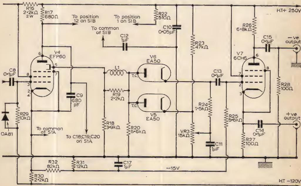
It will be seen that because of the delay line in the cathode circuit of V3b the output pulse from V7 is delayed with respect to the sync pulse from the cathode circuit of V3a. Thus, if the latter is used to trigger an oscilloscope time-base, the leading edge of the output pulse will always be visible providing the time-base generator is running at an appropriate speed. The actual delay may be altered from zero to  $1\mu\text{S}$ , so providing for most practical contingencies.
