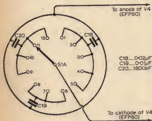
Fig. 2a (above)—Wiring details of S1A.
