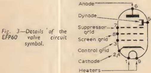
Fig. 3—Details of the EFP60 valve circuit symbol.
