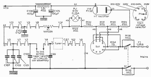
Fig. 4-The power supply and heater circuits.
