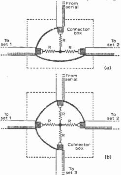
Fig. 2—Connections to more than one set from a common aerial system should always be made through resistors, as shown at (a) for two outlets and at (b) for three outlets. The value for R can be found by a simple calculation as detailed in the text.
