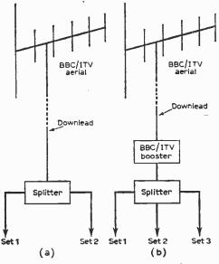
Fig. 3—Where the aerial signals are strong, the simple arrangement at (a) is suitable for two outlets, but where the signals are weak or if more than two outlets are required the boosted arrangement at (b) should be used.
