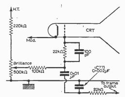
Fig. 42—Marconi method of frame flyback suppression.
