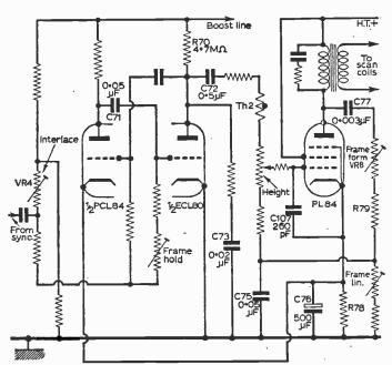
Fig. 39—Decca frame circuit. Note the interacting hold and interlace controls, the series feedback circuitry and the oscillator h.t. feed from the boost line.
