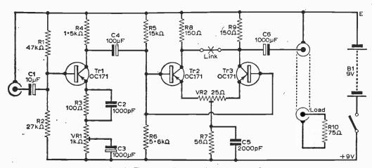
Fig. 4—The circuit of a vision distribution amplifier.
