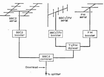
Fig. 7—BBC-2 signals nearly always require separate amplification before combining, as shown here.
