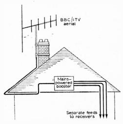
Fig. 4—The mains-powered signal booster can be housed in the roof space. Continuous powering is feasible, for the consumption is very small, amounting to a few pence of electricity per year.
