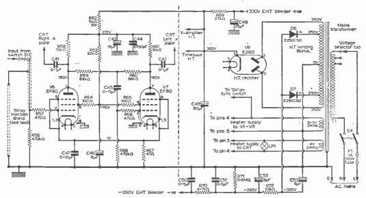
ig. 4—X-amplifier and the power supplies. Conventional components are used in the power supply, and the X-amplifier can be used with an external signal or with the built-in timebase of Fig. 2 (last month). To avoid h.t. surges, V8 may not be replaced by a metal rectifier.
