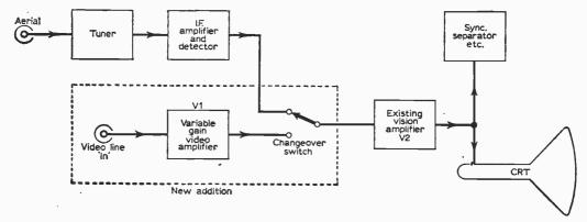
Fig. 1—A simplified block diagram of a television receiver, indicating the additional sections.
