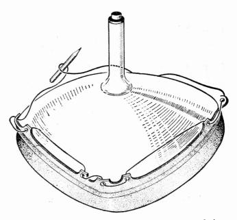
Fig. 3-Refitting the Cornehl safety hood to the latest type of tube.
