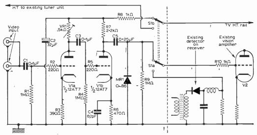
Fig. 2—The circuit modification. The circuitry to the right of the dotted line belongs to the existing receiver.
