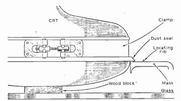
Fig. 1—Tube replacement diagram for the 17TG100U. The wood block fitted to ensure correct spacing between the c.r.t. and the glass should be 7mm thick.
