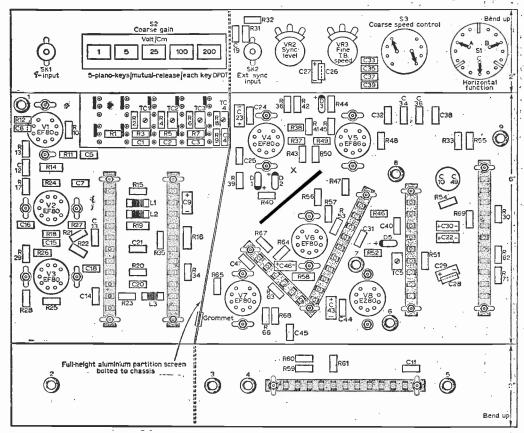
Fig. 6—Sub-chassis layout. The screen is essential to prevent blockage of the sensitive Y-amplifier by timebase transient injection.
