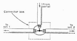
Fig. 1—Coaxial cables should never be connected in this way. This results in mismatch, standing waves and signal reflections.
