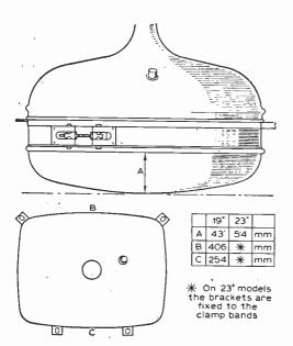
Fig. 2-Gritical measurements to be observed with the 19TGIIIA series.
