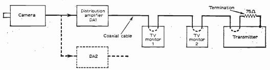
Fig. 5—An amateur television station set-up including a distribution amplifier (DA).
