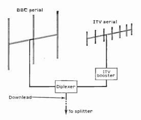
Fig. 5—If only one signal is weak, just one channel boost can be given, as this drawing shows.
