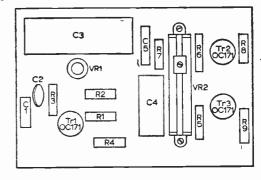
Fig. 6—A suggested layout for the distribution amplifier, for either printed circuit or conventional wiring.
