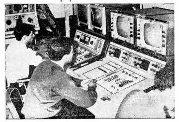
THIS photograph shows presentation switching equipment made and supplied by EMI Electronics Ltd., in service at the Wellington studios of the New Zealand Broadcasting Cor-
