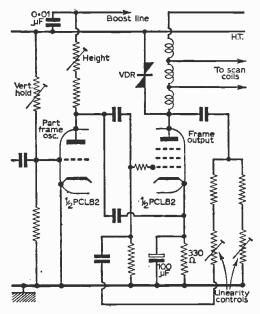
Fig. 40—Ferguson frame circuit. A typical feature is the provision of separate h.t. feeds and the VDR across the output transformer.
