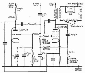
Fig. 41—Ultra frame circuit. A single linearity control is employed and thermistors are fitted in the output transformer secondary circuit to damp flyback pulses and compensate for changing characteristics with heat
