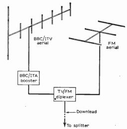
Fig. 6—Here is shown how f.m. is added to a master aerial system. If the f.m. signal is weak, a boost can be supplied with a separate f.m. booster.
