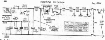
Fig. 2—Triple output h.t. smoothing and supply system used in many GEC/Sobell v.h.f./u.h.f./f.m. receivers. Note valtage variations on 625, 405 and f.m. and additional surge limiter in circuit on f.m. to reduce voltage.
