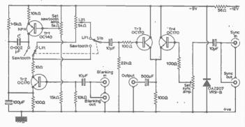
Fig. 4---Test waveform generator supplying sawtooth or variable lift waveform.
