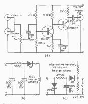
Fig. 8.—(a) Transistor video amplifier (b) D.C. power supply from parallel heater chain and (c) series heater chain.
