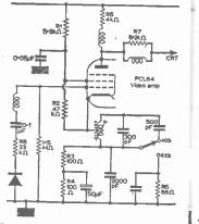
Fig. 1—Basic Ferguson dual-standard video amplifier. When RI and R2 reduced in volue thus increasing voltage drop across R3 and R4 and over-biassed the video amplifier, symptoms were (a) practically zero sync lock, (b) low a.g.c. voltage, (c) i, overloading and (d) poor picture towal gradation,
