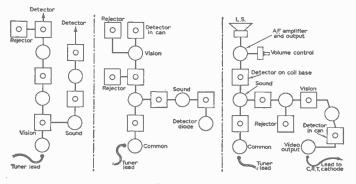
Fig. 1-Various i.f. layouts showing how sound and vision chains can be traced.
