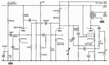
Fig. 3—Variation on the theme of Fig. 1, used in a wide range of Thorn receivers, under the Ferguson, Marconi, H.M.Y and Ultra trade marks. Differences are discussed in the text.
