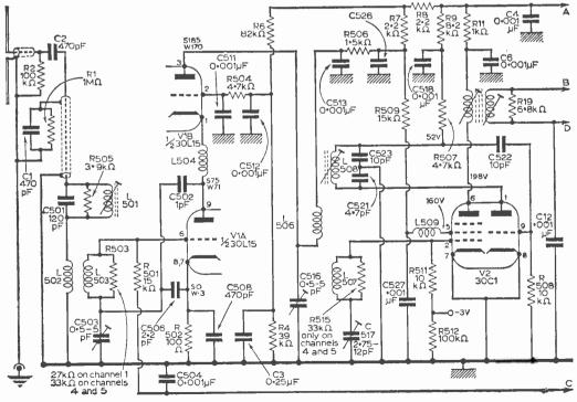
Fig. 1: Tuner circuit of the V470.
