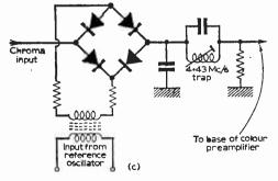
Fig. 7c: Semiconductor bridge demodulator.
