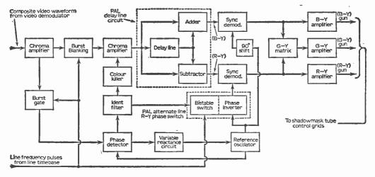
Fig. 1: Block schematic diagram of the essential features of a PAL decoder.
