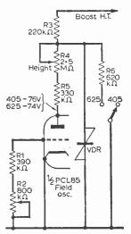
Fig. 1: Height stabilising circuit used in Ferguson/ HMV/Ultra 16in. range of portables.
