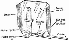
Fig. 49: System switches are often cable-operated. In some types it is important that the removal of the cable is by unhooking the clamp and releasing the nipple, but not loosening the retaining screw.
