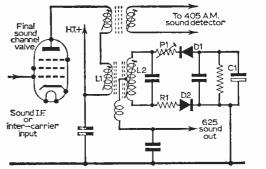
Fig. 6: Intercarrier buzz can often be reduced by carefully balancing the f.m. ratio detector by adjustment of P1.
