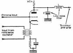
Fig. 7e: A simple synchronous demodulator elicuit using a triode valva. A low-pass filter and subcarrier releator are included in the output circuit.
