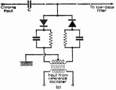
Fig. 7b: Synchronous demodulator using two diedes.
