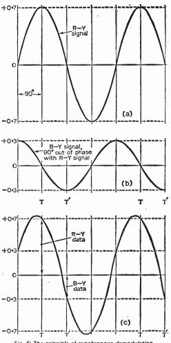
Fig. 6: The principle of synchronous demodulation.
