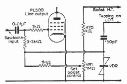
Fig. 3: GEC/Sobell/McMichael width stabilisation system. Correct picture width is obtained by setting VR1 "Set Booster Control" to give boost rail voltage of between 750–790V with full rester scan.
