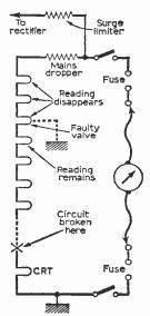
Fig. 1: Testing for heater/ cathoda leaks with an ohmmeter.
