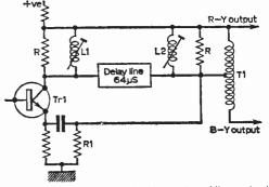
Fig. 5: Technique suggested by Mullard for adding and subtracting in conjunction with their DL1 de'ay line to provide separate R-Y and B-Y outputs (simplified circuit).
