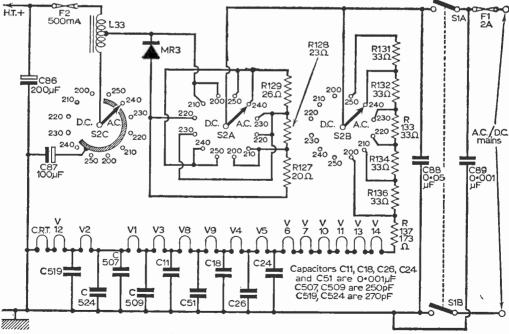
Fig. 3: Power supply circuitry for the V470 chassis.
