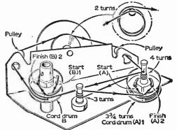
Fig. 50: An example of the fine tuner system employed for u.h.f. tuning. Exact routing of cord and freedom of pulleys in very important to avoid backlash and tuning drift.
