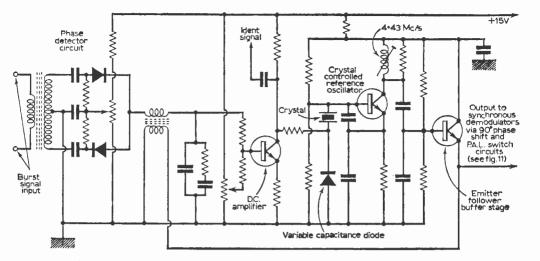
Fig. 11 (above): Simplified circuit of a crystal reference oscillator with phase detector and control circuits. Fig. 12 (below): PAL switch, using a bistable switch circuit and pair of switching diodes to reverse the phase of the reference signal to the R - Y synchronous demodulator on alternate lines.
