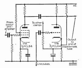
Fig. 10: Pentode colour output stage with triode clamp to clamp the output during the line flyback period to the correct zero value.
