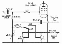
Fig. 2: Width stabilisation circuit used in many Dynatron models incorporating separate width setting potentiometers for both systems.
