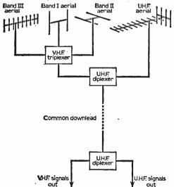
Fig. 2: While the existing v.h.f. downlead can also be arranged to carry the u.h.f. signal by the use of top and bottom u.h.f. diplexers. as shown, this technique should be avoided in areas of weak signal or where picture grain is troublesome.
