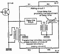
Fig. 4: Practical aspects of a PAL delay line circuit.
