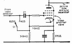
Fig. 4: Grid current in the video amplifier value can affect the picture locking on 625-lines owing to the a.c. coupling on this standard. The relatively low grid impedance on 405-lines, due to the d.c. coupling on this standard, can often mask grid current effects (see text).
