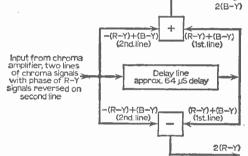
Fig. 2 (above): How the delay line circuit separates the B - Y and R - Y signals and carries out averaging over successive pairs of lines.
