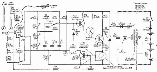
Fig. 1: Theoretical circuit diagram of the transistorised e.h.t. meter.
