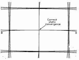
Fig. 5: Typical dynamic convergence errors.
