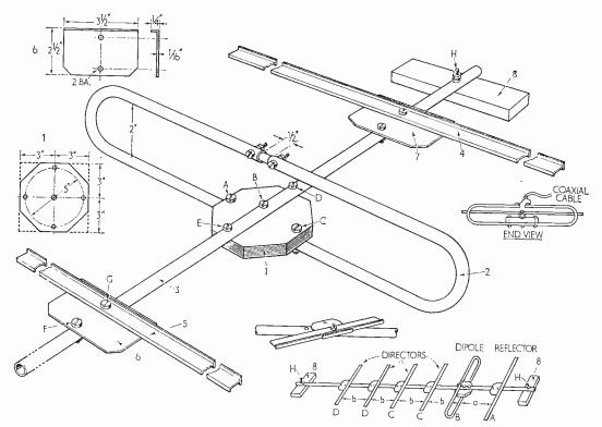
Fig. 1: Full constructional details of the Band III loft aerial.
