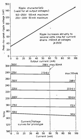
Fig. 7: Performance of the H.T.2 150-300V output. Procedure for presetting the output from this circuit is as follows. With zero output current drain (open-circuit) alternately adjust VR4 for 155V output and VR6 for 300V output between P5 and P7, with VR5 respectively at its left- and right-hand stops. Final adjustment is VR6 for 300V output with VR5 at its righthand stop. Then calibrate scale of VR5 with respect to output voltage readings at intermediate settings.
