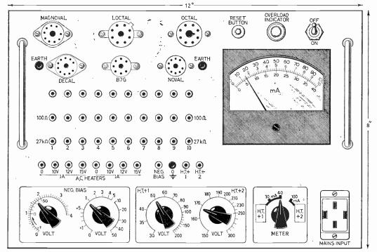
Fig. 8: Front panel layout. The front panel and chassis form an integrated drawer unit which pushes into the  $6\frac{1}{2}$  in -deep cabinet.
