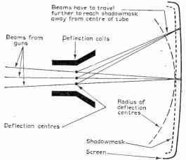
Fig. 2: The basic reason why dynamic convergence is necessary is because the geometry of the shadowmask and screen differs from the radius of the beam deflection centres.
