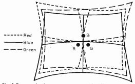
Fig. 4: Because the three guns are mounted in different positions relative to the axis of the tube the three rasters they trace out are of different shape.
