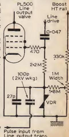
Fig. 1: Line output valve grid circuit.
