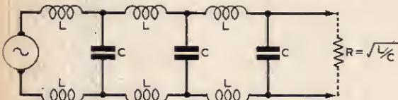
Fig. 4: Equivalent circuit of a transmission line.
