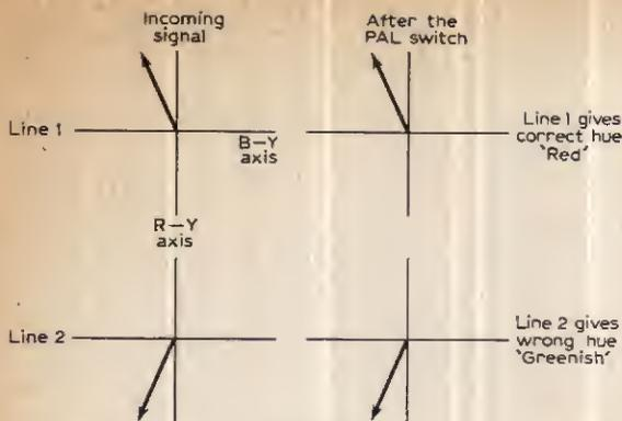
Alternate lines of a field are Red and Green in this example
