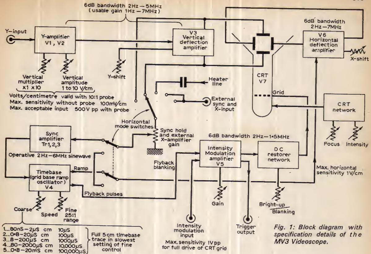
Fig. 1: Block diagram with specification details of the MV3 Videoscope.
