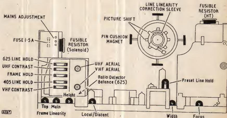
Fig. 1: Rear chassis view, showing preset adjustments.
