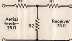
Fig. 7: Simple T-network attenuator.
