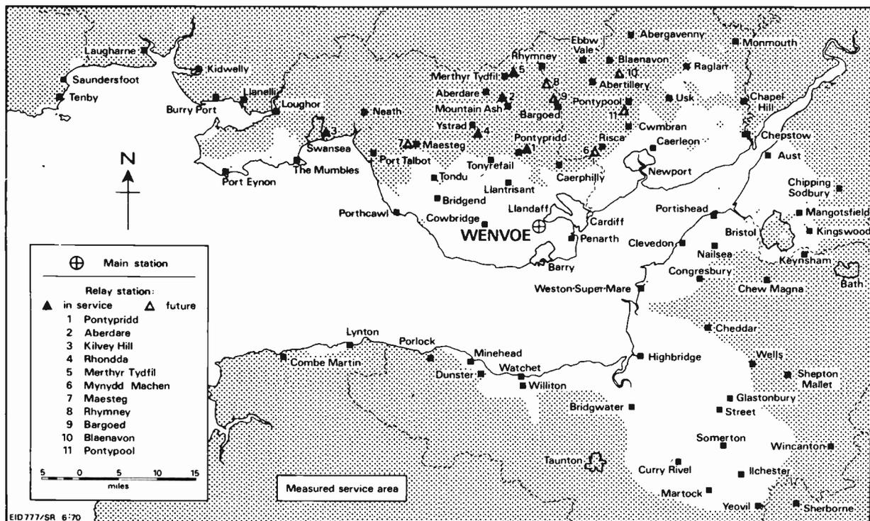
The above BBC map shows the approximate service area of the Wenvoe u.h.f. transmitter (maximum vision e.r.p. 500kW). Small pockets of poor reception too small to be shown in this map may be experienced. Channels: ITA 41; BBC Wales 44 BBC-2 51. Polarisation horizontal, receiving aerial group B.
