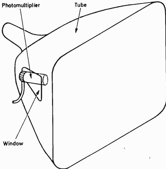
Fig. 7: Principle of ultra-violet indexing.
