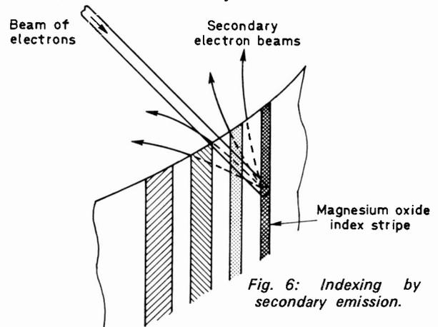
Fig. 6: Indexing by secondary emission.
