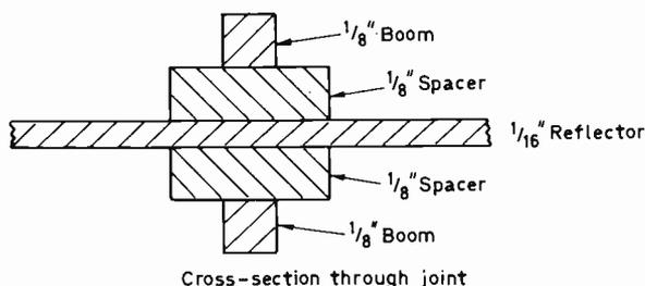
Fig. 2: Reflector assembly.
