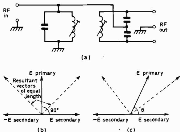
Fig. 3: (a) R.F. equivalent circuit of the ratio detector tuned circuits. (b) Relationship of voltages at resonance. (c) When the sound carrier frequency deviates the 90° phase relationship of (b) no longer applies and the resultant vectors are of unequal length: one detector diode therefore conducts more heavily than the other.
