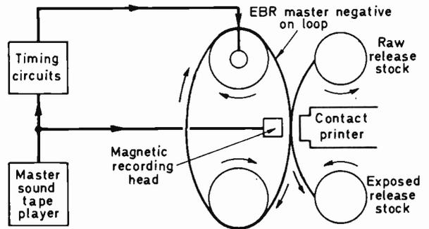
Fig. 3: High-speed EVR printer arrangement.
