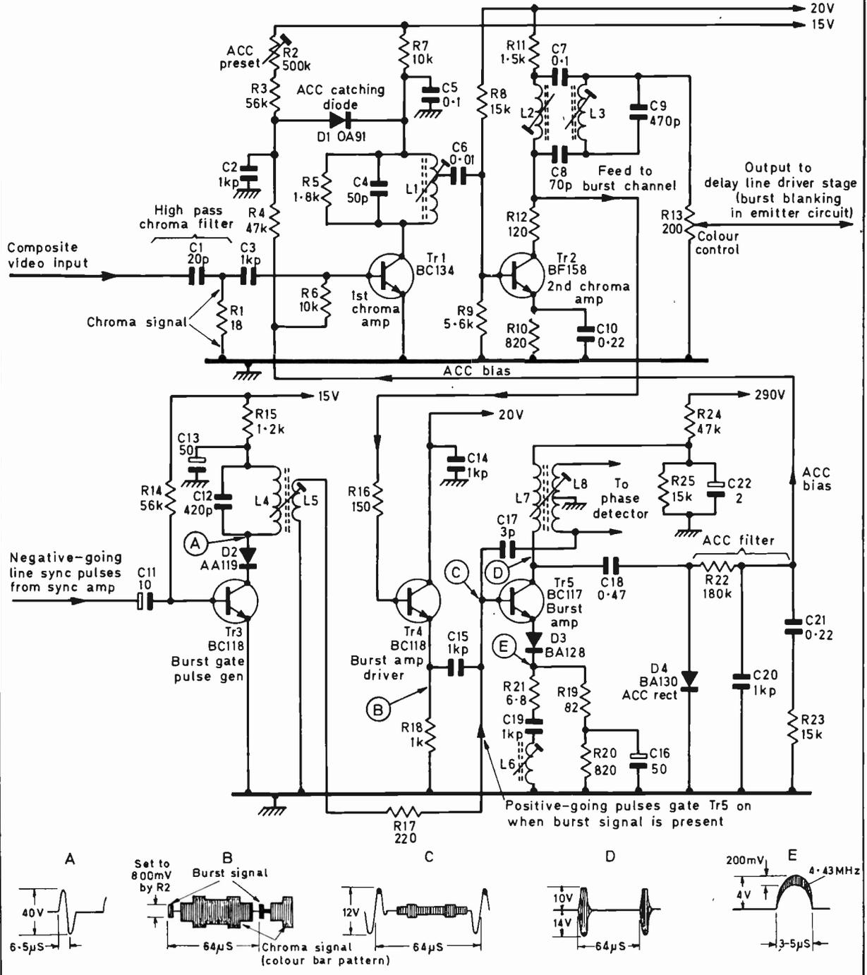
is in these models undertaken in the colour-difference preamplifier stages. Secondly instead of burst blanking—removing the burst signal from the chroma signal—being undertaken in the chroma circuits it is undertaken in the following delay line driver stage—by feeding positive-going pulses to its emitter so that it is switched off during the burst signal period. (the delay line driver, being an npn transistor, will be
