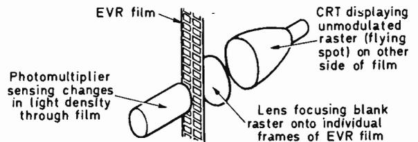
Fig. 4: Principle of flying-spot scanning.
