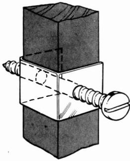
Fig. 1 (left): Back screw with cabinet clip, as described in the text.
