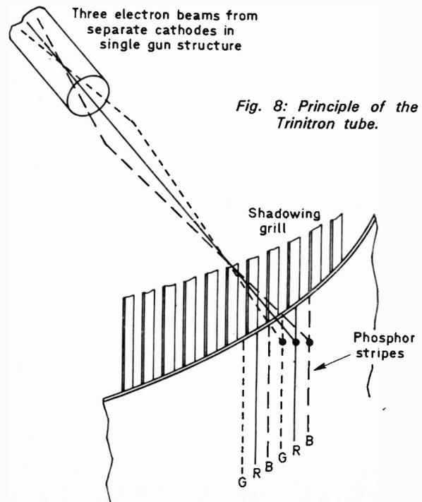
Fig. 8: Principle of the Trinitron tube.
