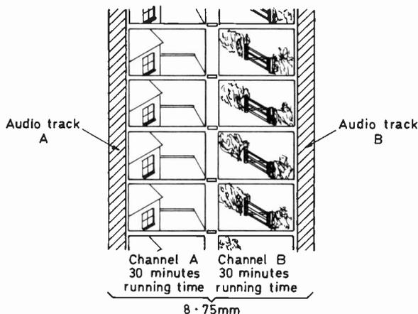
Fig. 1: Layout of monochrome EVR film. A one-hour cartridge has some 180,000 frames each of which can be studied individually.
