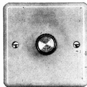
This is an attractive unit which fits in place of the normal modern light switch. The ivory mounting plate matches modern fittings and the control knob is bright chrome. An ON/OFF switch is incorporated to control 40-600 watts of all lights except fluorescent at mains voltages from 200-250V, 50 Hz.
