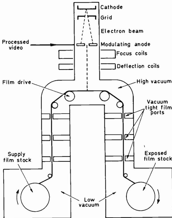
Fig. 2: Electron-beam recorder.
