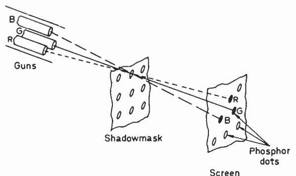
Fig. 1: Schematic of the shadowmask tube. The spacings have been distorted for clarity. In reality the guns are some 10-12in. from the screen, the shadowmask is about  $\frac{1}{2}$  in. from the screen, and the electron beams cover about three holes in the mask.
