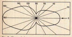
Fig. 5: Wrong design can cause a yagi to "back-fire" at certain frequencies within the bandwidth with a resulting impairment to the front-to-back ratio.
