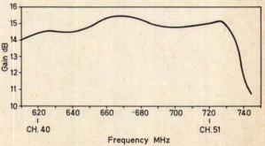
Fig. 7: Gain-bandwidth characteristic of the J-Beam Multibeam MBM38 array.
