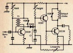
Fig. 3: Practical field timebase circuit using a blocking oscillator stage. Note the tapping on T1 primary, explained in the text.
