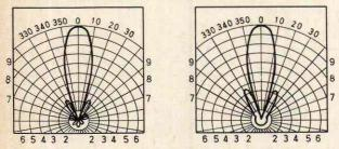
Fig. 1 (left): Horizontal polar diagram of 18-element yagi (including reflector system). This has a front-to-back ratio of about 26dB.
