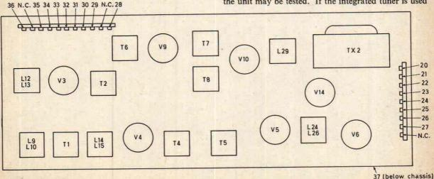
Fig. 1: Top layout of the panel, showing the tag connections.
