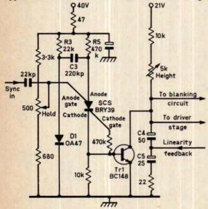
Fig. 6: Field oscillator stage using a new component, the silicon controlled switch, to provide the switching action required to discharge the scan charging capacitors C4 and C5 via Tr1 at the end of the scan period.
