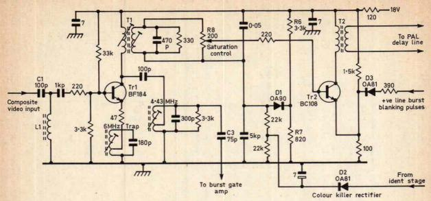
Fig. 3: Decca chroma amplifier circuit with burst blanking at Tr2 emitter.
