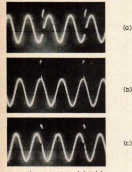
Increasing gate delay (a)  $\rightarrow$  (c) In each case the chunk chopped out of signal by gate is magnified alone over full screen in strobe operation as typically shown in G (b)
