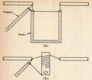
Fig. 4: Development of the J-Beam inverse balun: (a) shows the basic matching stub principle which gives a 75-ohm coax feed from the relatively higher terminal impedance of a skeleton slot radiator while (b) shows how J-Beam simulate the principle by means of a wound component.
