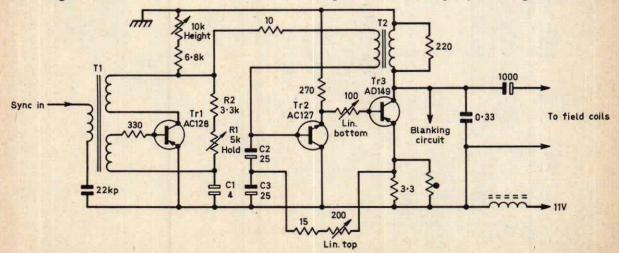
Fig. 4: A further practical blocking oscillator example, as used in the Philips portable T-Vette.
