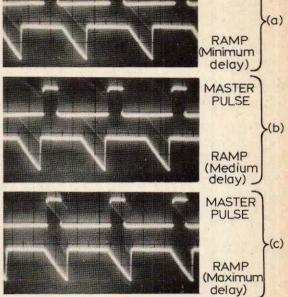
sive sync lock ranges overlap and an unlocked state is no longer possible. As the relative frequencies are changed cycles add or subtract abruptly without lock ever being lost. This automatic synchronisation persists up to signal repetition frequencies in the MHz range.
