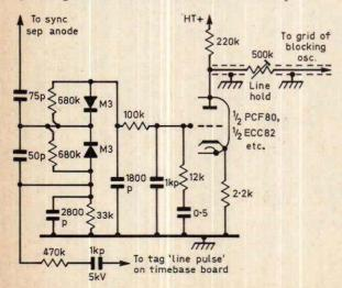
Fig. 8: Flywheel sync circuit for use with Thorn blocking oscillators (from Thorn 850 chassis). Diodes type M3 or similar.
