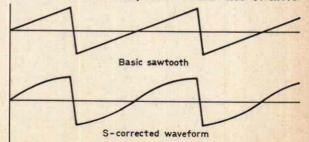
Fig. 7: Illustrating S-correction of line scanning.
