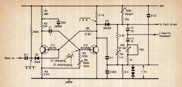
Fig. 5: The first transistorised multivibrator timebase oscillator stage to be used in the UK, from the BRC 3000 single-standard colour chassis.
