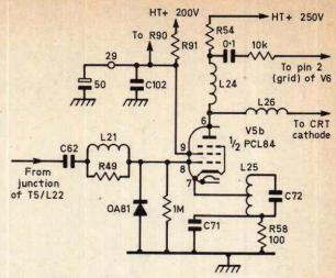
Fig. 5: Modified video amplifier circuit.
