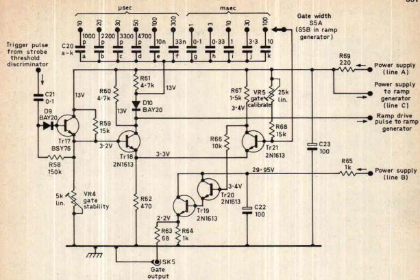
Fig. 5: Circuit diagram of the strobe gate generator. Voltages were measured with the master multivibrator off, gate width 100mS, gate delay maximum, zero sync and in the trigger setting, using a valve voltmeter.
