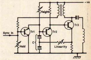
Fig. 2: Self-oscillating timebase circuit in which the flyback pulse caused by the collapse of the field around the deflection coils at the end of the scan is applied to the oscillator via a winding linked to the output inductor and drives the oscillator Tr1 hard on to discharge the scan charging capacitors. Note the introduction of a linearity feedback loop.
