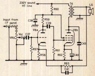
Fig. 8: The audio amplifier and output stages.
