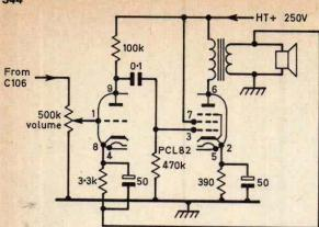
Fig. 3: Suggested audio amplifier circuit.
