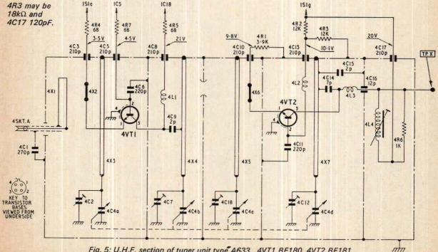
Fig. 5: U.H.F. section of tuner unit type A633. 4VT1 BF180, 4VT2 BF181.
