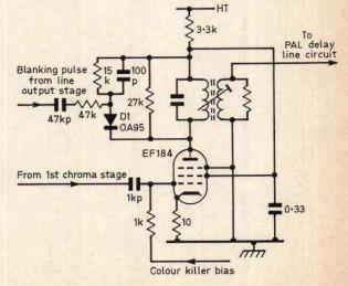
Fig. 1: Second chroma stage in the Philips G6 colour chassis, showing the burst-blanking system.
