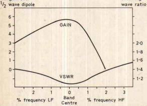
Fig. 3: The degree of mismatch over the bandwidth can be expressed as volts-standing-wave-ratio (VSWR in the diagram). The smaller the ratio the better the matching. The diagram shows that at band-centre the matching is almost perfect while either side of resonance it falls. A wideband aerial is designed to minimize the increase in VSWR over the entire channel group.
