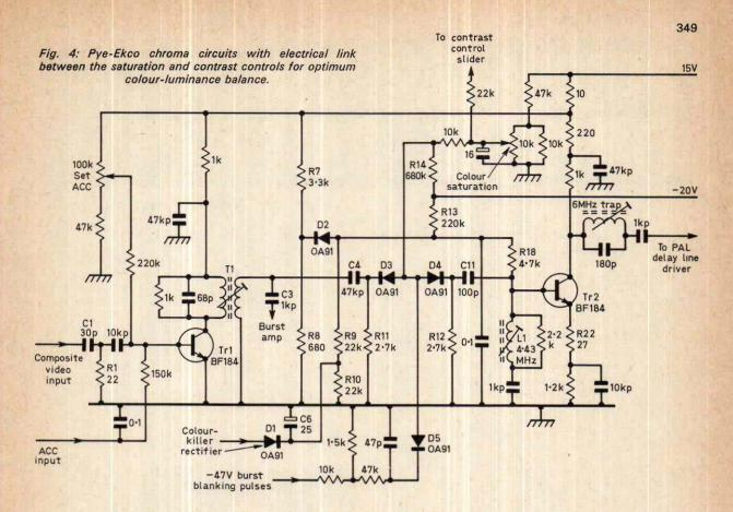
potentiometer with R12 as the lower section. Being arranged back-to-back in this manner the nonlinearity of the diodes, which would otherwise be especially evident at low-signal levels, is cancelled out.
