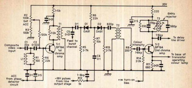
Fig. 2: Chroma amplifier stages in the GEC dual-standard colour chassis.
