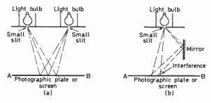
Fig. 6: Interference is seen only when one light beam is split into two sections one of which travels farther than the other. (a) There are no interference effects seen with this set up. (b) With one bulb and one slit, interference effects are seen.
