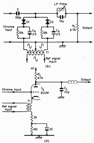
porated in the reference oscillator feed to the B-Y detector in order to achieve the correct 90° phase displacement between the instants of conduction of the two colour-difference synchronous detectors.
