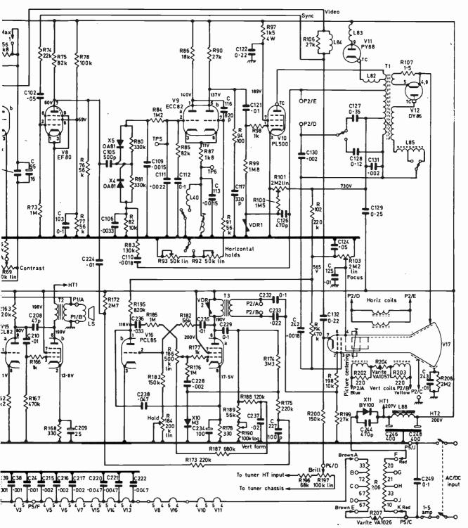
transformer (the v.d.r. will allow a little voltage to appear at pin 6 but not a lot).
