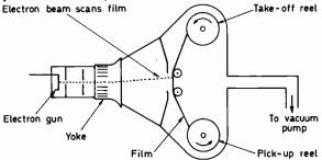
Fig. 8: Basic outline of an electron-beam recorder.
