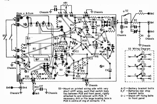
Fig. 4: Layout of the printed board, viewed from the component side.
