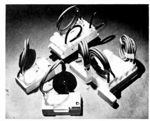
A selection of the replacement e.h.t. rectifier trays available from Clayridge Electronics Ltd.
