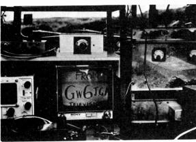
Transmission from GW6JGA/T Prestatyn received portable by GD6FDZ/T on the Isle of Man, path 79 miles.
