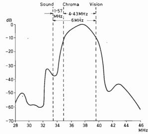
Fig. 2: Typical colour receiver response curve.
