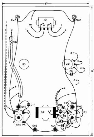
Chassis soldering tag under fixing bolt for coaxial socket PMC Chassis soldering tag under fixing bolt for coaxial socket and printed circuit board
