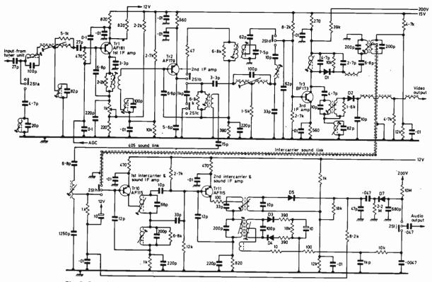
Fig. 3: Sound and vision i.f. circuits and detectors of the Rank-Bush-Murphy CTV25 chassis.
