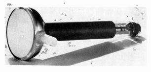
The Brimar Q8-100AA 3in. flying-spot scanner tube developed for use with EVR teleplayers.
