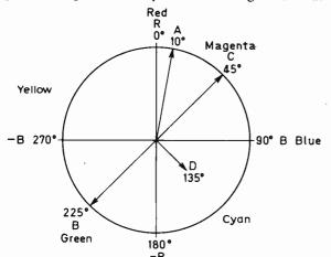
Fig. 3: The "colour clock": the phase of the chroma subcarrier varies to indicate different colours.
