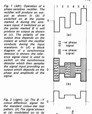
instant, the output then being of the correct amplitude and polarity. For this action to be accurate of course the transmitter subcarrier and receiver reference oscillator must be synchronised and for this purpose the colour burst is transmitted once each line.
