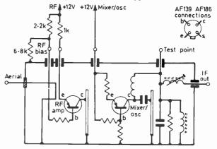
Fig. 2: Basic d.c. and signal paths in a typical "surplus" u.h.f. tuner using germanium transistors. The values of the external resistors are for guidance only and may require slight adjustment for optimum noise performance.
