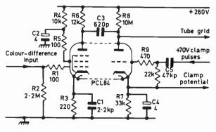
Fig. 1: Pentode colour-difference output stage with triode clamp. With colour-difference drive each shadowmask tube grid is driven by a stage like this.
