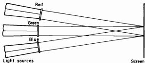
Fig. 4: Additive colour mixing. Sources of red, blue and green light are all directed to the same spot on the screen. The colour seen at this spot on the screen will depend on the proportions of the three primary colours used. Because the lights are added in parallel this is known as additive colour mixing.
