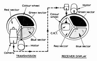
Fig. 6: Principle of early sequential colour systems. The colour wheel was common to all the early sequential colour systems and was the factor which contributed to their downfall. Synchronising difficulties, the high speed of the wheel in line-sequential systems and the non-compatibility doomed such systems to extinction.
