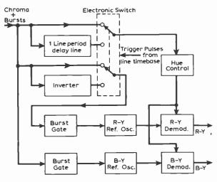
Fig. 1: The chroma signal decoding system used in the Sony Model KV1320.
