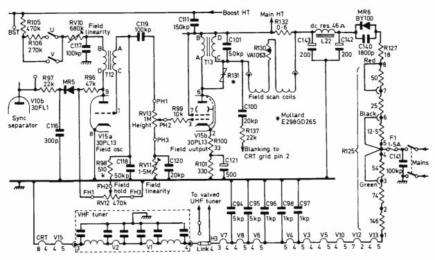
Fig. 2: The field timebase and power supply circuits of the Ekco Model T402. Minor component value variations in the blocking oscillator (V15a) and sync feed circuits may be found in some chassis. C117 charges slowly from the boost rail to give the field timebase waveform. C118, R98 and RV12 control the speed.
