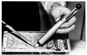
The Picard "Abiko" desoldering gun in use.
