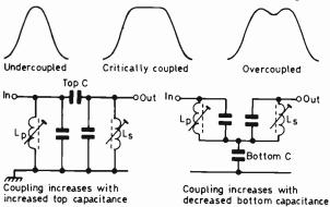
Fig. 4: The three possible bandpass response shapes and two possible types of bandpass circuit.
