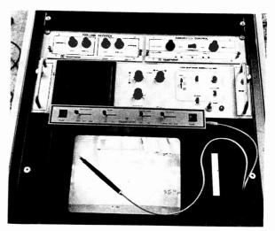
View looking down at the operating surface and the component sections of the Telestrator type TIM-400. The scan converter and converter controls can be remotely mounted if required.
