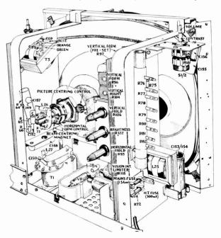
Fig. 1: Rear chassis view. The positions of the tuner and main controls vary from model to model.
