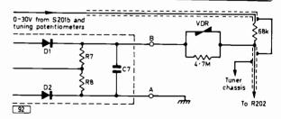
Fig. 8: Correct a.f.c. circuit connections.
