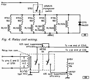
Fig. 5: Suggested switch-off spot suppression circuit. The relay contacts are shown with the receiver switched on, i.e. the relay coil is energised.
