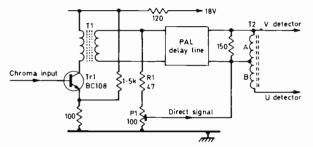
Fig. 3: Representative PAL delay line/matrix circuit. Addition and subtraction are carried out by windings A and B of the centre-tapped transformer T2.
