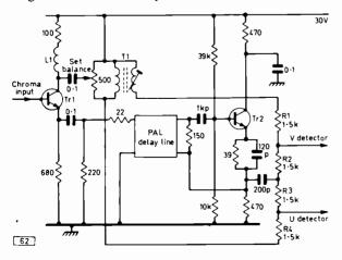
Fig. 7: In this circuit a resistive add and subtract network (R1-R4) is used in conjunction with a post delay line amplifier stage.
