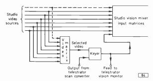
Fig. 4: How the Telestrator output is used with the studio system.
