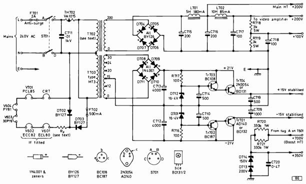
Fig. 2: Power supply circuits. The I.t. and 625-line brightness control feeds are stabilised.
