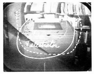
Some of the patterns possible with the Telestrator—solid, dotted and dashed lines—photographed on the face of a monitor. The background shows a podium Telestrator type TIC-100.
