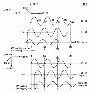
Fig. 6: PAL subcarrier phases shown in both sinewave and vector form.
