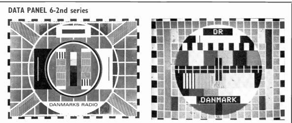
Denmark. Two main Test Cards are used by Danmarks Radio, Test Card G as shown above left and the Philips PM5544. The latter has two versions, one with identification as shown above right and the other not identified but carrying a single vertical white line in the lower black rectangle, or, the left-hand side one tenth of the way in.
