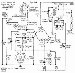
Fig. 1: Suggested field timebase circuit.
