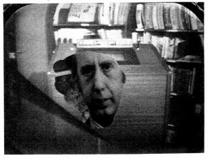
Photograph of monitor face showing an insert key of a second video source. Note the arbitrary shape that can be wiped in, in this case with a medium-strength continuous line.
