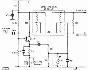
Fig. 6: With more recent types of delay line the summing networks are contained in the delay line housing.
