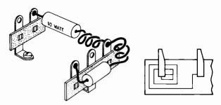
Fig. 1 (left): A replacement silicon rectifier and surge limiter resistor mounted well spaced apart using two tagstrips. The adjacent wire ends have been left long and coiled to minimise heat conduction and maximise heat dissipation.
