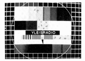
Finland OY Yleisradio. Two test cards are used, the electronic one above including the circle for the TVI network and omitting it for the TV2 network, and also recently on TV2 Test Card G with the identification "Yleisradio TV2".
