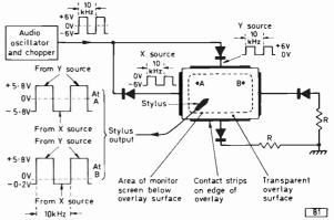
Fig. 1: Telestrator position detector.
