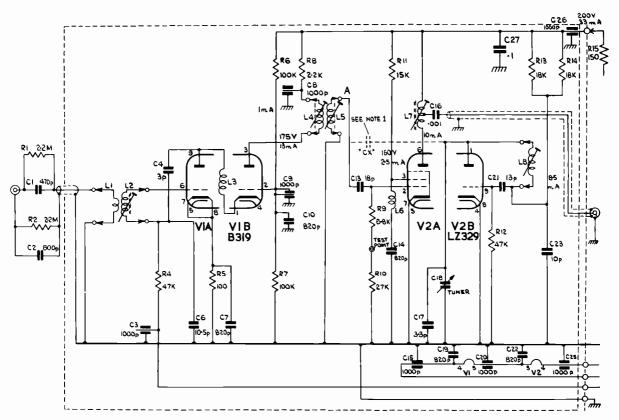
Fig. 3: Circuit of the turret tuner. Note 1: Capacitor CX consists of stray capacitance supplemented on Band III by a loop around L8 connected to point A.
