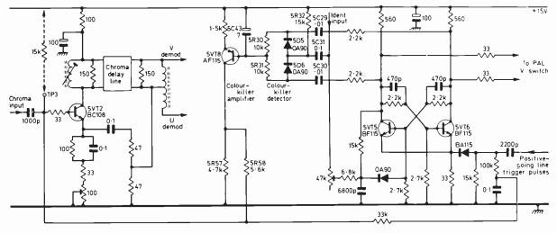
Fig. 1: The colour-killer circuit used in the Bush-Murphy dual-standard colour chassis.
