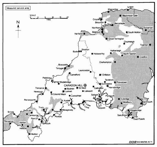
The measured service area of the **Caradon Hill** u.h.f. transmitter is indicated by the unshaded area of the above map. Channels: BBC-1 22, ITA 25, BBC-2 28, fourth 32. Maximum vision e.r.p. 500kW. Polarisation horizontal. Receiving aerial group A. Map courtesy the BBC Engineering Information Service.
