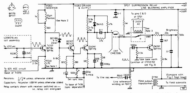
Fig. 6: Video circuit for single-standard (625 lines) operation. Notes: (1) R240 470 $\Omega$  in this circuit. (2) Additional components in Tr207 collector lead. (3) Spot suppression relay—same type as in Fig. 5.
