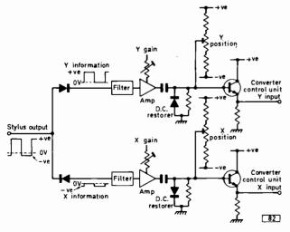
Fig. 2: Position decoder-basic processing of the X and Y position signals.
