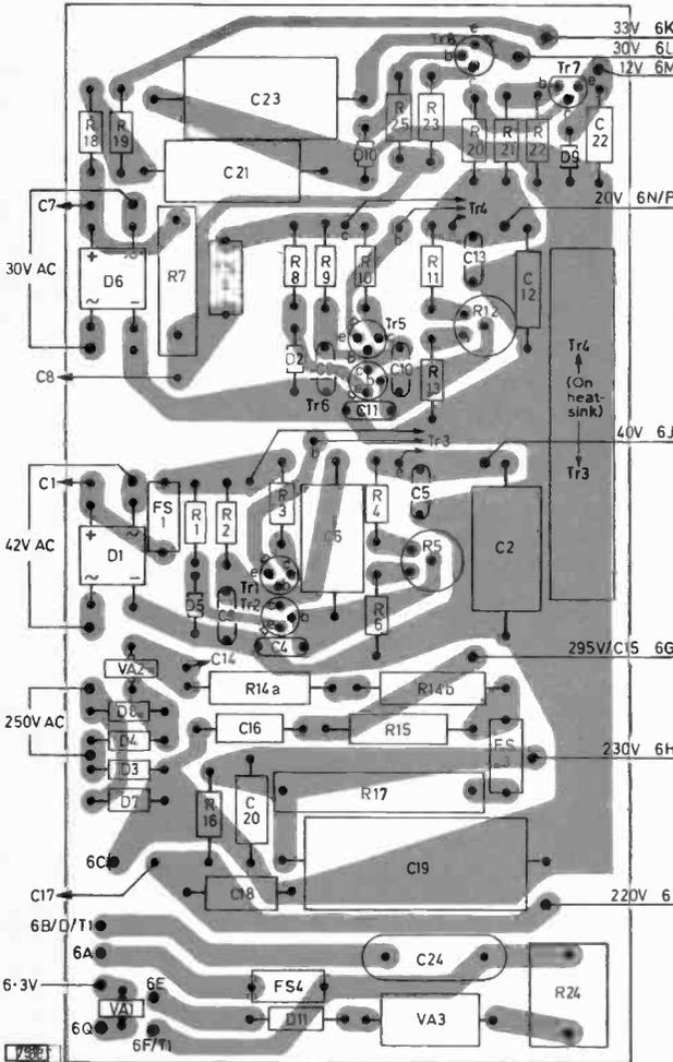
Fig. 6 (left): Layout of E. Erven's power supply, viewed from the component side. C1, C7/8, C14 and C15 are mounted off the board.
