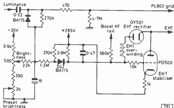
Fig. 3: Beam limiting arrangement used in conjunction with a PD500 e.h.t. stabiliser triode.
