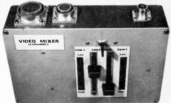
THIS unit is designed for use with any standard video system in which the cameras are synchronised and there is a composite video signal available from at least one camera. The mixer provides fades, dissolves, switch cuts and superimposition and has the possibility of adding an effects unit to permit electronic wipes and split-screen operation.
