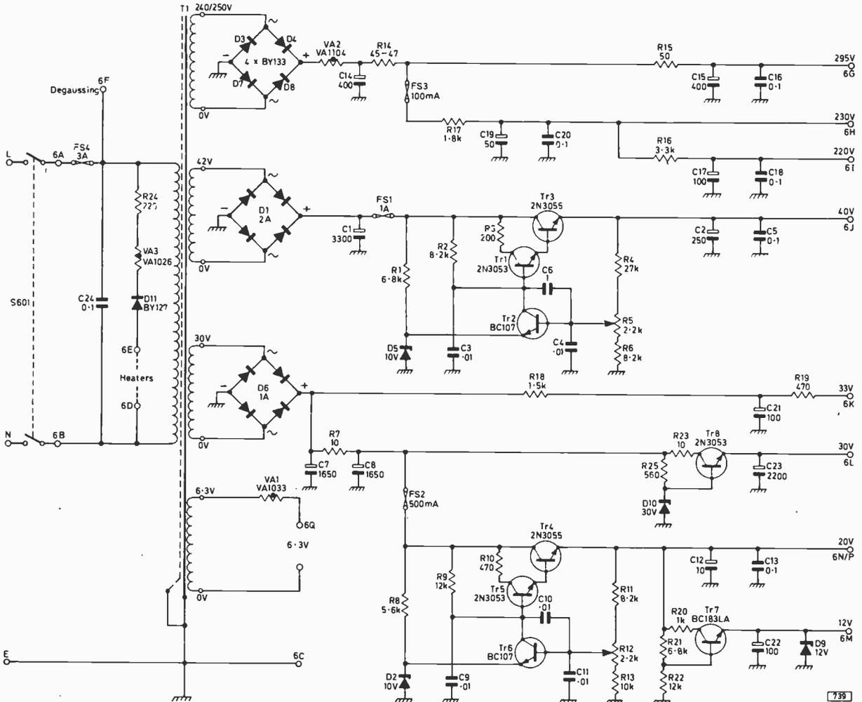
Fig. 4: Power supply circuit designed for the receiver by E. Erven, with stabilised 40V and 20V outputs. R14 can be made up from the 30Ω and 15Ω resistors (R504 and R509) supplied in the original component pack.
