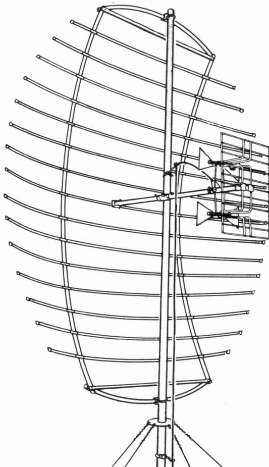
*Drawing of the Channel Master paraboloid "Super Panoscope" u.h.f. aerial.*
