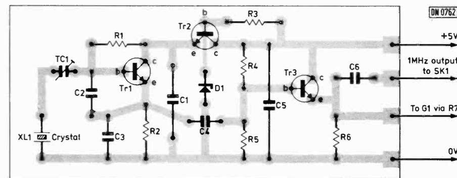
Fig. 8: Layout of the oscillator board, viewed from the copper side. (C5 is an electrolytic.)
