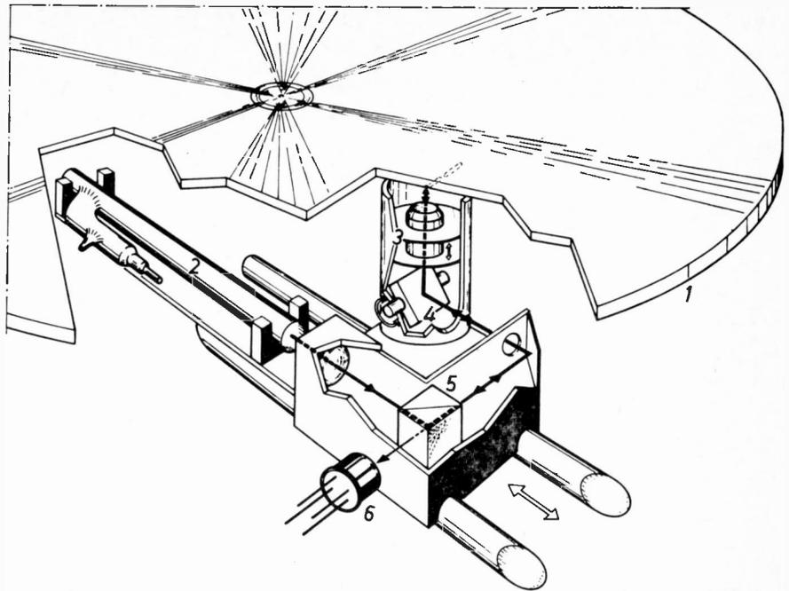
*Fig. 2 (right): Simplified schematic diagram of the VLP playback system. The disc (1) is scanned from below by light from the helium-neon laser (2). Focus lens (3) is suspended in the same way as the cone of a loudspeaker, an automatic control system providing drive so that the focus remains correct. Pivoting mirror (4) is automatically controlled to keep the beam centred on the track. Prism (5) separates the incident and reflected light which is detected by the photodiode (6).*
