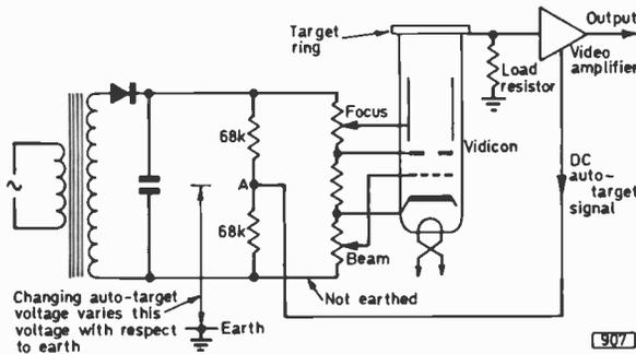
Fig. 4: Auto-target circuit based on the use of a floating power supply (i.e. neither side earthed).
