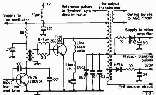
Fig. 2: Line driver and output stages of the Murphy Model V1400 14in. mains/battery portable. The npn line output transistor Tr26 is operated in the common-emitter mode.
