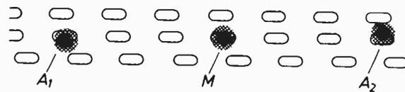
Fig. 10: Position of the main beam *M* and the auxiliary beams *A1* and *A2* in relation to the section of the track being scanned.
