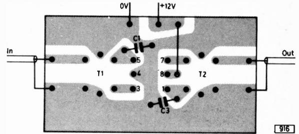
Fig. 6: Layout of the printed circuit.
