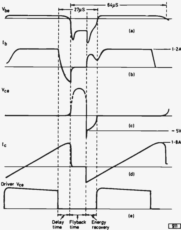
Fig. 3: Several large-screen monochrome receivers use the Mullard BU105 line output transistor. The correct waveforms in a stage using this transistor are shown above.
