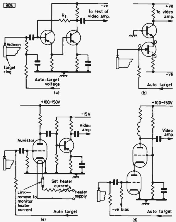
Fig. 2: Typical head amplifier circuits (simplified). (a) The feedback pair. The feedback resistor  $R_f$  may need optimising if the transistors are changed. (b) Cascode amplifier with f.e.t. input stage. (c) Valve/transistor hybrid circuit. (d) Valve cascode circuit—typically uses two nuvistors (heater circuits omitted).
