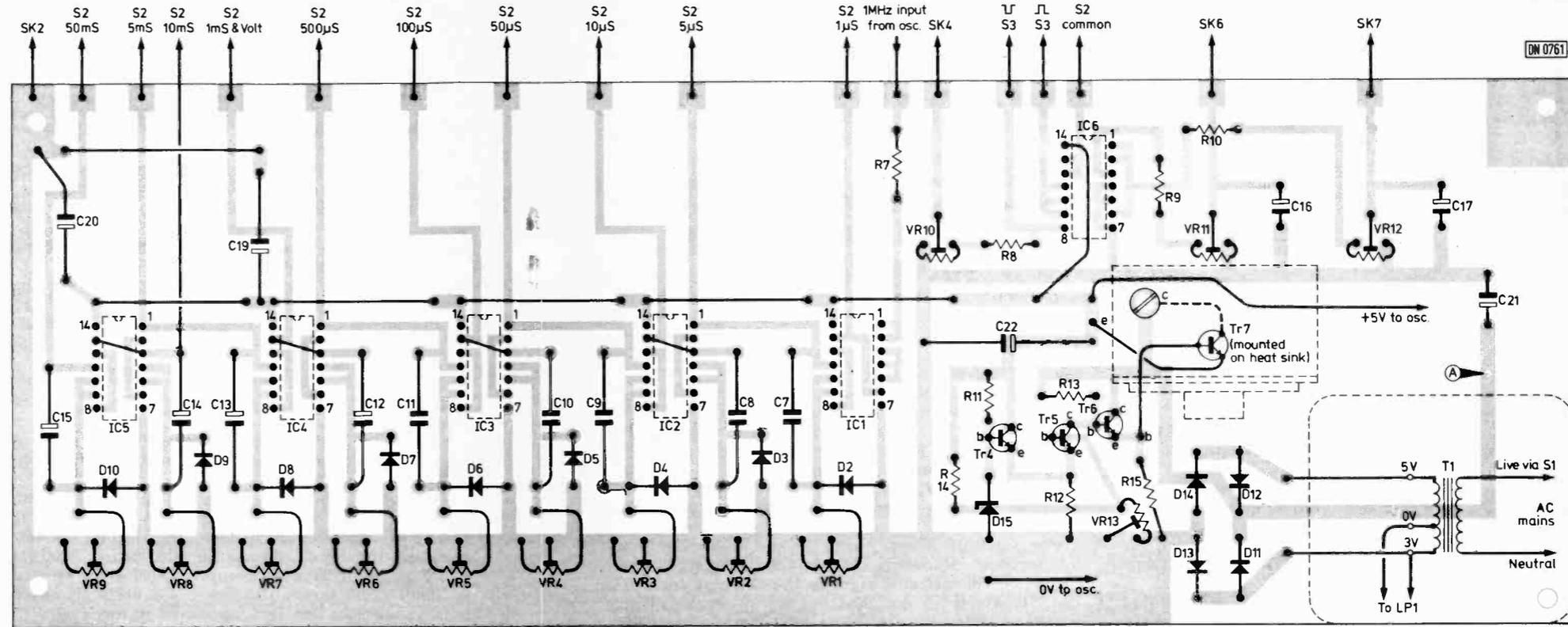
Fig. 7: Layout of the main panel used in the prototype, viewed from the copper side. Note that incorrect pin numbers were given for IC6 in the main circuit (Fig. 3) last month: the pin numbers shown there for G21 and G24 and also for G22 and G23 should be interchanged to conform with the layout above.
