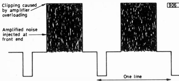
Fig. 3: Section of the output waveform.
