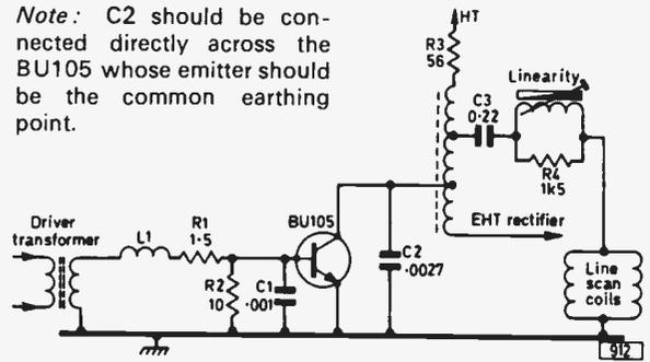
Fig. 4: The basic BU105 line output stage: the component values shown are typical of those found in practice.
