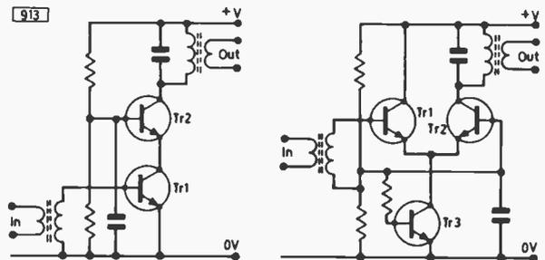
Fig. 1 (left): Cascode amplifier circuit.
