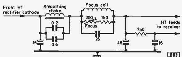
Fig. 1: Classical simplicity, the focus system used by Vidor and others.
