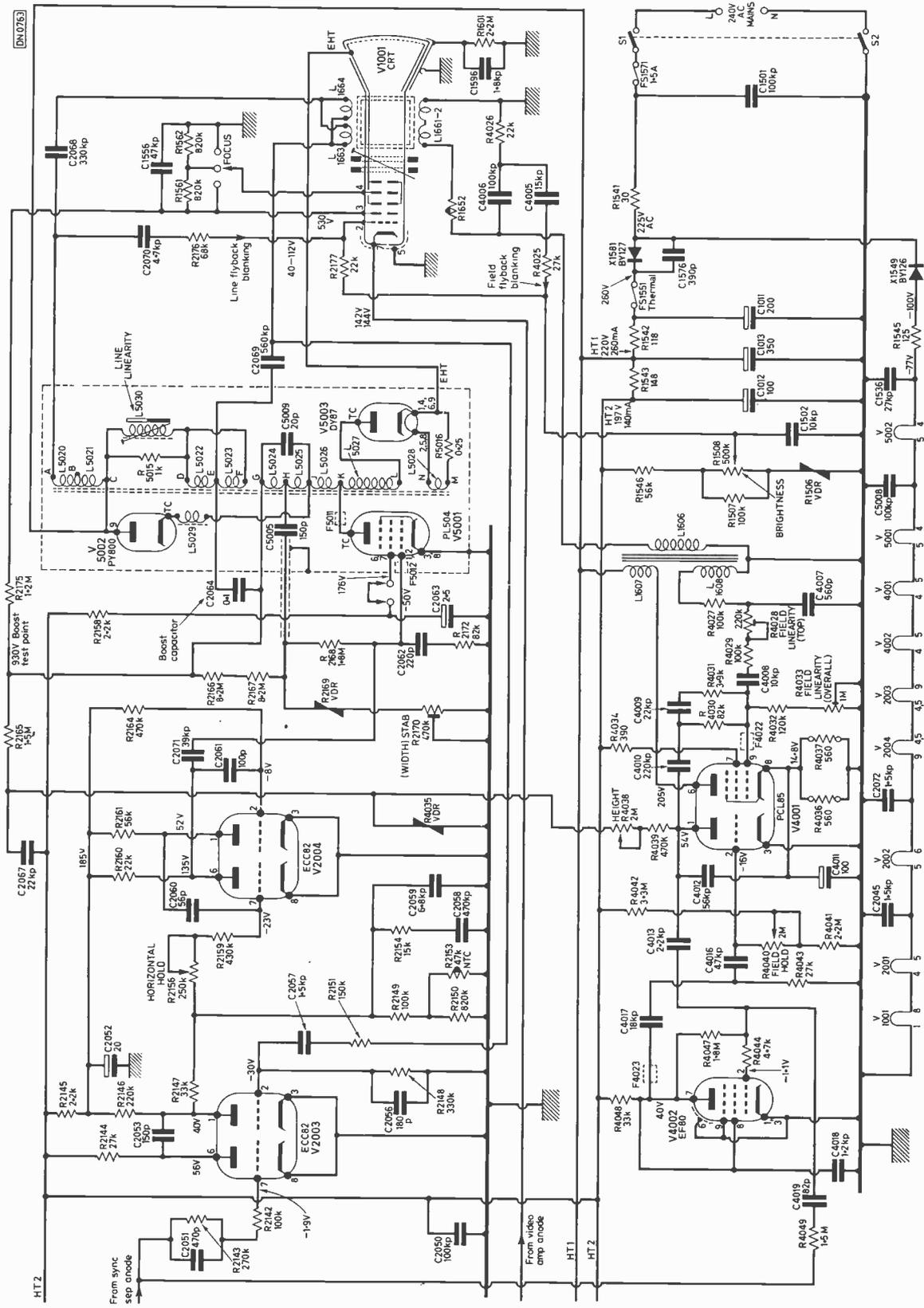
Fig. 1: Timebase and power supply circuits of the Philips 300 chassis. Voltages measured using a 100k  $\Omega$ /V meter, with no signal input. V4001 triode anode voltage varies with the height-control setting.
