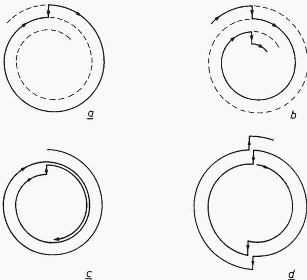
Fig. 3: Different ways of using the picture recorded on the VLP disc—twice per revolution during the field flyback period an opportunity occurs to change from one track to another. (a) A reverse jump after each revolution gives a stationary picture; (b) a forward jump after each revolution gives motion at twice the true speed; (c) reverse jump after every second revolution reduces the speed by half; (d) a reverse jump every half revolution gives reverse motion at the correct speed.
