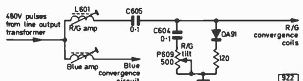
Fig. 1: Part of the horizontal R/G convergence circuit in the GEC 2040 series. Red/green horizontal convergence was well out due to lack of pulse at the junction C604/P609.
