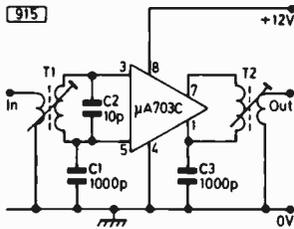
Fig. 5: Circuit of the i.f. preamplifier using the  $\mu$ A703 i.c.
