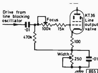
was a labyrinth of voltage dividers (see Fig. 2) supplying not only the focus potentiometer but also the contrast control and the negative side of the brightness control! By and large the system worked well enough, apart from the splendid sound-on-vision effects resulting from an open-circuit C16!
