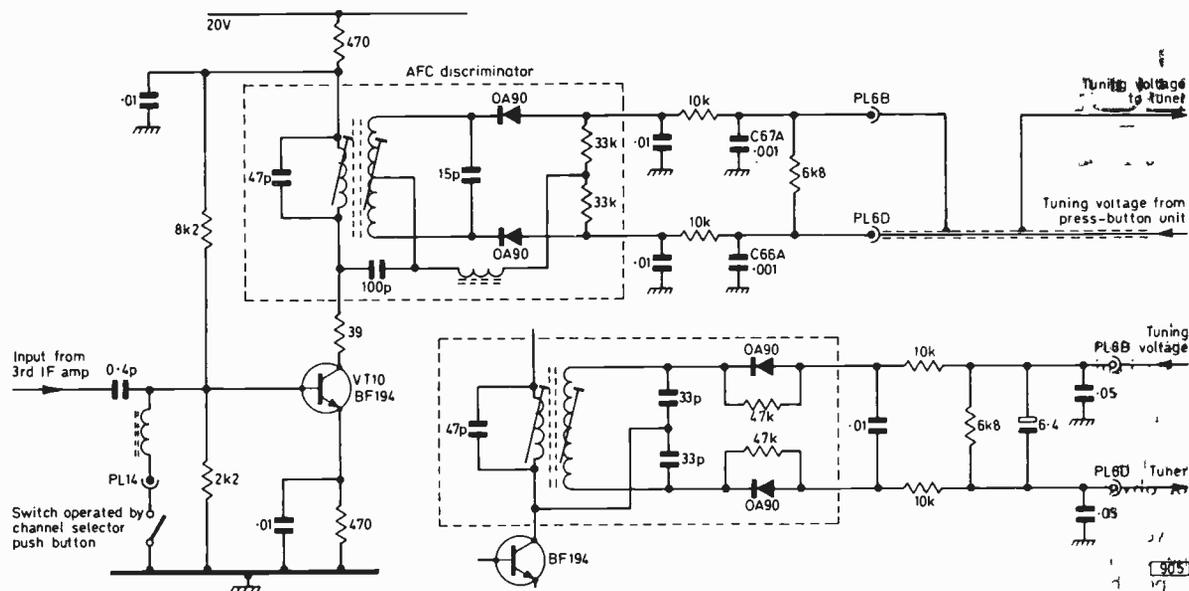
Fig. 4: Single-stage a.f.c. circuit used in chassis fitted with varicap tuners. Complete circuit, 693 chassis; below right, modifications in the 697 chassis.
