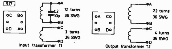
Fig. 7: I.F. transformer winding details.
