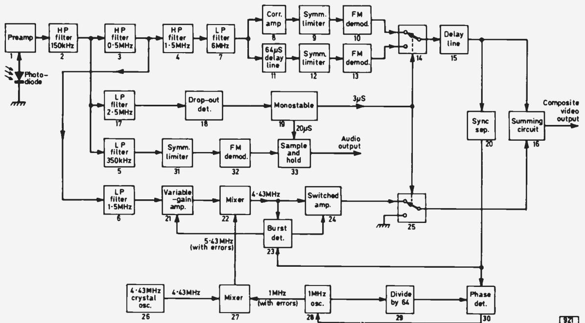
Fig. 8: Block diagram of the circuits used in a VLP player.
