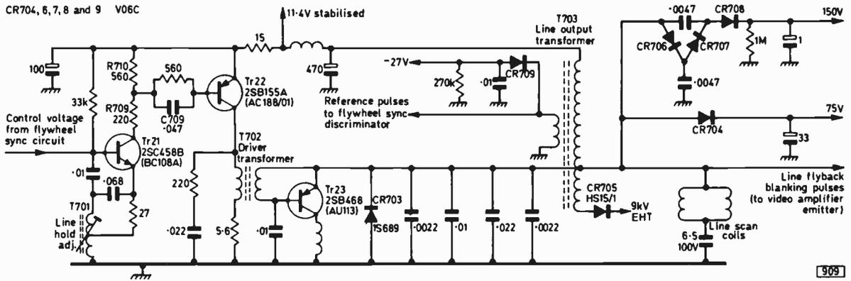
Fig. 1: Line timebase circuit used in the Ekco Model T545 9in. mains/battery portable. The pnp line output transistor Tr23 is operated in the emitter-follower mode.
