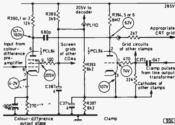
Fig. 3: Colour-difference output stage/clamp circuitry.
