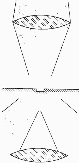
*Fig. 1 (left): How the pits in the surface of the VLP disc modulate the scanning beam.*
