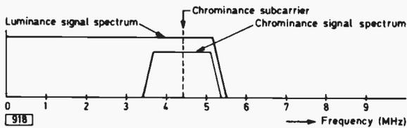
Fig. 4: Frequency spectrum of the basic PAL signal.
