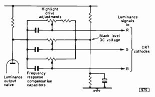
Fig. 2: Using this simple circuit, correct grey-scale tracking is maintained despite changes of h.t. voltage.
