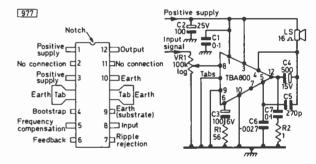
Fig. 1 (left): Pin connections to the TBA800. The TBA810S and TBA810AS are the same except that there is no connection to pin 3.
