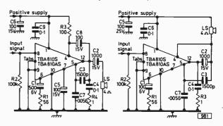
Figs. 9 and 10: Alternative audio circuits using the TBA810S or TBA810AS.
