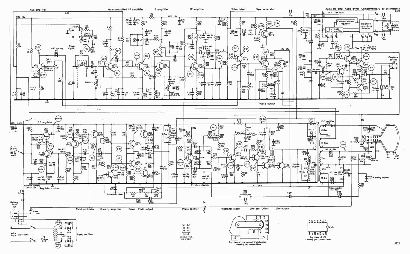
Fig. 7: Circuit diagram of the TCE/BRC 1591 chassis, schedule C. The 1590 chassis differs as follows: R131 150k Ω; C106 3,900pF; C115 fitted; C42 and R49 omitted. See also modifications on page 507.
