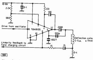
Fig. 13: Field output stage for 12-17in. monochrome receivers, using the TBA810S.
