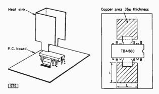
Figs. 5 and 6: Alternative heatsink arrangements for the TBA800 and TBA810S.
