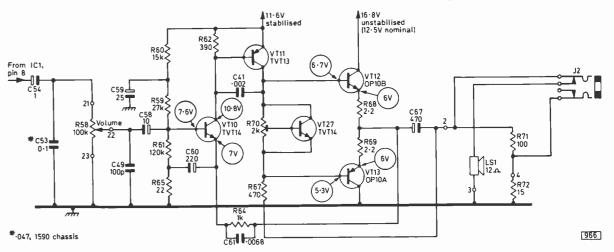
Fig. 6: Audio circuit used in later versions of the chassis.
