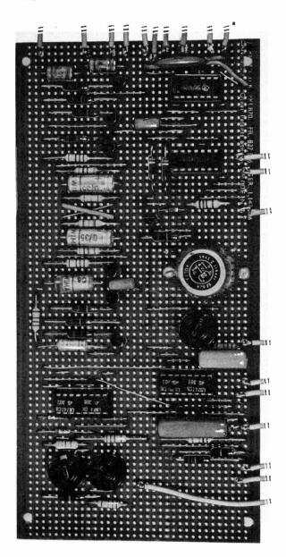
Photograph of the simple game board, showing the component side.
