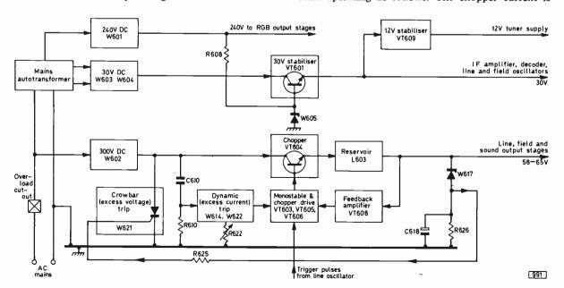
Fig. 3: Block diagram of the power supply arrangements used in the BRC/TCE 3000/3500 colour chassis.
