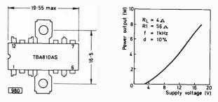
Fig. 7 (left): Outline drawing of the TBA810AS.
