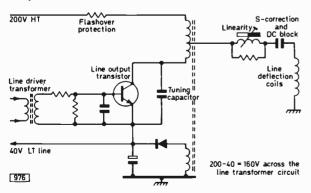
Fig. 3: Simplified transistor line output circuit using the anti-boost technique.
