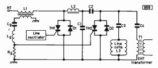
Fig. 1: Basic elements of the thyristor line timebase used with thin-neck 110° shadowmask tubes.
