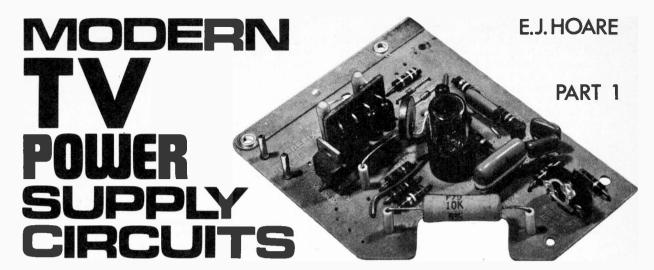
It was only a comparatively short time ago that the design of power supplies for most monochrome and colour receivers involved little more than routine care. The circuits were simple, usually consisting of a diode or two and one or more tapped dropper resistors for obtaining the appropriate h.t. and heater voltages. Matters have changed now and those days have gone for ever—or for at least as far as we can see into the future.
