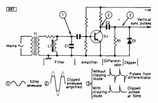
Fig. 4: Method of deriving the field drive pulses from the mains.
