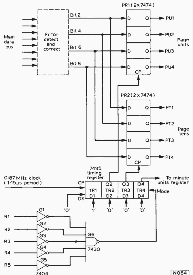
Fig. 15: A page address detection circuit.
