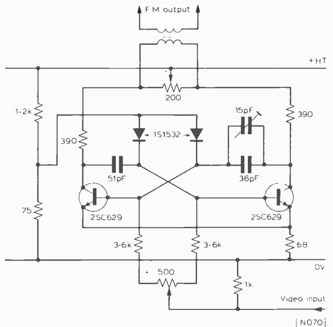
Fig. 13: A typical multivibrator f.m. generator.
