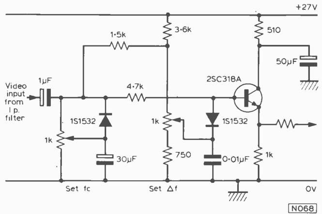
Fig. 11: Deviation control circuitry.
