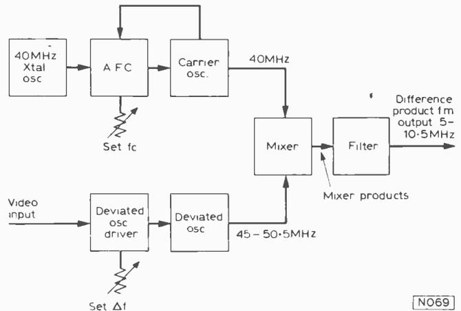
Fig. 12: Two-oscillator method of f.m. generation.
