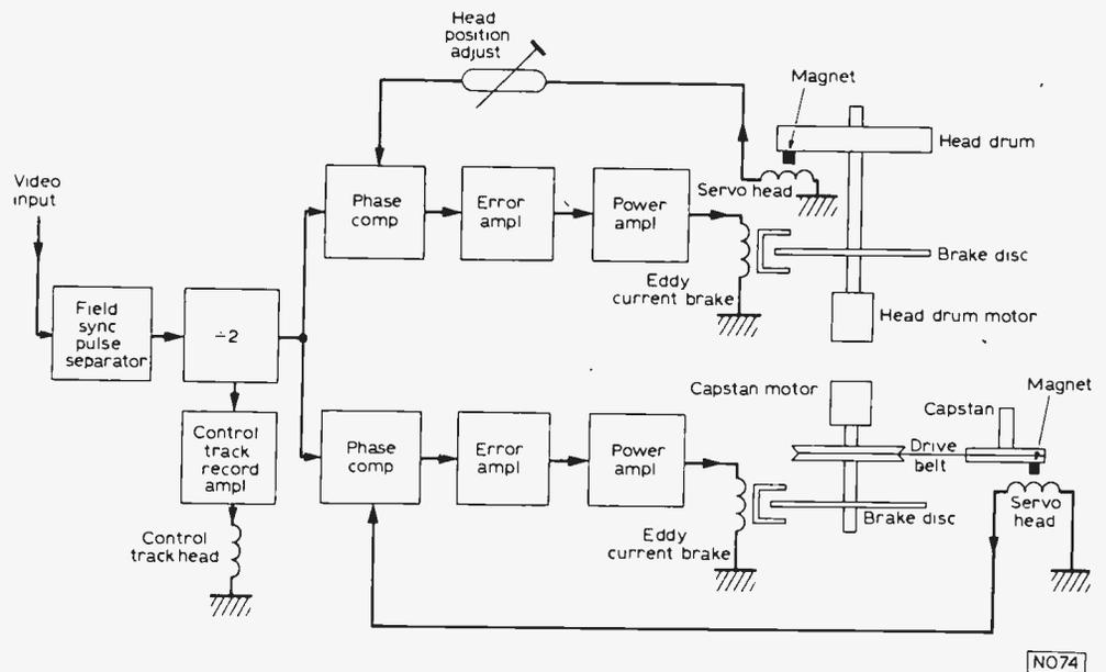
Fig. 16: A typical VTR servo system in the Record mode.
