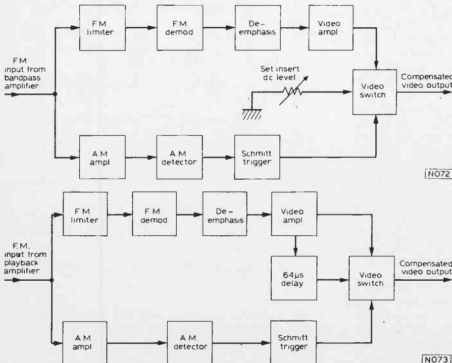
Fig. 15: Dropout compensation circuits.
