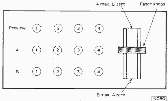
Fig. 4: Video mixer front panel layout.
