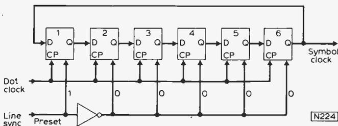
Fig. 45(b): A symbol clock divider using a shift register.
