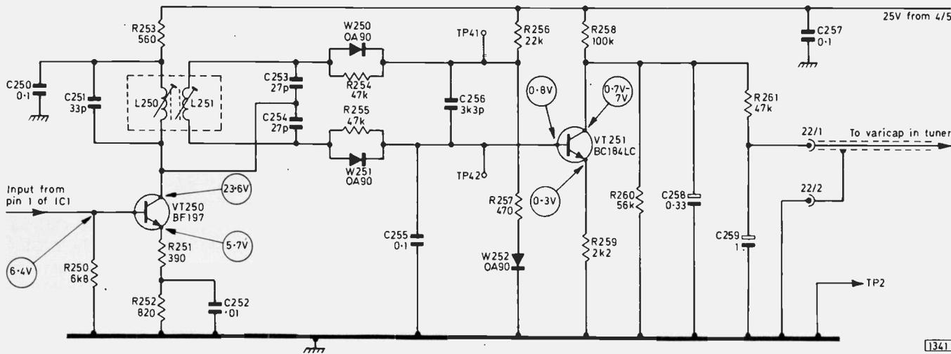
Fig. 6: The a.f.c. subpanel circuit.
