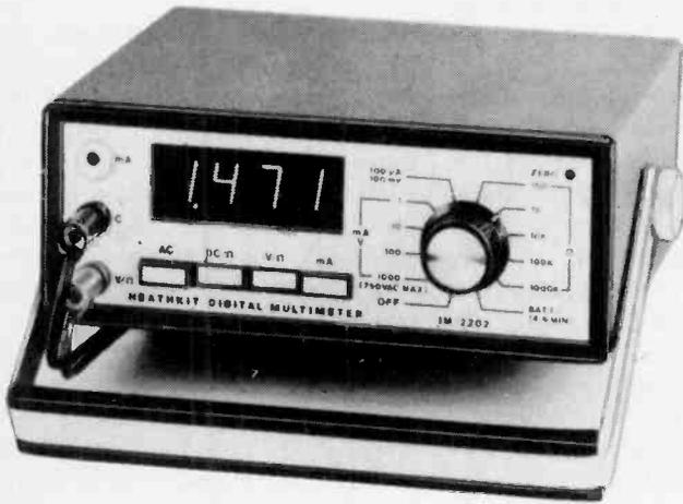
The Heathkit IM-2202 is a compact instrument with a very respectable specification. On switching it on for the first time our reaction was "Oh, aren't they big?" Shades of the Bishop and the actress, but we refer here to the display digits. In point of fact the digits, at 14mm (0.55in) high are the same size as those in several other instruments we looked at, but somehow the presentation makes them seem larger.
