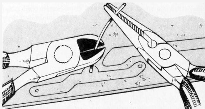
Fig. 1: When cropping excess wire from a joint on a printed panel, hold the free end to prevent it falling down into the chassis where it may cause a short-circuit.
