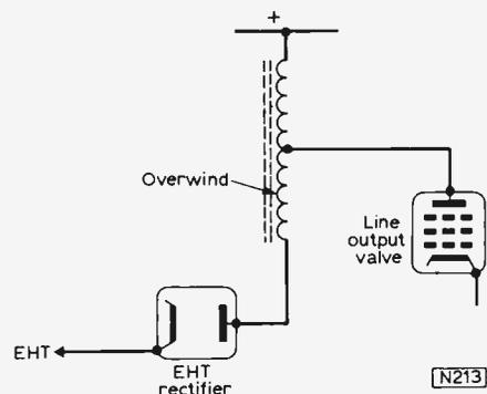
Fig. 5: Basic principle of e.h.t. generation by the line output stage.
