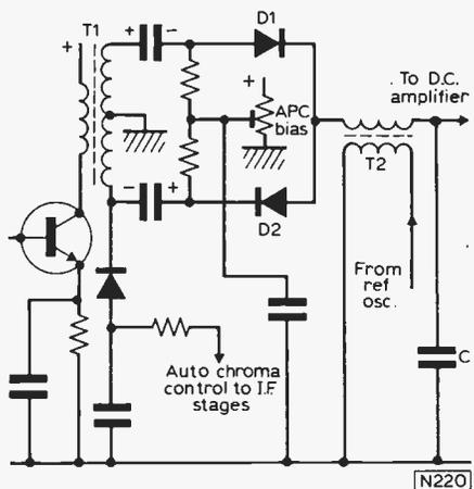
Fig. 12: A burst detector circuit. This phase sensitive detector produces a control voltage to lock the receiver's reference oscillator to that at the transmitter.
