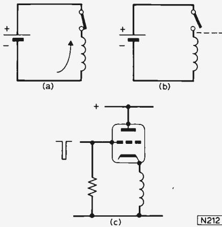
Fig. 4: Moving the switch to the opposite end of the inductor does not alter the circuit action, only the polarity of the induced voltage. This will always be opposite to the voltage that was applied.
