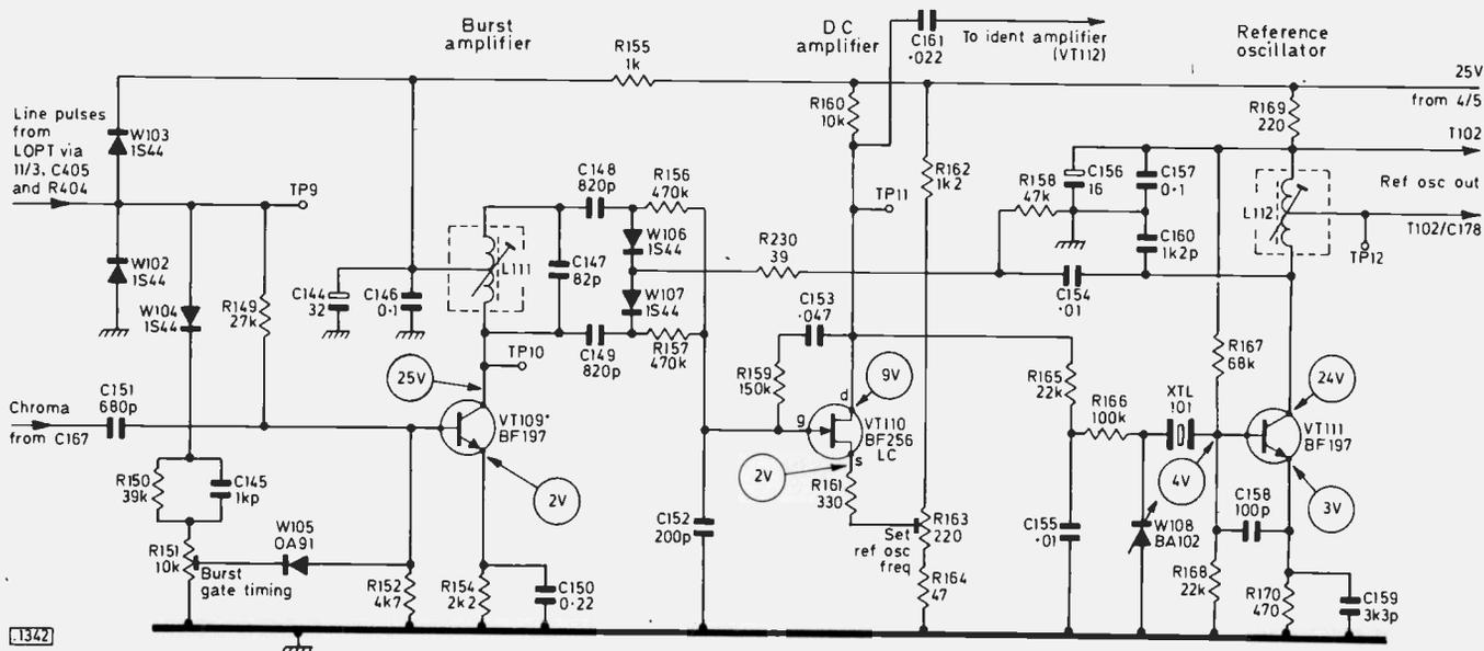
Fig. 7: The burst channel and reference oscillator circuits.
