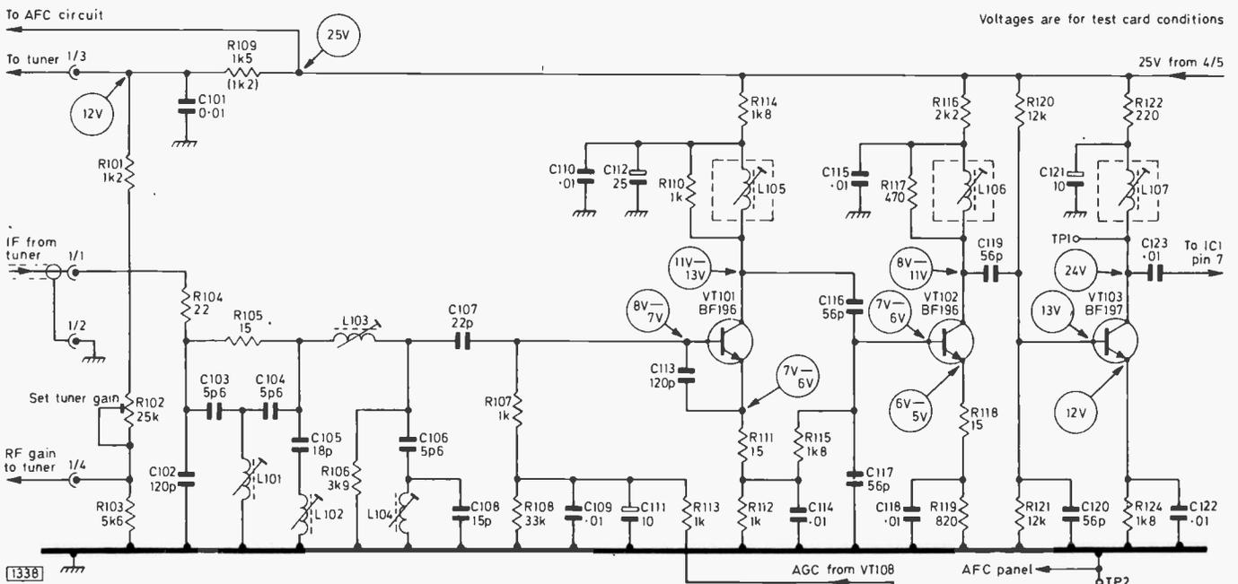
Fig. 2: Circuit of the i.f. amplifier.
