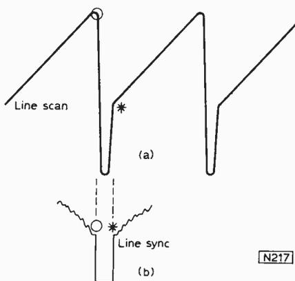
Fig. 9: Relative timing of line scan and line synchronising pulses.
