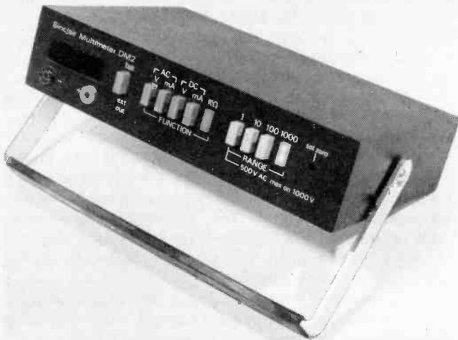
This is one of the least expensive DVMs on the market, yet it has most of the facilities and specifications of its more pricey counterparts. Function and range selection are by push-buttons. The case is extremely rugged, being made of cast aluminium. The power source is an internal PP9.
