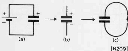
Fig. 1: (a) A capacitor stores electric energy in the form of an electric field. (b) The field remains when the capacitor is disconnected from the voltage, until . . . (c) A closed circuit is set up, when the charge moves as a flow of current.
