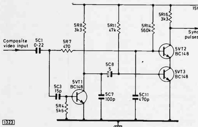
Fig. 4: This circuit, used in the Rank Z504 scan drive panel, discriminates between noise and the sync pulses by the higher amplitude and greater bandwidth of the former, 5C3 and 5R4 forming a high-pass filter.
