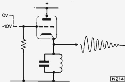
Fig. 6: A simple ringing circuit. Note how the amplitude of the oscillations decreases.
