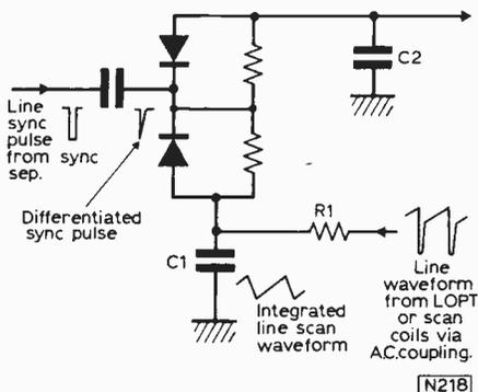
Fig. 10: A typical flywheel line sync circuit.
