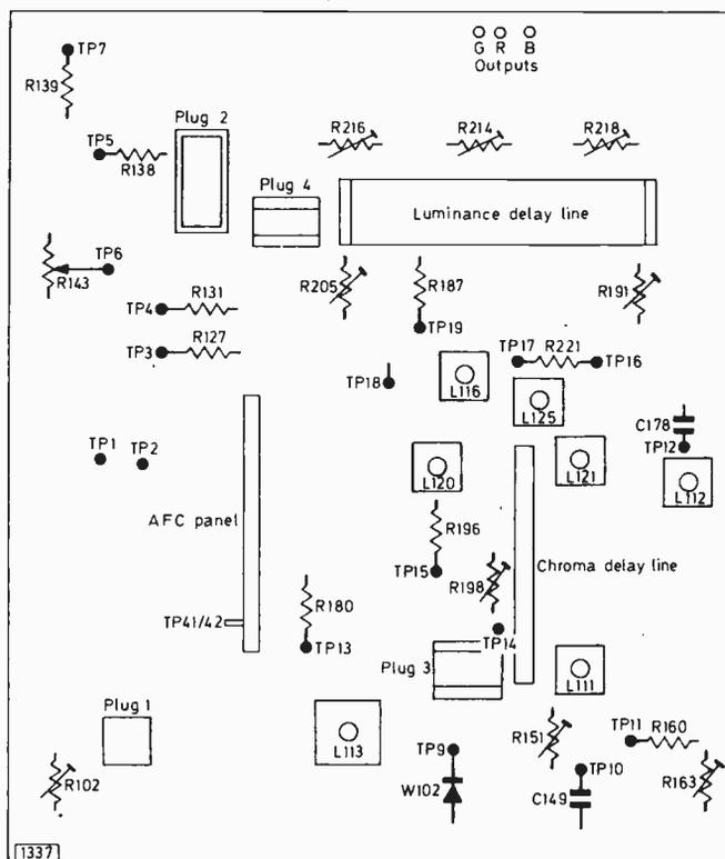
Fig. 5: Positions of the i.f. and decoder test points and preset controls on the panel.
