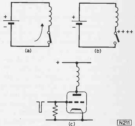
Fig. 3: When an inductive circuit is broken, a high voltage is induced in the inductor.
