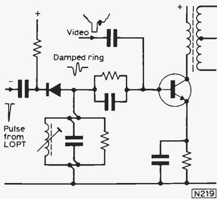
Fig. 11: A typical circuit for gating out the line-by-line colour burst for use by the burst detector.
