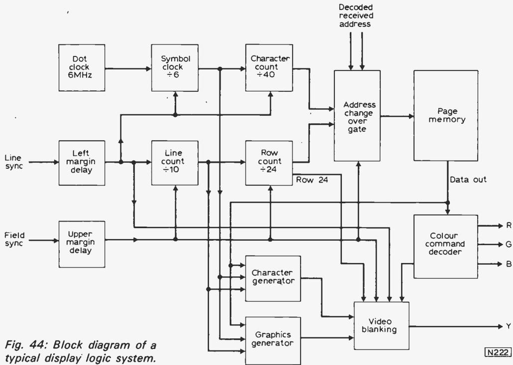
Fig. 44: Block diagram of a typical display logic system.
