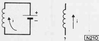
Fig. 2: An inductor stores energy in its magnetic field. What happens when the circuit is broken?
