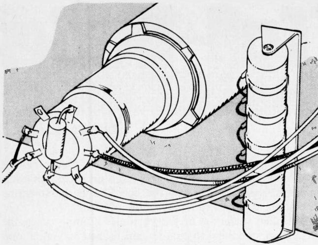
Fig. 2: Tube base leads caught around the mains dropper: make sure that all wiring is routed clear of power resistors and sources of high pulse voltages.
