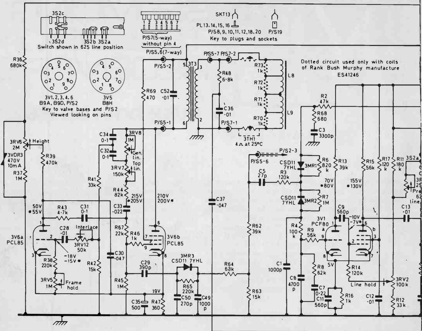
Fig. 1: Circuit of the power supplies and timebases, Bush TV161 series. Voltages marked with an asterisk apply to 625-line of sections.
