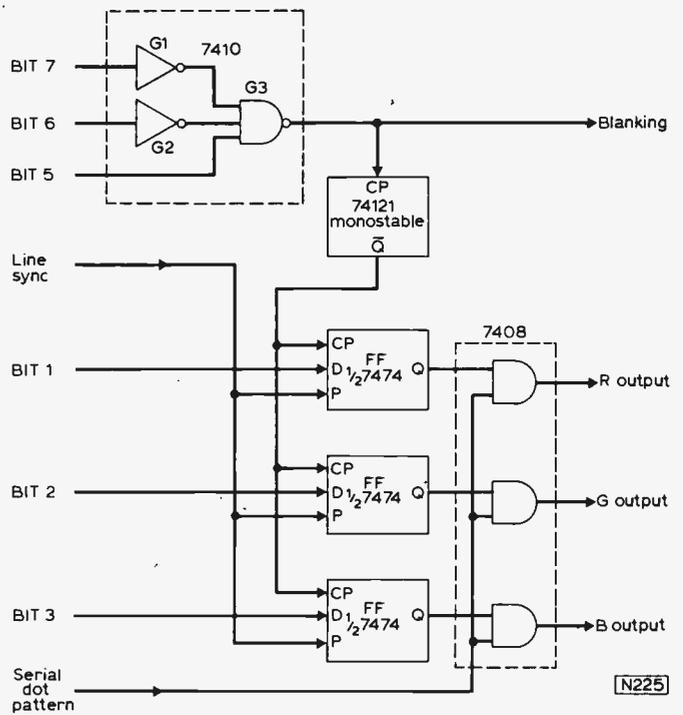
Fig. 46: Colour decoding logic.
