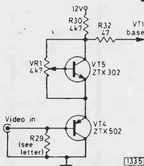
Fig. 1: Circuit used by M. T. Hawkins to d.c. couple a 1V video signal with its sync pulses clamped to earth to the u.h.f. modulator. The emitter-follower VT4 also provides the first 0.7V of the required level shift, the rest being provided by the amplified diode VT5 whose voltage drop is set by VR1.
