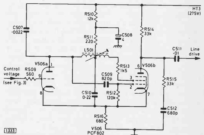
Fig. 1: The line oscillator circuit. The line output stage circuit was shown in Fig. 2, page 518 of the September issue.
