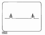
Fig. 6 (left): Typical oscillogram showing a correctly adjusted burst gate.
