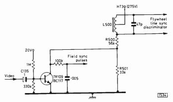
Fig. 2: The sync separator circuit used in the GEC hybrid colour chassis. The collector load resistor R500 tends to go high-resistance. In the case in question the result was various colour faults plus bent verticals.
