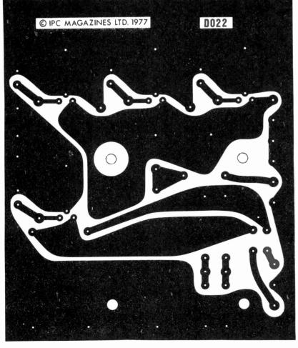
*Fig. 5: The printed circuit board for the power supply shown full size.*
