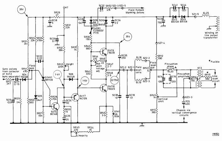
Fig. 1: Field timebase circuit used in the Rank A823A/AV/B chassis.
