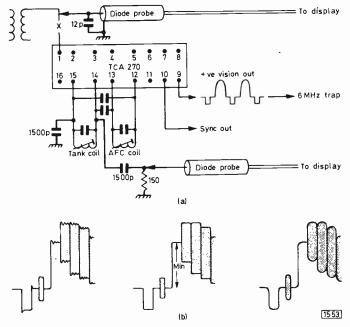
Fig. 10: Aligning the TCA270 vision synchronous demodulator i.c. (a) Connections for i.f. alignment: either break the input at X and load the diode probe with a 12pF capacitor, or decouple pin 15 and connect the diode probe to pin 14 as shown. (b) Aligning the tank coil. Look at the output from pin 9 after the 6MHz trap, and adjust for minimum height of the white bar consistent with the squarest response. Left, vision carrier too low; centre, on tune; right, vision carrier too high.
