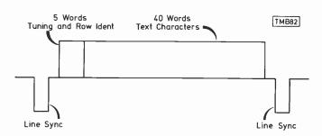
Fig. 1: Layout of transmitted data.
