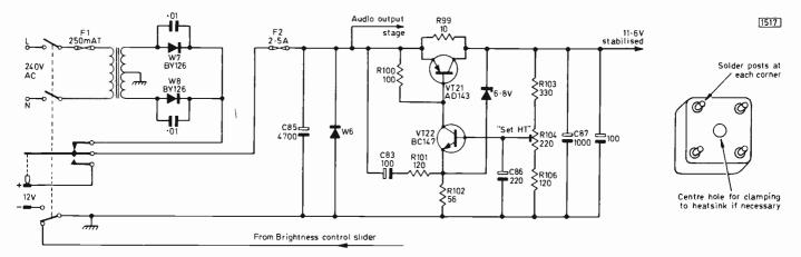
Fig. 5 (left): The power supply circuit used in the Thorn 1590/1/3 chassis. A suitable Mullard replacement for the series regulator transistor VT21 is the AD149.
