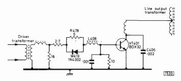
Fig. 1: Line output transistor circuit used in the Thorn 8500 chassis. A dry-joint on L408 upset the drive conditions, leading to demise of the line output transistor and, subsequently, lack of width and loss of line sync when a replacement transistor was fitted.
