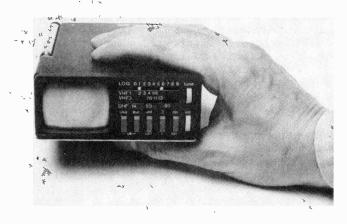
The Sinclair Microvision is the world's first hand-held TV set. It operates on three different standards.
