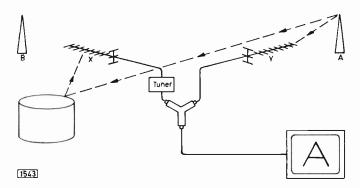
Fig. 4: The final installation. The tuner attenuates the signal picked up by aerial X when receiving station A.
