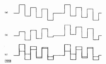
Fig. 7: The use of coincident traces in chroma alignment. (a) Correct B-Y waveform. (b) Phase displaced: alternate lines as seen on an oscilloscope scanning consecutive lines. (c) Phase displaced, this time alternate lines as seen on an oscilloscope superimposing alternate lines as required to give correct alignment.
