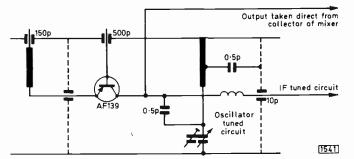
Fig. 2: Pressing an old tuner unit into service as a narrowband amplifier. Take the output directly from the collector of the mixer transistor, not from the i.f. output point. The tuner unit used was one from a Thorn 1500 chassis.
