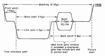
Fig. 5: Line flyback blanking period parameters.
