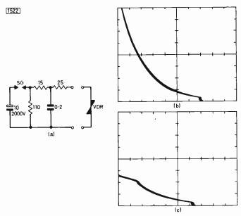
Fig. 1: (a) Lightning simulation test circuit. (b) Voltage waveform without the VDR in circuit. (c) Voltage waveform with VDR included. Vertical scale 200V/division, horizontal scale 500µs/division. Courtesy Mullard Ltd.
