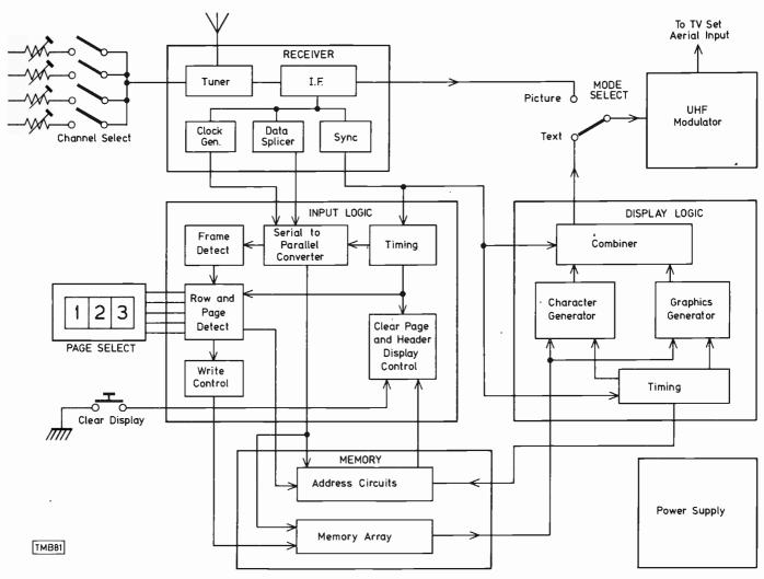
Fig. 2: Block diagram of the Television Teletext Decoder.
