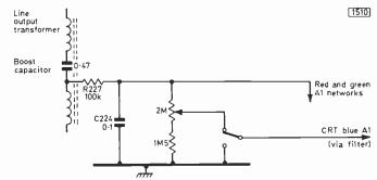
Fig. 1: The c.r.t. first anode supply on the Pye hybrid colour chassis. The filter components R227/C224 between the boost line and the first anode preset potentiometers are a regular source of trouble on these chassis.
