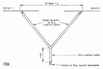
Fig. 1: Method of interconnecting two stacked aerials. To calculate a quarter wave, use the formula (246/f) x cable velocity factor. Answer in feet; frequency f in MHz.
