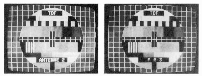
*Two shots of the PM5544 test pattern as used by France. Left, the second chain; right, the third chain. These photographs by D. F. Brown (near Brighton, Sussex) were taken in colour from the screen of his SECAM receiver.*
