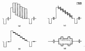
Fig. 2: Alignment of the 4.43MHz subcarrier trap in the luminance channel. (a) Composite video signal entering the decoder. (b) The same signal after passing via the subcarrier trap – note the low chroma content and the otherwise sharp rise times. (c) The effect of insufficient trapping: note the large amount of chroma on the transients. (d) Normal chrominance waveform with the luminance signal removed – the "cotton reel".
