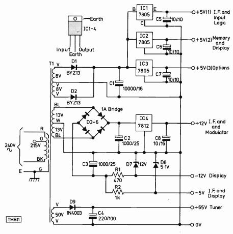
Fig. 3: Circuit diagram of the power supply unit. Component details will be found in the components list at the end of this article.
