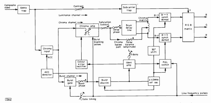
Fig. 1: Basic decoder block diagram. The contrast and saturation controls are sometimes linked so that they track together
