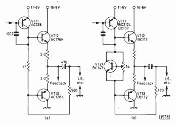
Fig. 4: Audio driver and output circuits used in the Thorn 1590/1/3 series chassis. (a) Original circuit using germanium transistors. (b) Later circuit using silicon transistors.
