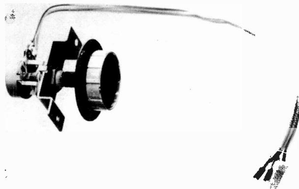
*The rotary tuning drive system designed for the 1690/1691 series of monochrome portables.*
