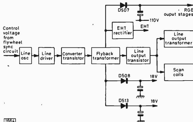
Fig. 5: Block diagram of the line timebase, showing how various supplies are obtained from the converter stage between the line driver and output stages.
