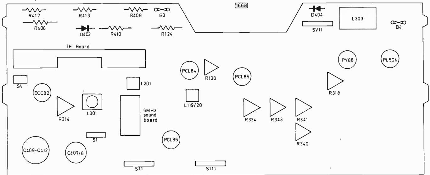
Fig. 2: Layout of the main components on the main printed circuit board.
