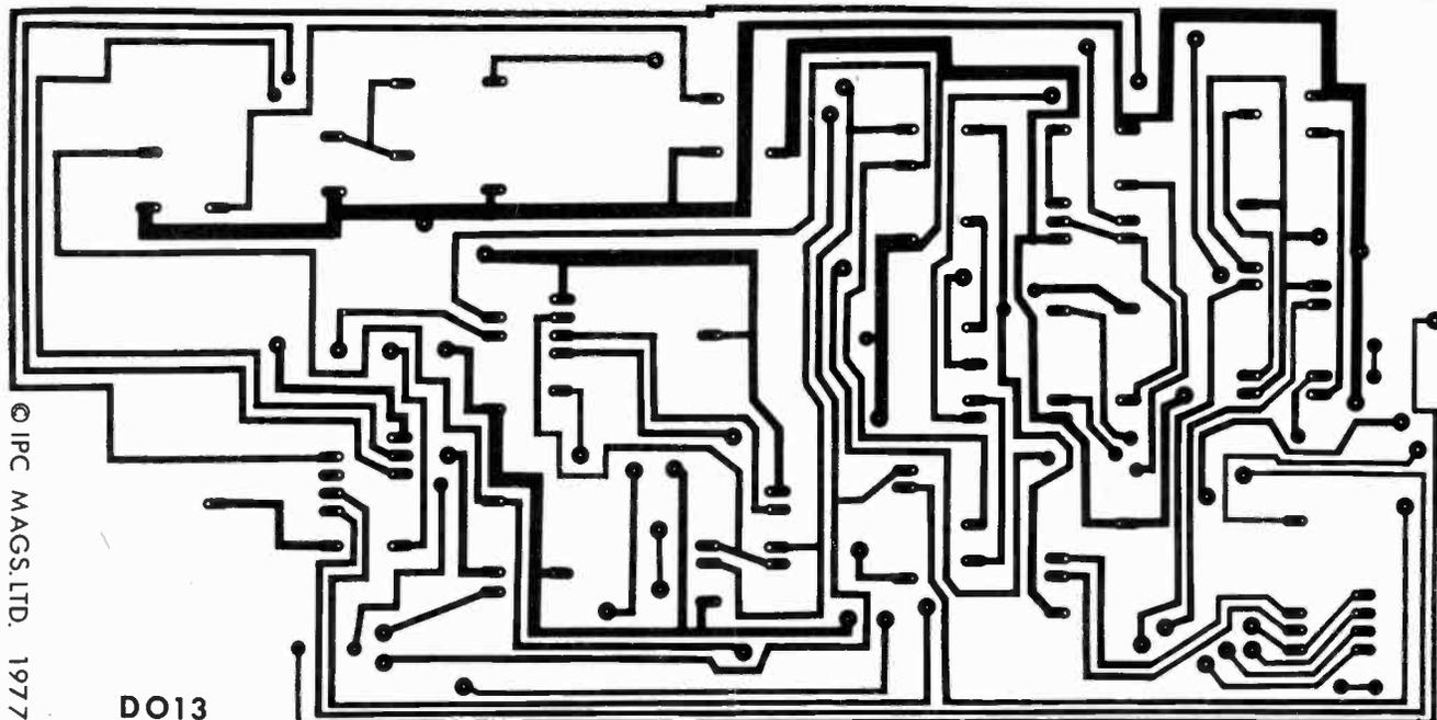
Fig. 3: Copper print on the top side of the p.c.b. The full size of the board is 4in. x 8.375in.
