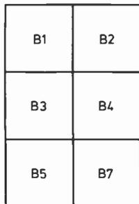
Fig. 1: Representation of a graphic cell made up of six segments with the assigned data bits shown for each segment.
