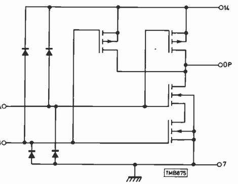
Fig. 5 (top) shows the equivalent circuit in Fig. 1 of CMOS devices which can be used as alternatives - see text. Fig. 6 (below) shows drilling details for the lid of the diecast box which accommodates the l.e.d.s.
