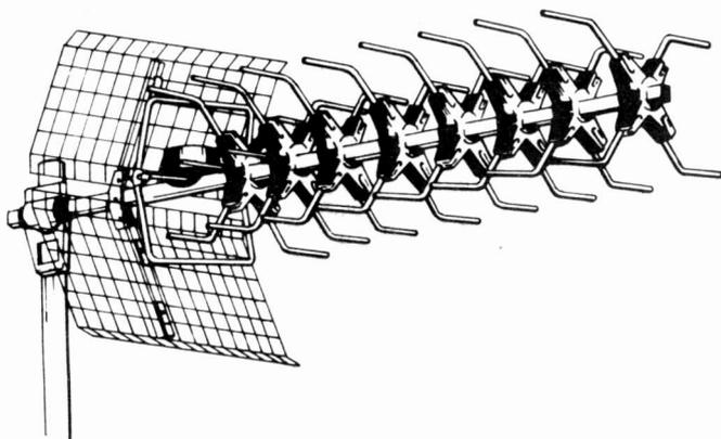
The new range of Multibeam u.h.f. aerials, the MSG range, features an extra large screen-grid reflector to give improved directivity. There are three models, the MSG8, MSG15 and MSG21, with eight, fifteen and twenty one multi-element director assemblies respectively. The aerial shown above is the MSG8.
