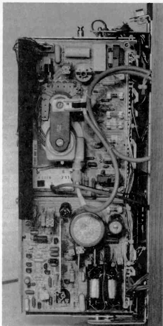
*The component sides of the printed boards. Considerable ingenuity was required in order to pack the components into the available board area. Note the field timebase i.c. with its heatsink towards the centre of the timebase panel (top left). The line scan board (top right) is dominated by the diode-split line output transformer.*
