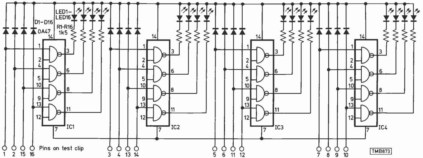
Fig. 2. Complete circuit diagram of the unit.
