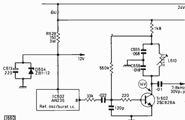
Fig. 1: Loss of colour and also faulty PAL switching were traced to this section of the decoder in the National Panasonic Model TC42G. The ident tuning coil L610 occasionally needs peaking for maximum ident output and hence optimum colour stability.
