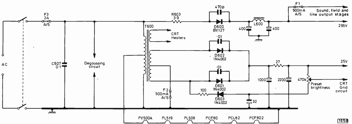
Fig. 1: Circuit diagram of the power supplies.
