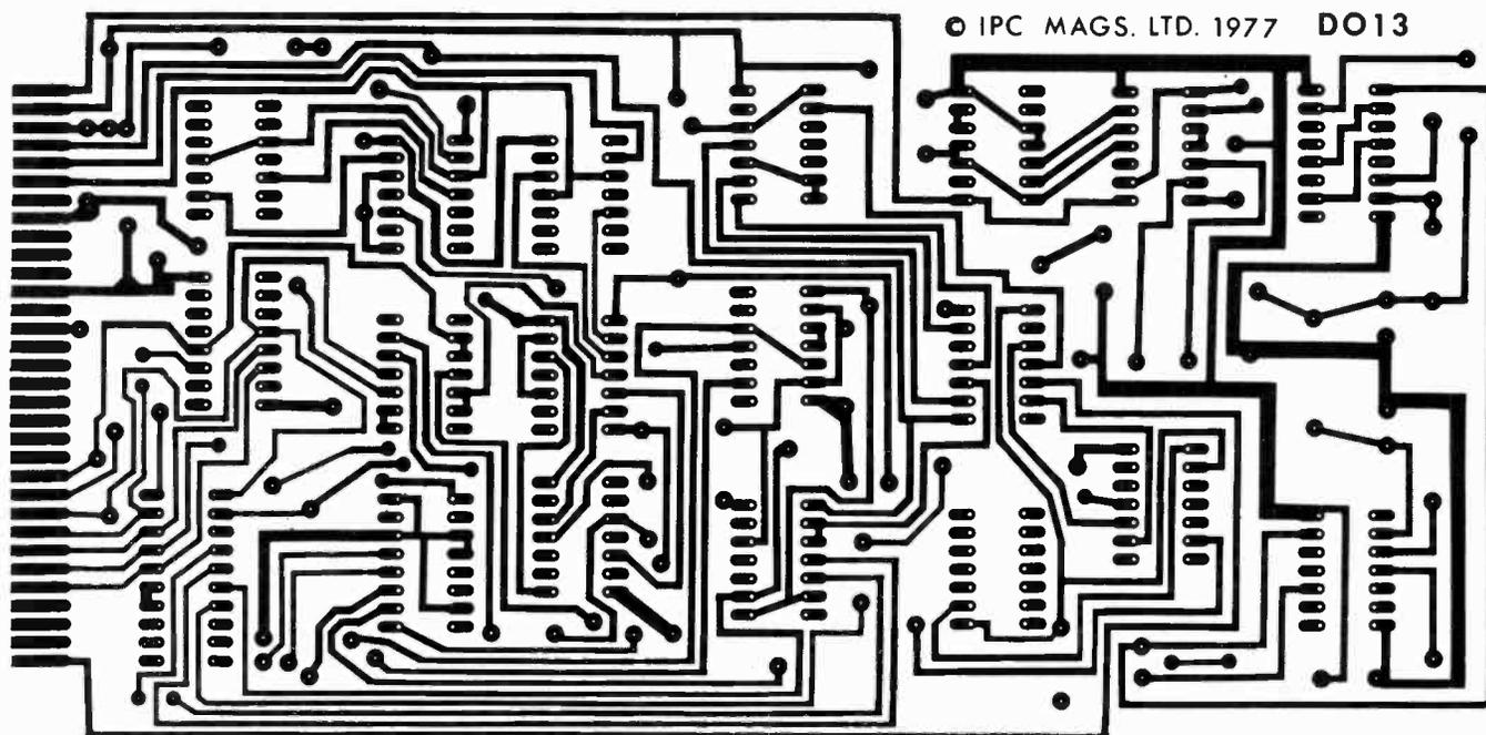
Fig. 4: Copper print on the under-side of the p.c.b.
