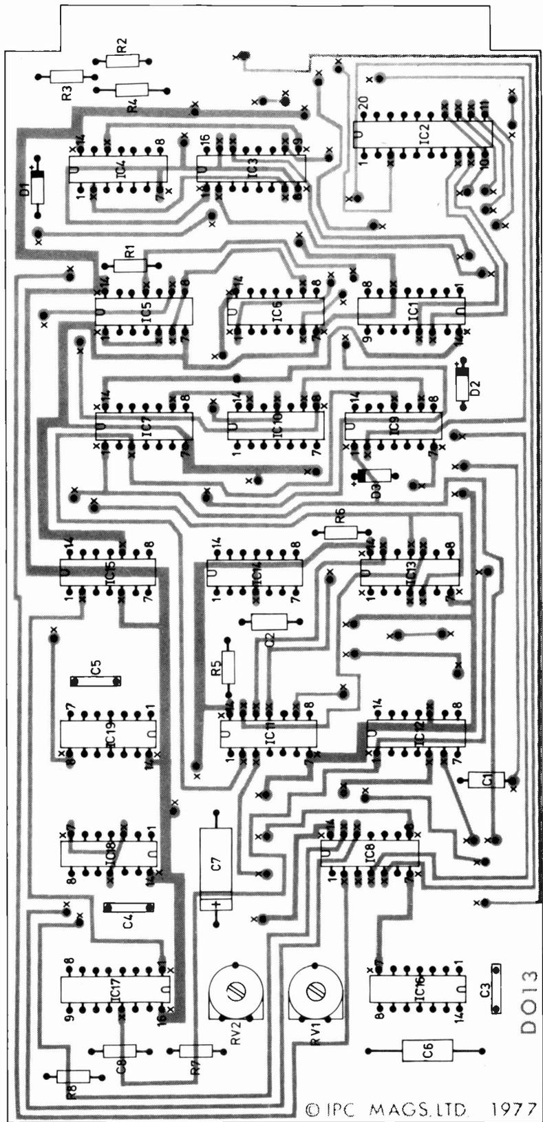
Fig. 5: Component layout diagram for the display board.
