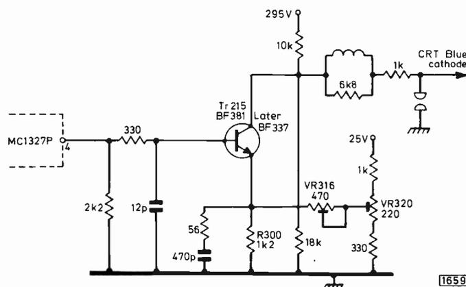
Fig. 2: One of the RGB output stages.
