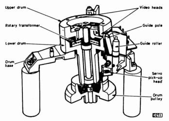
Fig. 2: Cut-away view of the head drum assembly.
