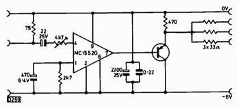
Fig. 2: Alternative version of the circuit for use as a pulse distribution amplifier.
