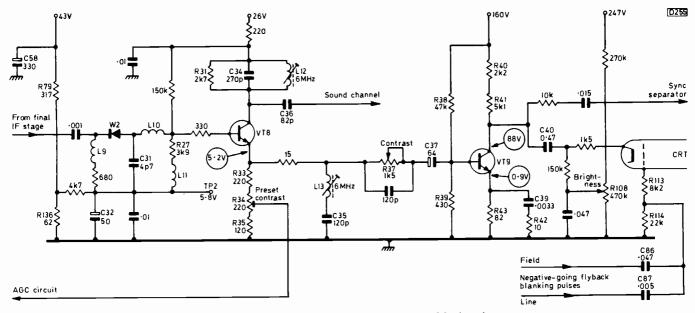
Fig. 1: Video circuitry used in the Thorn 1500 chassis.
