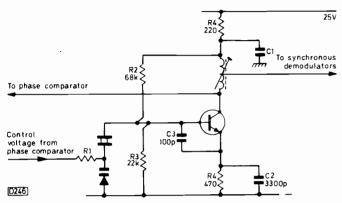
Fig. 6: Typical decoder reference oscillator circuit.
