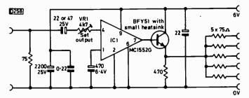
Fig. 1: Steve Beeching's video distribution amplifier circuit. Adding a  $22k\Omega$  resistor between pin 1 of IC1 and chassis alters the output as shown in Fig. 3(b).
