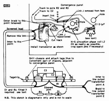
Fig. 2: Physical layout of the modification.
