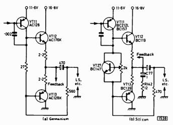
Fig. 2: Audio circuit modifications when silicon devices are used in the output and driver stages. The network C77, R142 was added to improve the audio stability.
