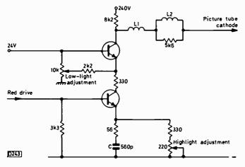
Fig. 3: Simplified circuit of a cascode RGB output stage for a colour receiver using a PIL tube.
