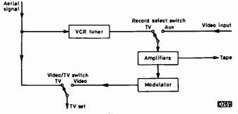
Fig. 1: Input/output switching.
