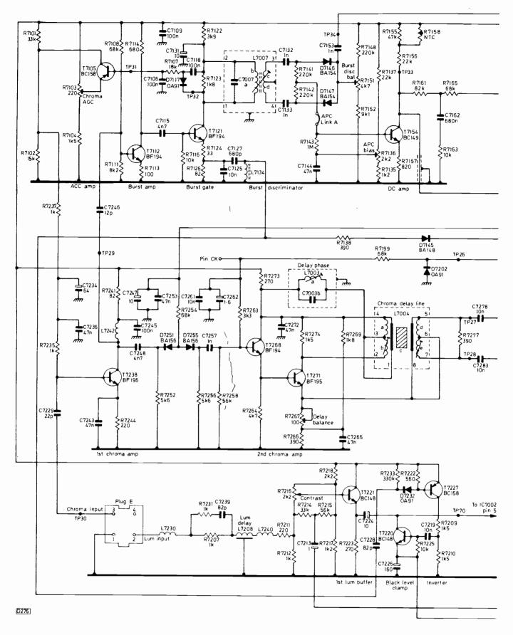
Fig. 9: Circuit of the two-i.c. decoder
