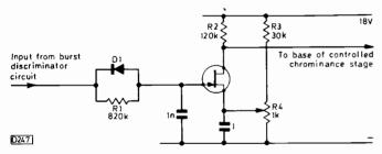
Fig. 7: Field-effect transistor used as an a.c.c. amplifier.
