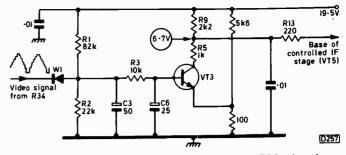
Fig. 3: A.G.C. circuit used in the Thorn 1500 chassis.
