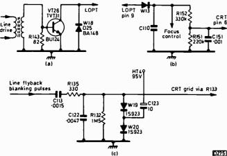
Fig. 3: Recent modifications. (a) Use of silicon line output transistor. (b) Revised c.r.t. first anode supply with c.r.t. type TMT31-102. (c) Spot-quench circuit.
