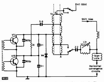
Fig. 3: Line output stage circuit (simplified) used in the Thorn 2000 chassis. The raster correction circuit is connected across points E and A. Note that there are three "LOPTs" in all in the 2000 chassis. One is used in the separate e.h.t. generator circuit. The other two (T3/4) are connected in parallel in the line output stage.
