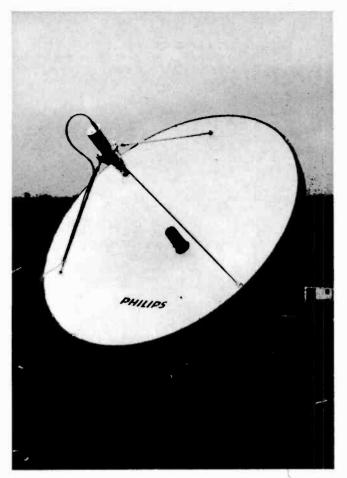
Philips 1.2m dish/head end used for the Canadian CTS satellite experiments.
