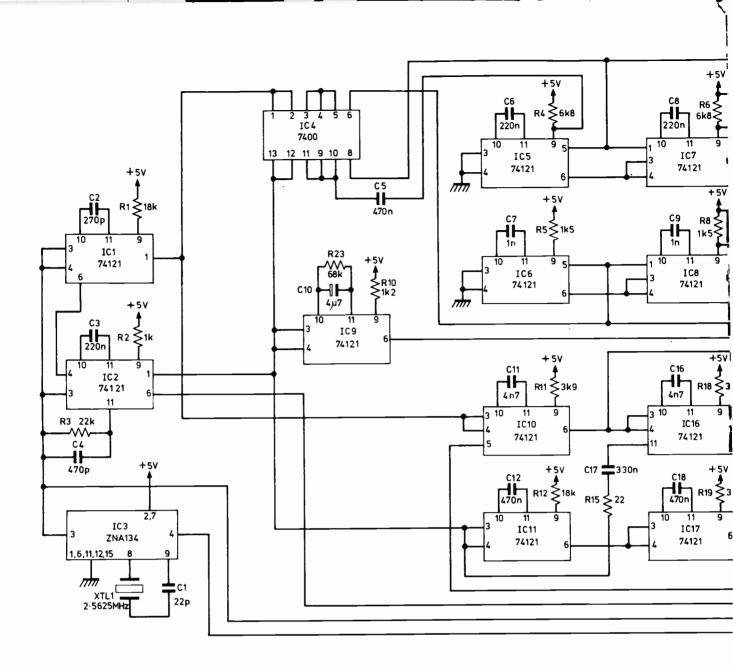
for the start of the streak pattern and, despite the apparently similar time-constant, IC15 ends the pattern (due to R15/C17, which mix a little of the field waveform in to give the curved leading edge, the time-constant of IC16 is shortened slightly). The value of R17 is selected to make the tip of the pattern as narrow as possible.
