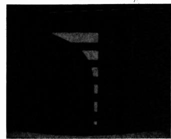
Simulated teletext and negative streak chart shown on a set with slow field flyback.
