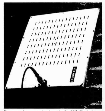
Prototype planar array developed by the BBC. The half-wave slots are spaced approximately one wavelength in the H plane and one half wavelength in the E plane.
