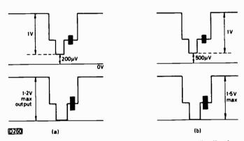
Fig. 3: Output waveforms obtained from the video distribution amplifier circuit. (a) Standard 6V circuit. (b) Circuit with 6V supply and  $22k\Omega$  resistor added between pin 1 of IC1 and chassis (across the 470µF capacitor).
