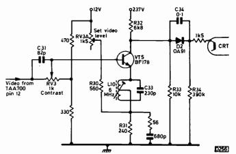
Fig. 2: Video circuit used in the Pye 169/569/173 chassis.
