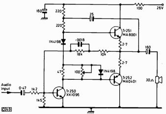
Fig. 1: The audio circuit used in some early Decca singlestandard colour sets (20 series chassis). Most of the rest of the circuitry is similar to later versions of the Decca CTV25 series, though a different set of component reference numbers was used. Sets using this chassis are the CS2225, CS2227 and CS2520. Another difference is the use of an MC1351P intercarrier sound i.c.
