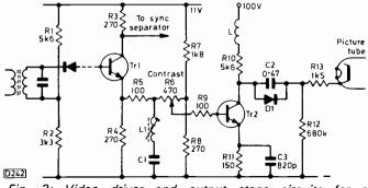
Fig. 2: Video driver and output stage circuits for a monochrome portable set.
