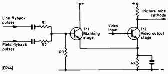
Fig. 4: One method of achieving flyback blanking.
